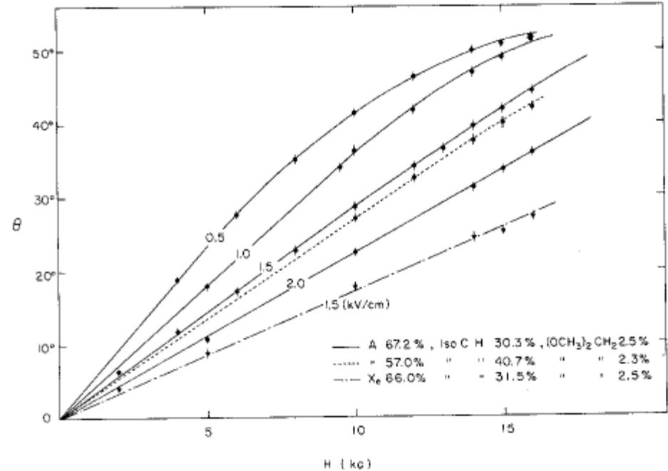
Fig. 38 Measured drift angle (angle between the electric field and the drift directions) as a function of electric and magnetic field strength<sup>9</sup>.
