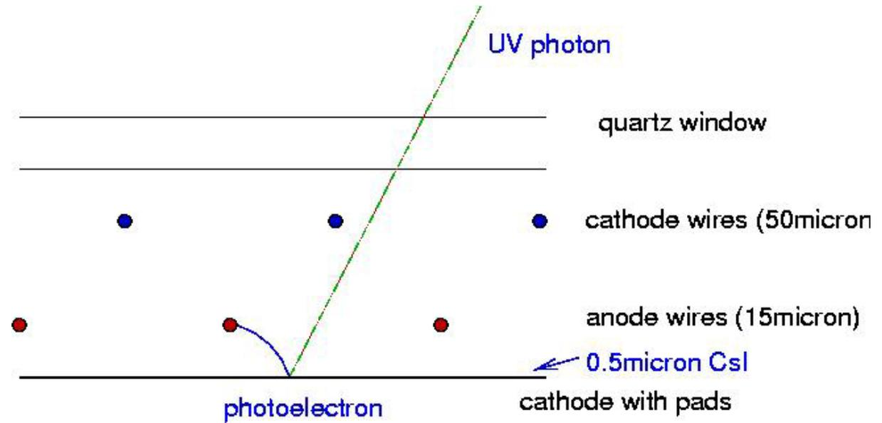
One of the cathodes of a multiwire chamber is segmented with pads (e.g. 8mmx8mm) and covered by a material which
