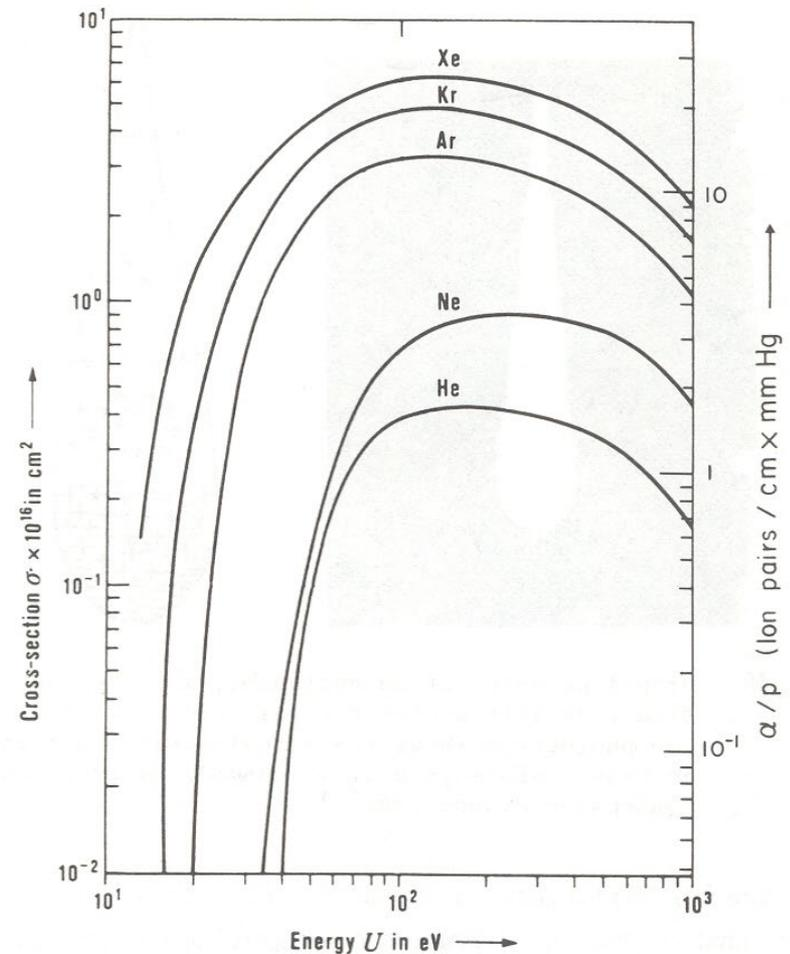
Fig. 45 Cross-section and first Townsend coefficient as a function of electron energy, for noble gases<sup>28)</sup>
