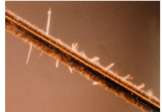
Cathodes: deposited layer is typically poorly conductive  $\rightarrow$  charge accumulation on both sides of the layer  $\rightarrow$  high electric fields  $\rightarrow$  high breakdown probability  $\rightarrow$  random high pulses
