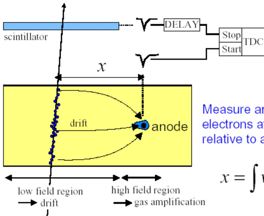
Measure arrival time of electrons at sense wire relative to a time  $t_0$ .
