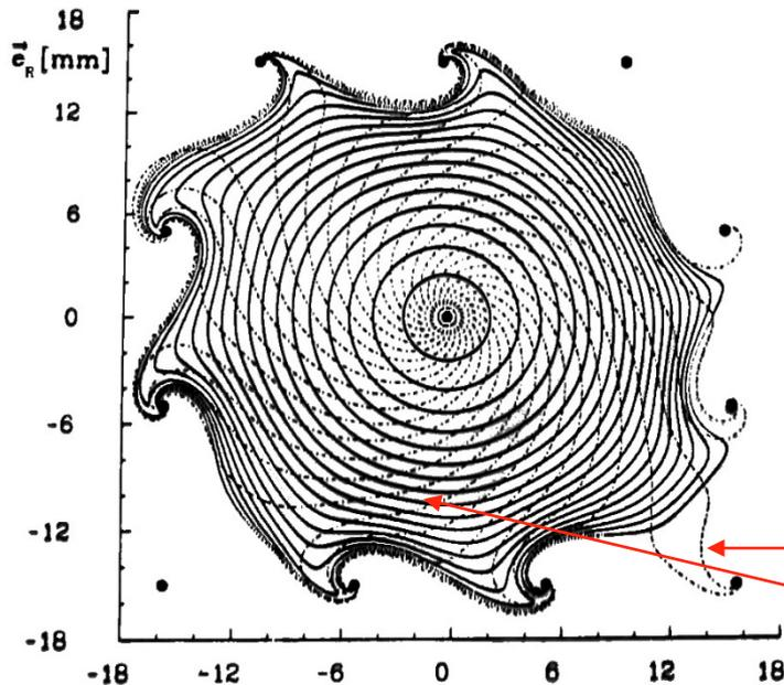
Drift lines in a radial E field (dash-dotted)
