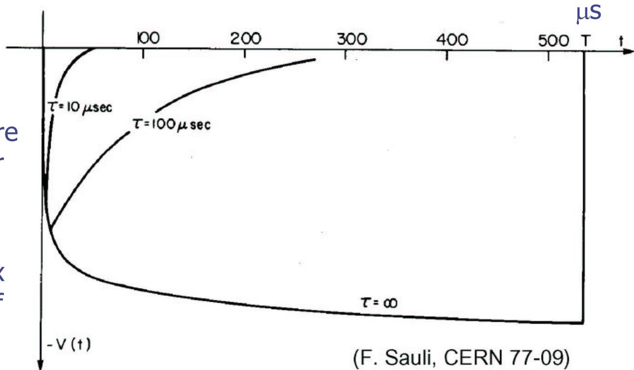
If faster signals are needed  $\rightarrow$  smaller time constants  $\rightarrow$  smaller signals
