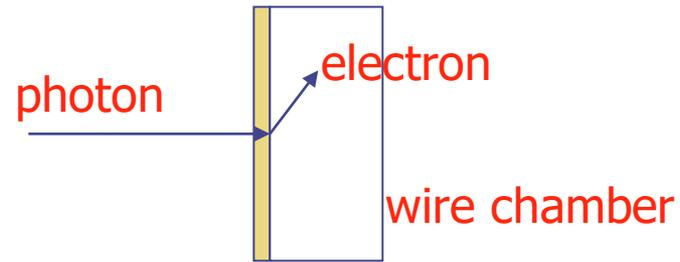
Need a high Z material (large photon absorption cross section) at the entrance of the wire chamber.
