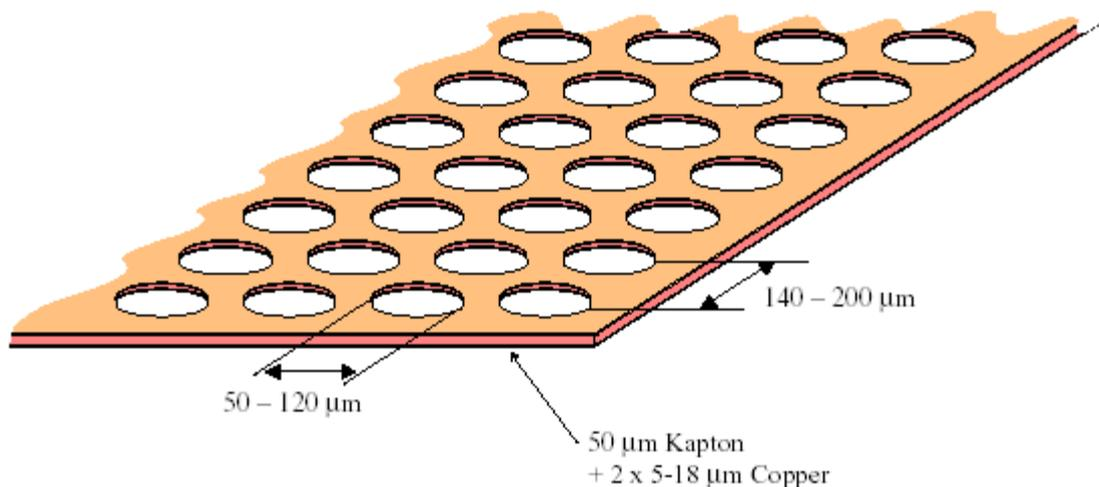
The E field in the holes is non-uniform – large enough to get gas amplification of about 100: useful as a preamplification stage for MSGCs.
