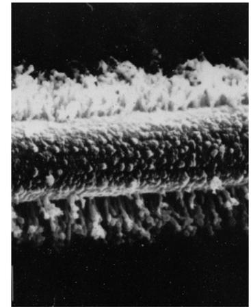
Anode wire ageing, consequence: gas amplification drops as a function of deposited charge (wire is thicker, and the amplification process is stopped earlier).
