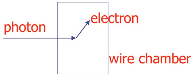
Need a high Z gas (large photon absorption cross section): the best is Xe, Ar is OK as well.
