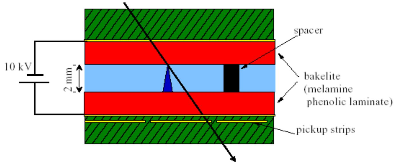
Gas amplification in a uniform electric field.
