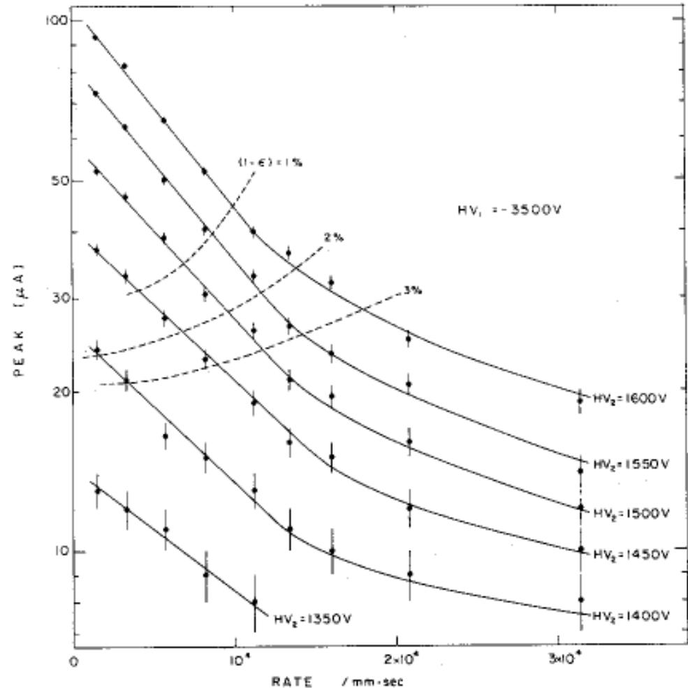
Fig. 54 Rate dependence of the peak current for minimum ionizing particles, in a drift chamber. The dashed curves show the equal inefficiency intercept, for a fixed detection threshold ( $5 \mu A$ )<sup>9</sup>.
