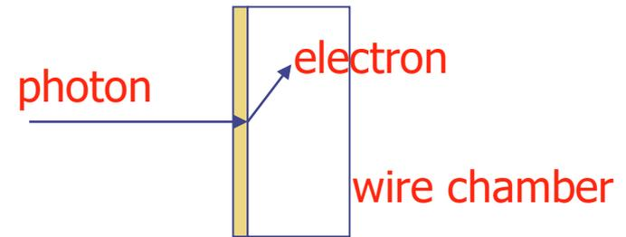
A multiwire proportional chamber can be used as a detector of electromagnetic radiation as well: if the photon hits an electron out of the material in the chamber (photo-effect), this electron can then be treated as a charged particle. In such a way a position sensitive detection of X,  $\gamma$  and UV rays becomes possible.
