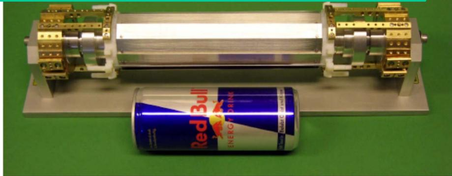
Prototype DEPFET pixel sensor and readout
