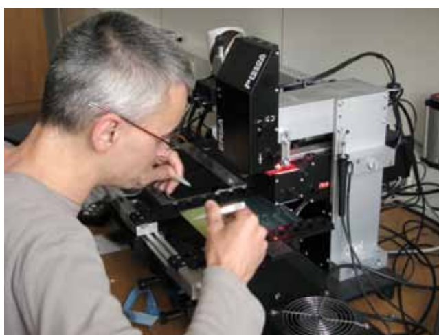
Figure 5: Assembly of the detector module using BGA (Ball Grid Array) technology
