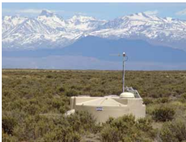
Figure 4: Čerenkov detectors placed in the so-called Ground array. More than 1600 such detectors measure high-energy particles through their interaction with water
