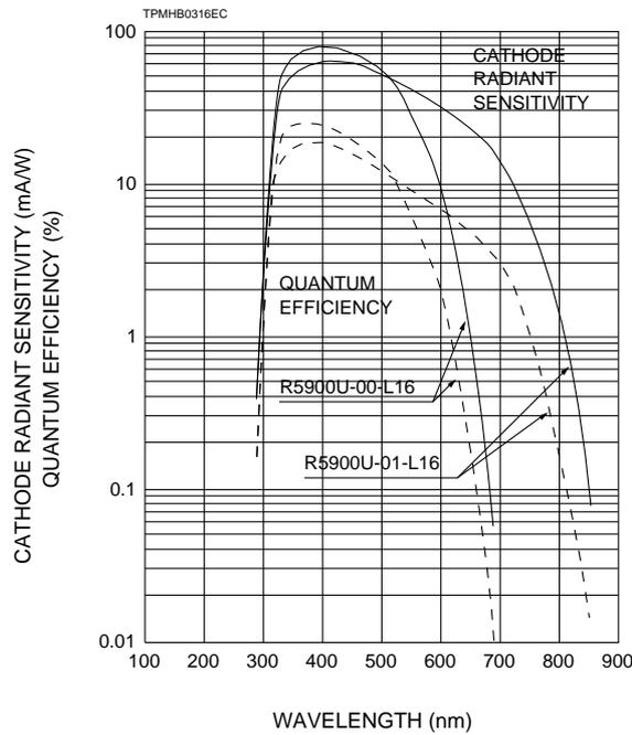
Figure 3: Typical spectral response of L16 PMT [8].
