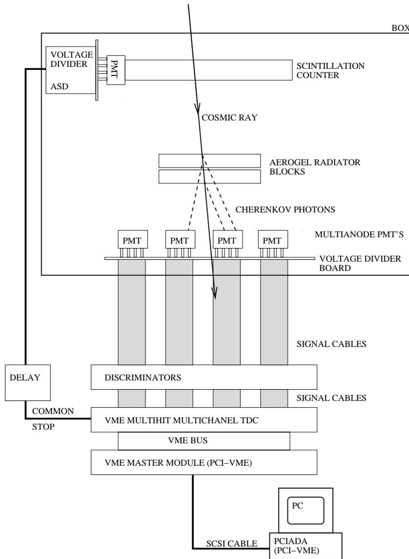
Figure 8: RICH counter for cosmic muons: the set-up.
