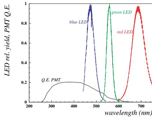
Figure 11: Spectra of three different LED sources.
