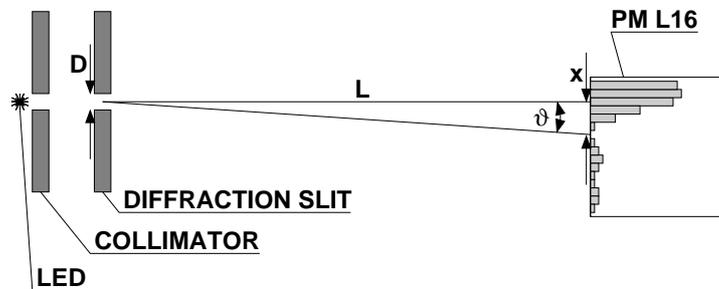
Figure 12: Geometric parameters for the diffraction measurement.
