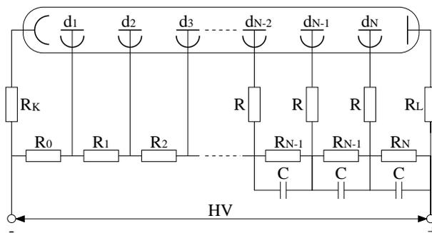
Figure 1: Voltage divider.
