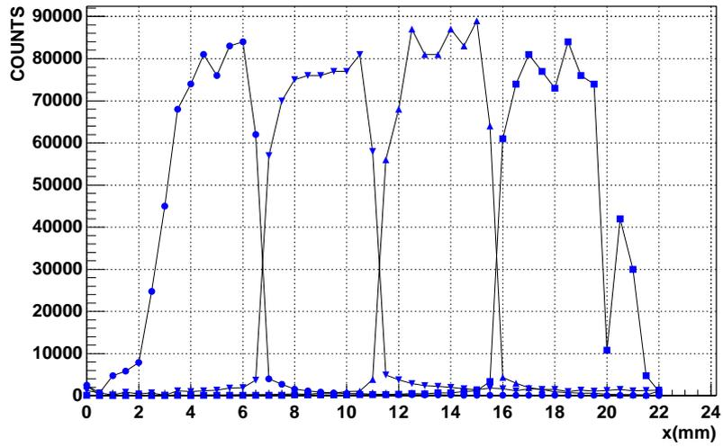
Figure 7: Count rate on 4 channels of the M16 PMT depending on the light spot position.
