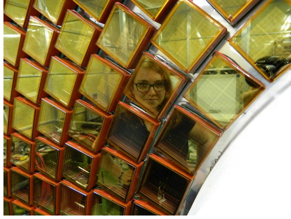
Figure 5.4: Array of Hybrid Avalanche Photo Diodes (HAPD), placed in one of the endcaps of Belle II and designed to detect photons from Cherenkov light being emitted by charged particles in an aerogel. Photo: R. Pestotnik.
