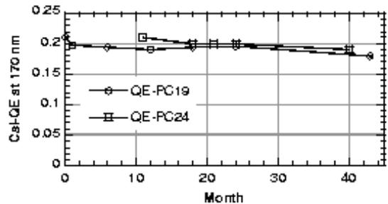
Fig. 10. Stability of CsI cathodes, stored in gas [28].
