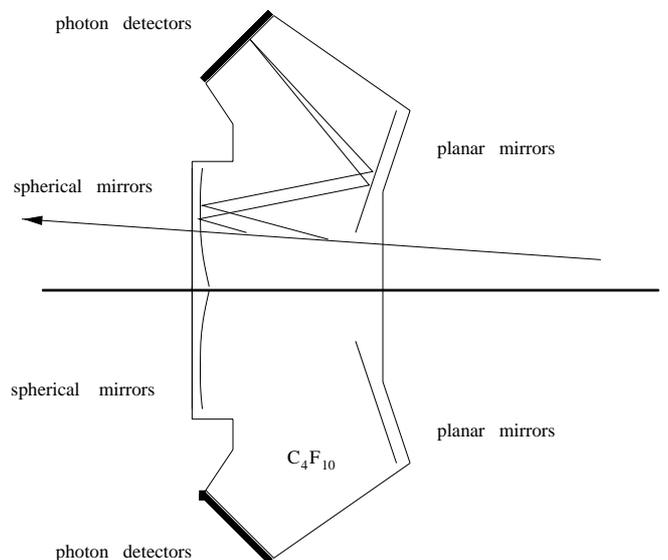
Fig. 2. Elements of a RICH counter. Shown is the HERA-B RICH layout, a typical fixed target example.
