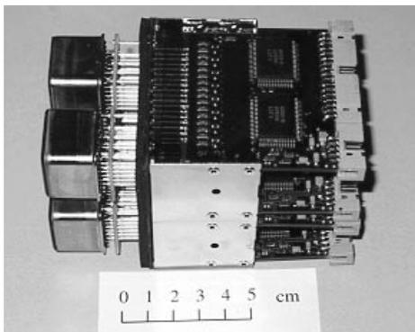
Fig. 5. Fully equipped basic module of the HERA-B RICH housing Hamamatsu R5900-M16 photomultiplier tubes.
