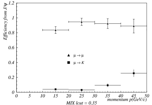
Fig. 22. Particle identification in the HERA-B RICH: efficiency to identify a muon, as deduced from the  $J/\psi \rightarrow \mu\mu$  decays.
