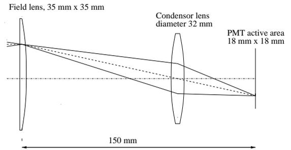
Fig. 13. Light collection in the HERA-B RICH: a system of two UVT acrylic lenses [33].
