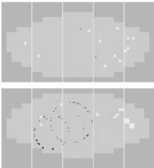
Fig. 4. A low multiplicity event recorded in the HERA-B RICH: on top of two clear rings on the lower photon detector half, only very few spurious hits can be observed. The diameter of the larger ring is about 60 cm.
