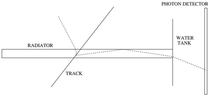
Fig. 18. Principle of the DIRC counter. Quartz is used as the radiator, and PMTs as photon detector.
