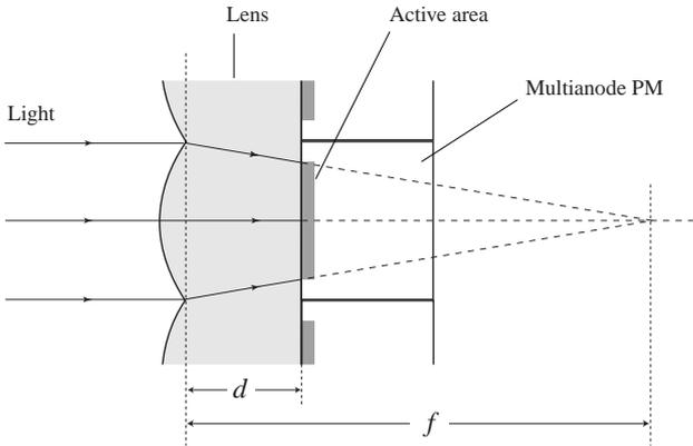
Fig. 15. Light concentrator for one of the LHCb photon detector options, a single quartz lens with a multianode PMT [31].
