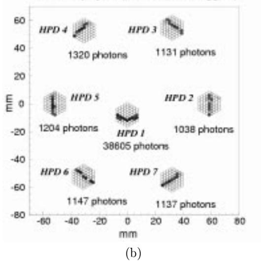
Fig. 12. HPD beam test with two radiators, gas and aerogel [31]: (a) set-up and (b) hit distribution on the photon detectors.
