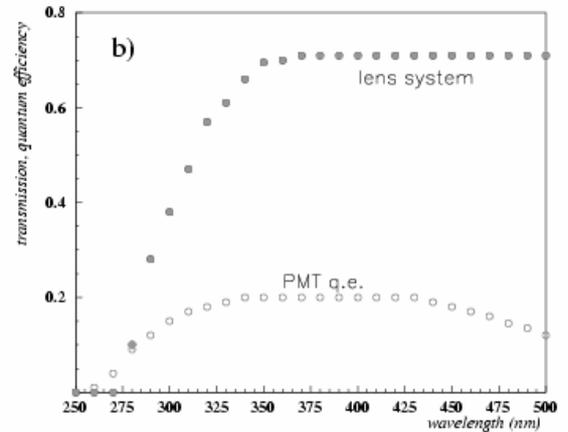
Fig. 14. HERA-B lens system: angular acceptance for three different wavelengths (a), transmission as a function of wavelength compared to the quantum efficiency of the PMT (b) [33].
