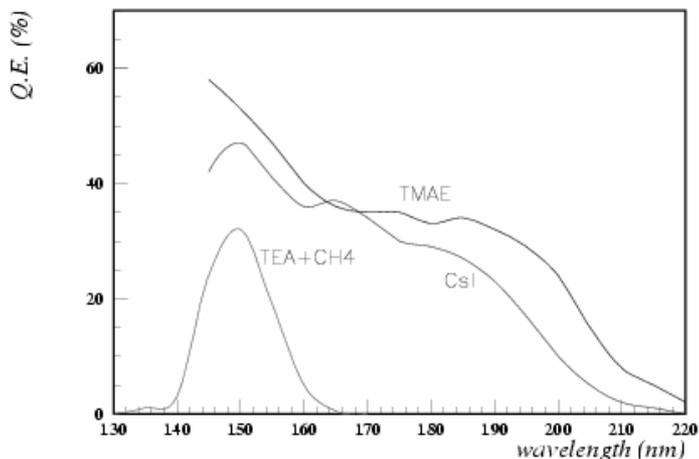
Fig. 6. Quantum efficiency of photosensitive substances which are most commonly used with wire chambers.
