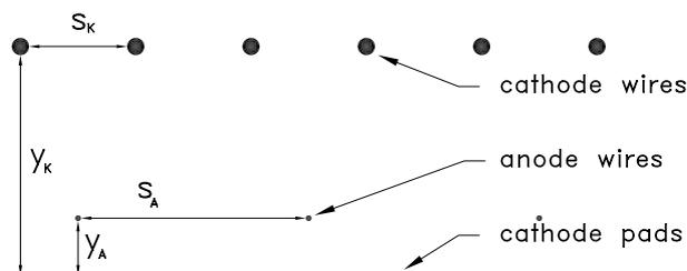
Fig. 7. An asymmetrical thin multiwire chamber with pad read-out and a photosensitive additive (either TEA in the chamber gas, or CsI evaporated on the pad cathode). The dimensions are:  $s_K = 1$  mm,  $y_K = 2$  mm,  $s_A = 2$  mm,  $y_A = 0.6 - 1$  mm. Instead of cathode wires, stripes evaporated on the chamber window material can be employed.
