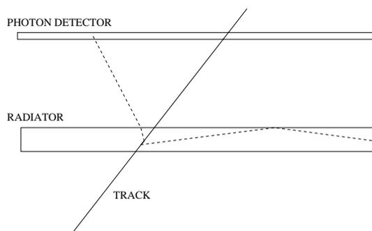
Fig. 8. Proximity focusing RICH: the Čerenkov photons are emitted in a thin (typically 1 cm thick) solid or liquid radiator medium, and are detected after they have traversed a gap of typically 10-20 cm.
