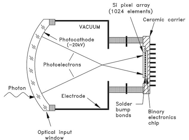
Fig. 11. Hybrid photon detector (HPD) of the LHCb experiment [31]. The outer diameter of the detector is 17 cm.
