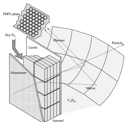
Fig. 17. The HERMES RICH counter with aerogel and gaseous radiators [39].
