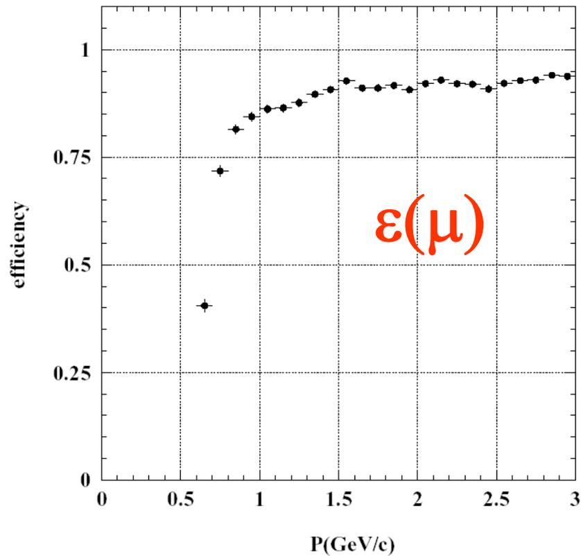
Fig. 109. Muon detection efficiency vs. momentum in KLM.
