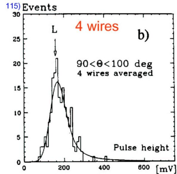
Measure in each of the 50 drift chamber layers – use truncated mean (discard 30% largest values – from the tail).
