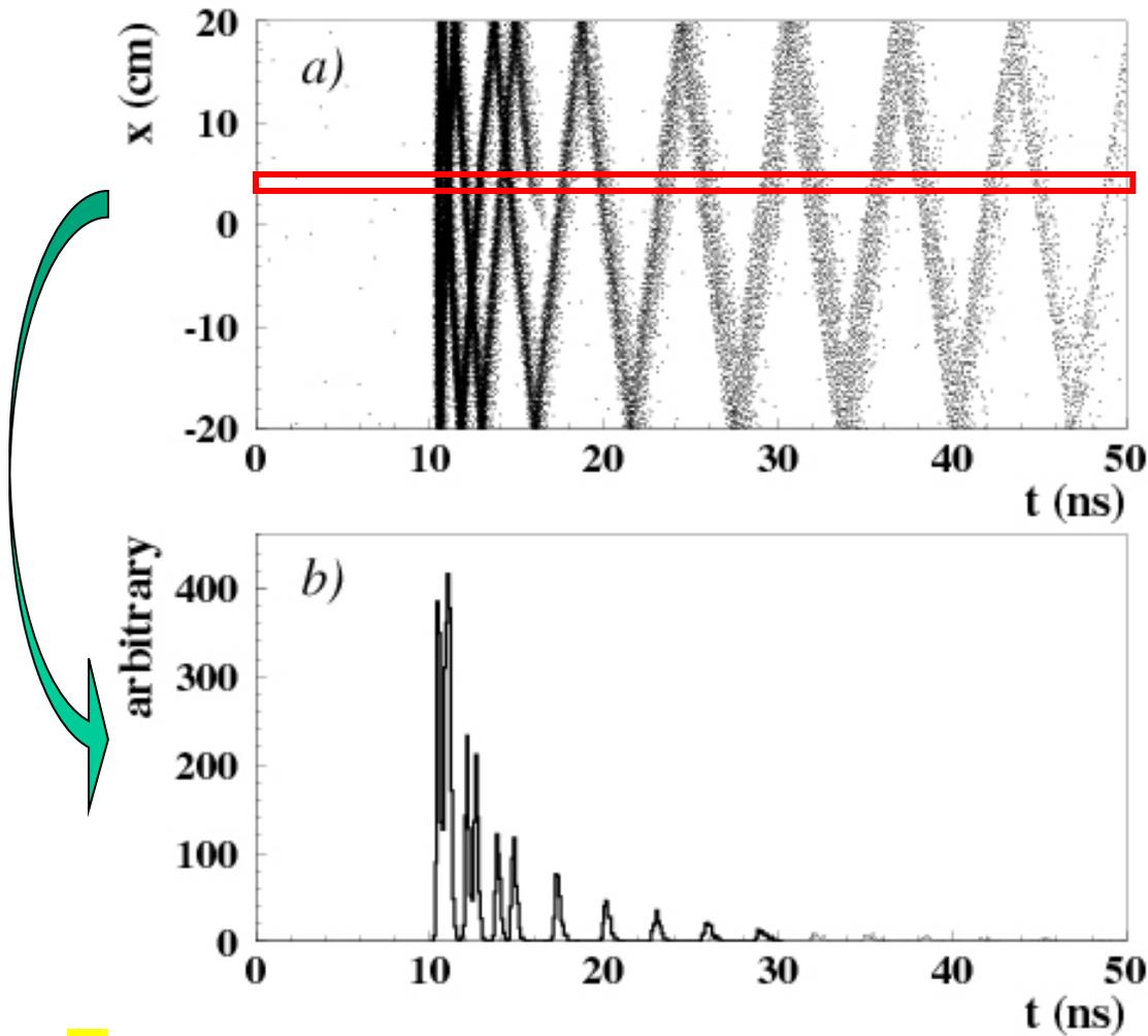
Pattern in the coordinate-time space ('ring') of a **pion** hitting a quartz bar with  $\sim 80$  MAPMT channels
