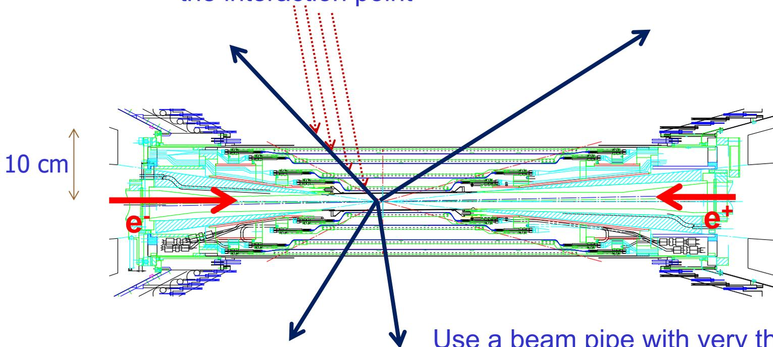
Use a beam pipe with very thin walls
