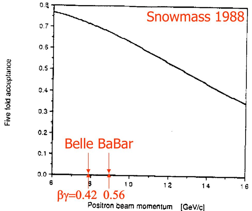
**Figure 4.** The acceptance of a detector covering  $|\cos \theta_{lab}| < 0.95$  for five uncorrelated particles as a function of the energy of the more energetic beam in an asymmetric collider at the  $\Upsilon(4S)$ .
