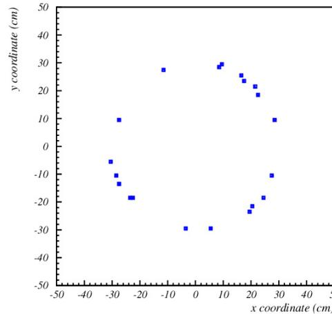
Idea: transform the **direction** into a **coordinate** → ring on the detection plane → **Ring Imaging Cherenkov (RICH) counter**
