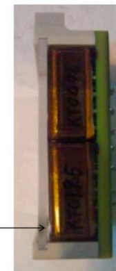
The bottom two PMTs rotated and came off the filter.
