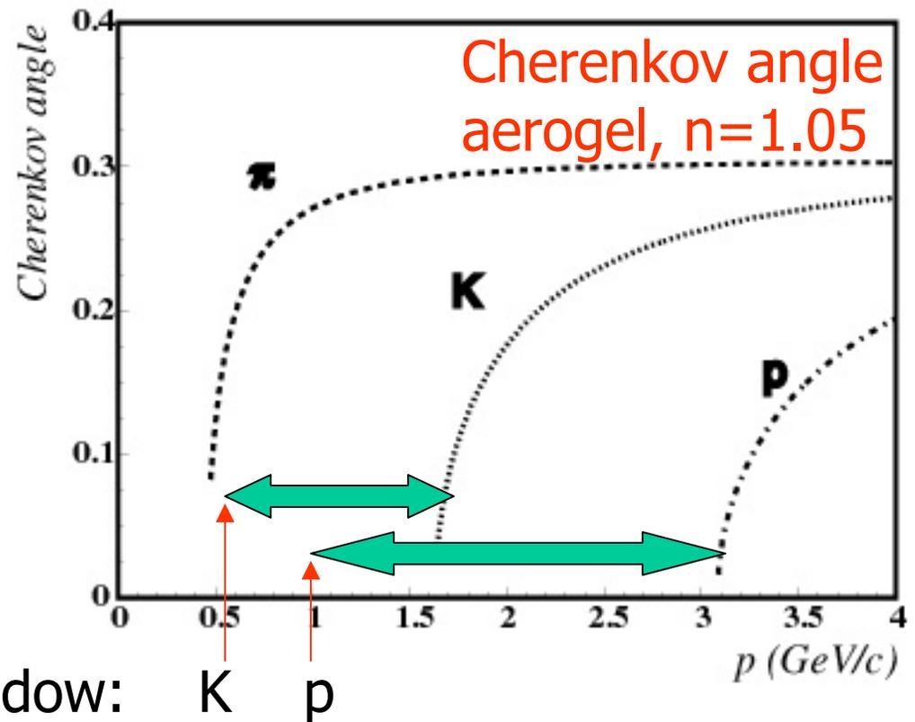
**Window:** threshold for kaons (protons) is at  $\sim 0.5$  GeV ( $\sim 0.9$  GeV):  $\rightarrow$  **positive identification** possible.
