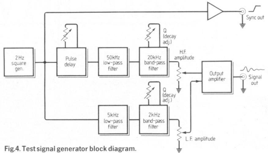
Fig.4. Test signal generator block diagram.
