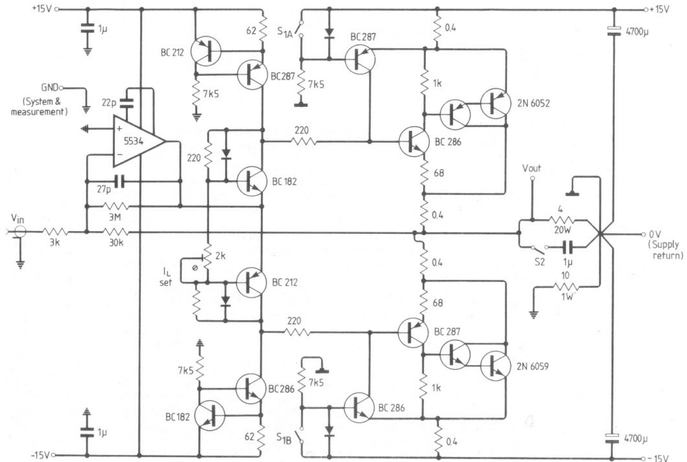
bandwidth and gain<sup>7</sup>. Also, the output impedance, being not near-zero under distortion conditions, forms an attenuator, together with the load which becomes part of the feedback loop. This is confirmed by Fig. 6 which shows error increase under capacitive load.
