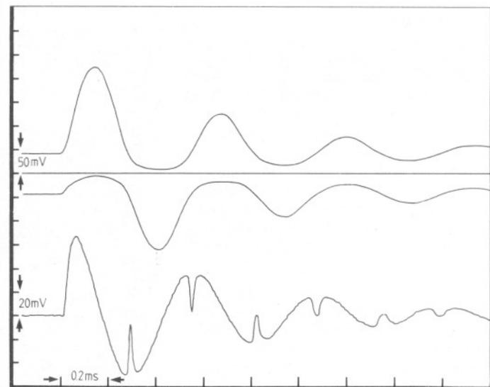
Fig.8. Class B output transistor currents (recorded as voltages across the emitter resistors) with zero current level shown for comparison. Vertical sensitivity 50mV/div.,  $R(e) = 0.4\text{ohm}$ ,  $R(L) = 4.0\text{ohm}$ ,  $I(q) = 100\text{mA}$ . Bottom trace shows the error signal at 20mV/div. Time base: 2ms full scale.
