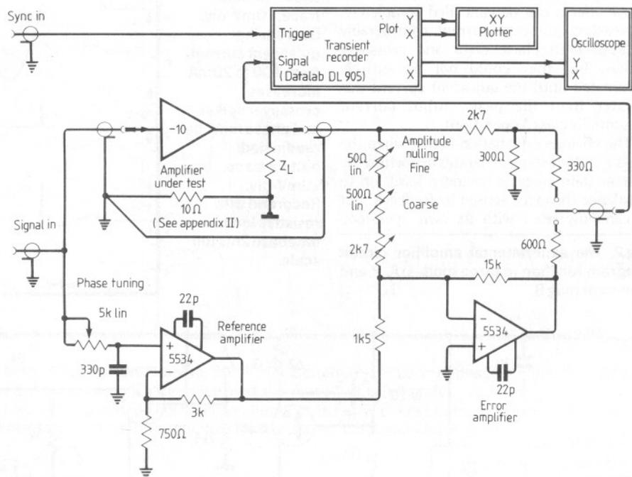
Fig.1. The "subtraction" test set-up due to Baxandall can be used with both steady-state and transient signals and does not require a precision reference.
