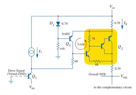
One half of the Non-Switching Class-B circuit.
