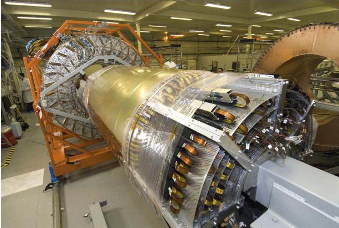
Fig.15: Mounting of the ATLAS Silicon Tracker (SCT) into the Transition Radiation Tracker (TRT). Note the large number of low-mass tapes providing power and control signals, one pair of tapes for each detector module.
