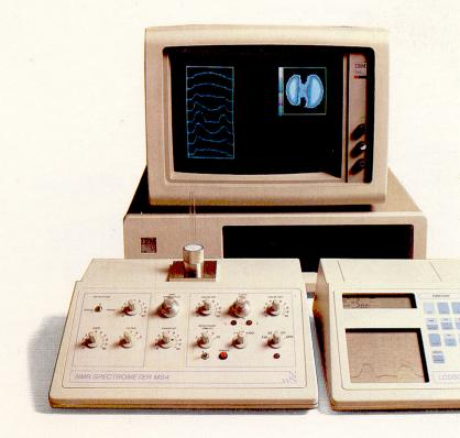
After Fourier transforms of the phantom free induction decay (measured at 32 different orientations of the phantom with respect to the static magnetic field gradient), the x-z cross section of the phantom sample is calculated in the IBM PC computer using the standard back-projection reconstruction technique. The resulting MR image is shown on the picture above and on the next page.
