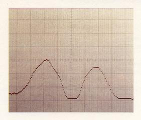
**A typical NMR signal** such as the Hahn echo of water protons displayed on the LCD screen is shown on the right. The free induction decay appearing first is brought about by the first 90° r.f. pulse. The 180° pulse which reverses the coherence loss and thus enables the formation of Hahn echo, is shown as three dots half way between the free induction decay and the echo.
