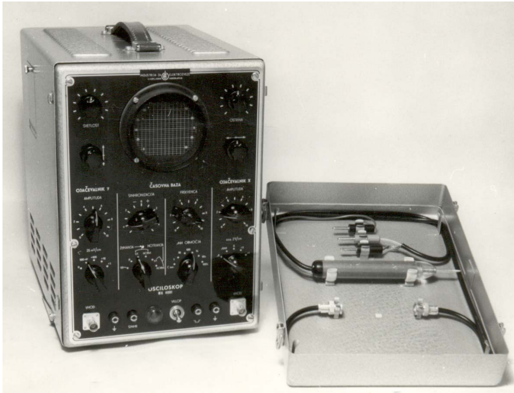
Fig. 1: This instrument, labeled MA4001, was designed in 1957, and it was the first oscilloscope with a triggered time base which went into regular serial production at Iskra. Maximal vertical sensitivity was 1 cm/100 mV, bandwidth 10 Hz to 800 kHz; the cathode ray tube was a 7 cm flat screen Telefunken DG 7-52A.
