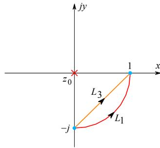
**Fig. 1.8.6:** The integral along the straight path  $L_3$  is the same as the integral along the circular path  $L_1$
