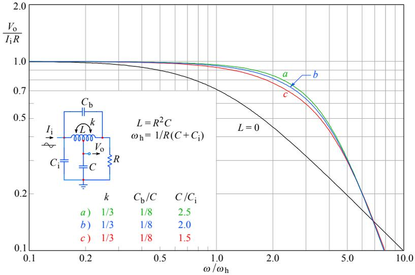
Fig. 2.5.8: Low coupling factor, Group 1: frequency response.
