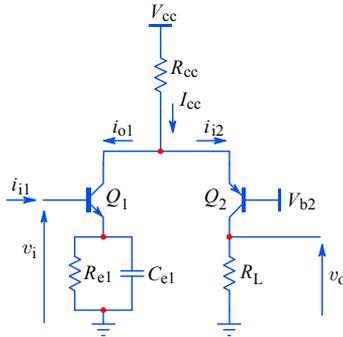
**Fig. 3.6.11:** The ‘folded’ cascode is formed by a complementary, NPN and PNP, transistor pair, connected in the otherwise usual cascode configuration. Since thermionic devices are not produced in complementary pairs, this circuit can not be realized with electronic tubes.
