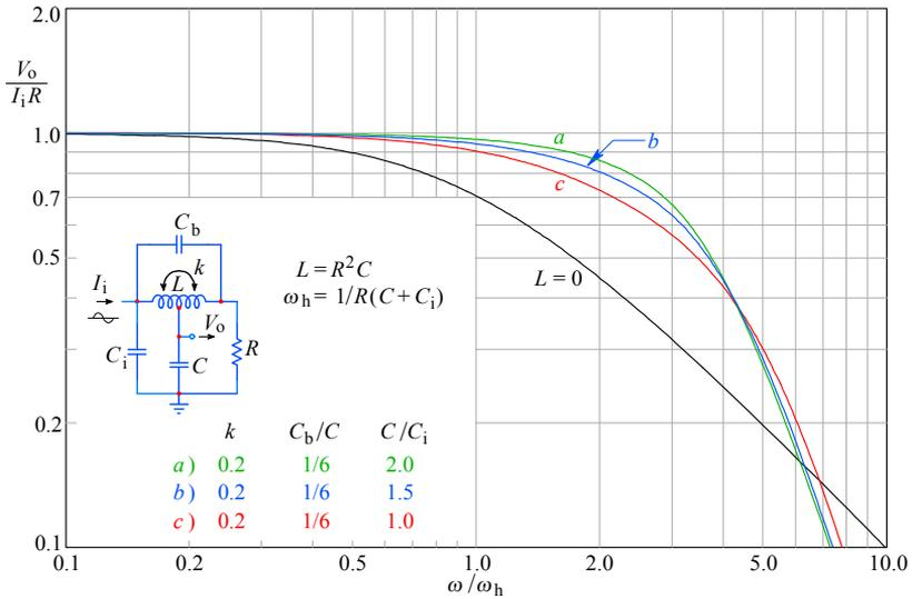
Fig. 2.5.10: Low coupling factor, Group 2: frequency response.
