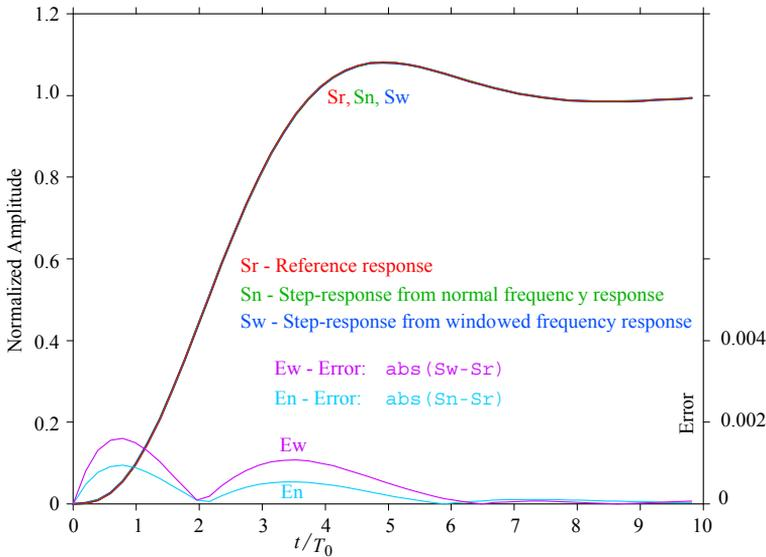
**Fig. 6.5.9 and 6.5.10:** As in Fig. 6.5.5–8, but with 50 samples of a 3<sup>rd</sup>-order Butterworth system. Windowing does not help any longer and produces even greater error. The dominant error is now owed to the Gibbs' effect.
