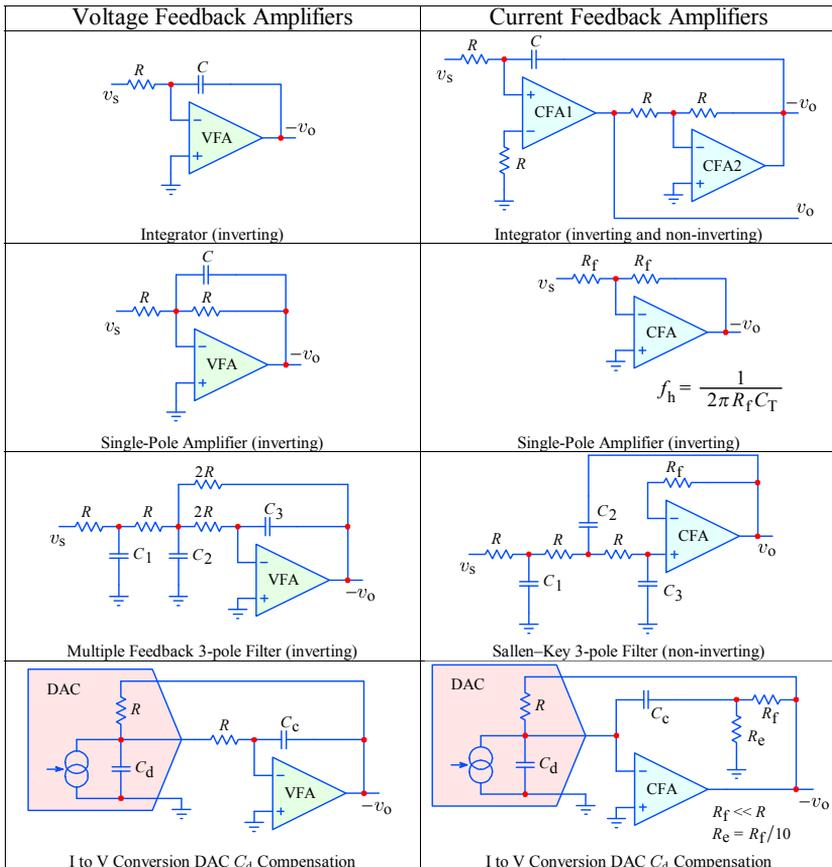
**Fig. 5.3.19:** Functionally equivalent circuits with conventional and current feedback amplifiers. Integrators, filters and current to voltage converters in inverting configurations cannot be achieved using a single CF amplifier. However, two-amplifier circuits can provide inherent amplifier pole compensation, which is very important at high frequencies. Filters can be realized in the non-inverting configuration. And feedback capacitance can be isolated by a resistive divider.
