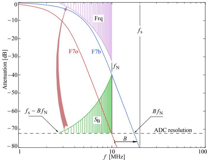
**Fig. 7.2.10:** If we invert the alias spectrum  $S_B$  the envelope of the resulting spectrum  $F_{rq}$  represents the minimum attenuation requirement that a digital filter should have in order to suppress the aliased spectrum below the ADC resolution.
