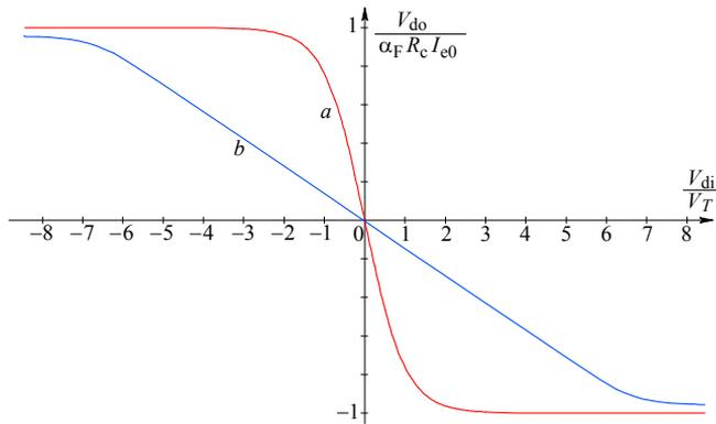
**Fig. 5.4.9:** **a)** The DC transfer function of the differential amplifier in [Fig. 5.4.8a](#); the input differential voltage is normalized to  $V_T$  and the output is normalized to  $\alpha_F R_c I_{e0}$ . **b)** With the emitter degeneration, as in [Fig. 5.4.8b](#), the transfer function is more linear, but at the expense of the gain (lower slope).
