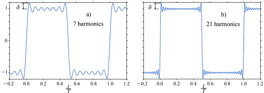
**Fig. 1.2.7:** The Gibbs' phenomenon; **a)** A signal composed of the first seven harmonics of a square wave spectrum from Table 1.2.1. The overshoot is  $\delta \simeq 18\%$  of the nominal amplitude; **b)** Even if we take three times more harmonics the overshoot  $\delta$  is nearly equal in both cases.
