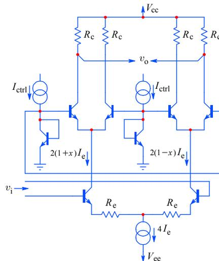
**Fig. 5.4.44:** Two quadrant multiplication is sufficient for the oscilloscope continuously variable gain control; however, the same differential symmetry of the four quadrant multiplier has been retained for the M377 because of good thermal balance and DC stability.
