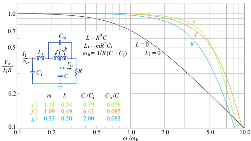
**Fig. 2.6.4:** Some additional frequency response plots of the four-pole L+T peaking circuit: *e)* Chebyshev with 0.05° phase ripple, *f)* Gaussian to -12dB, *g)* double 2<sup>nd</sup>-order Bessel. Note the lower bandwidth of *g)* ( $2.9\omega_h$ ) compared with *b)* in Fig. 2.6.3 ( $3.47\omega_h$ ). This clearly shows that the bandwidth of a cascade of identical stages is lower than if the stages have staggered poles.
