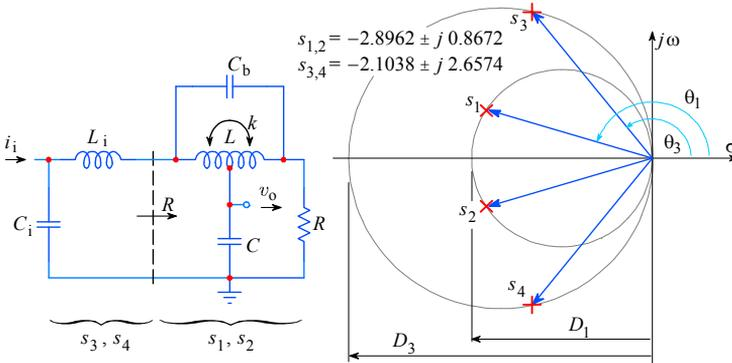
Fig. 2.6.1: The four-pole L+T network.
