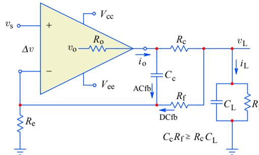
**Fig. 5.3.29:** The capacitive load is separated from the AC feedback path by a small resistor  $R_c$  in series with the output; owing to the capacitance  $C_c$  this type of compensation can be applied only to voltage feedback unity gain compensated amplifiers.
