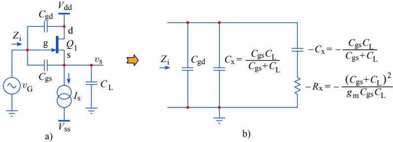
**Fig. 3.9.2:** The JFET source follower biased by a current generator and loaded only by the inevitable stray capacitance  $C_L$ : a) circuit schematic; b) the input impedance has two **negative** components, owed to  $C_{gs}$  and  $g_m$  (see [Sec. 3.9.5](#)).
