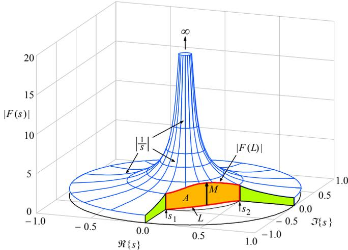
**Fig. 1.13.1:** The complex function magnitude,  $|F(s)| = |1/s|$ . The resulting surface has been cut between  $-j$  and  $+1$  to expose an arbitrarily chosen integration path  $L$ , starting at  $s_1 = 0 - j0.5$  and ending at  $s_2 = 0.5 + j0$ . On the path of integration the function  $|F(s)|$  has a maximum value  $M$ .
