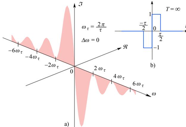
**Fig. 1.3.3:** a) The frequency spectrum of a single square wave is expressed by complex conjugate phasors. Since the phasors are infinitely many, they merge in a continuous planar form. Also the spectrum extends to  $\omega = \pm \infty$ . The corresponding waveform is shown in b). Note that all the even frequency components  $2\pi n/\tau$  are missing ( $n$  is an integer).
