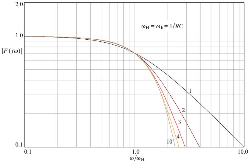
**Fig. 4.4.10:** Frequency response magnitude of systems with normalized Bessel poles of order  $n = 1, 2, 3, 4,$  and  $10$ . Note the nearly identical passband response—this is the reason why we can approximate the oscilloscope (multi-stage) amplifier rise time from the cut off frequency, using the relation for the first-order system:  $\tau_r = 0.35/f_T$ .
