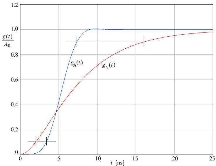
**Fig. 5.1.7:** The gain normalized step responses of the 7-pole compensated system  $g_A(t)$  and the 2-pole non-compensated system  $g_N(t)$ . The rise time is 14 ns for the  $g_N(t)$ , but only 3.8 ns for  $g_A(t)$ . The overshoot of  $g_A(t)$  is only 0.48 %.
