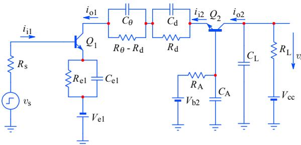
**Fig. 3.4.12:** The compensated cascode amplifier. If  $R_A C_A$  compensation is used,  $R_d C_d$  may become unnecessary. The main bandwidth limiting time-constants are now  $(R_s + r_{b1})C_{e1}$  and  $(C_{\mu2} + C_L)R_L$ .
