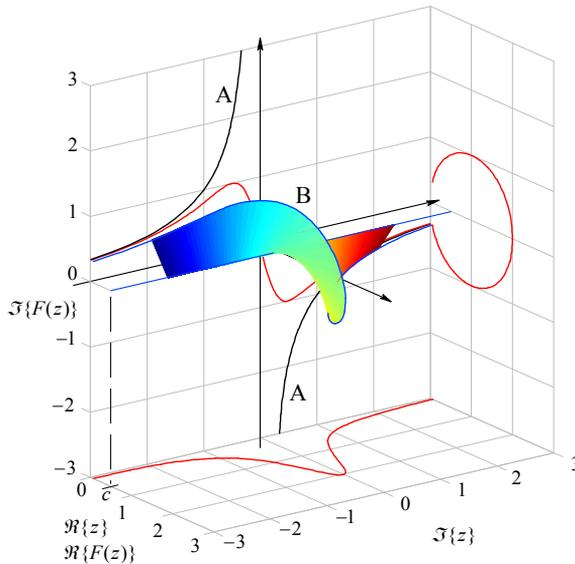
**Fig. 1.8.2:** By reducing the complex domain  $x + jy$  to  $c + jy$ , where  $c$  is a constant, we can plot the complex function  $F(c + jy)$  in a 3D graph. Here we have  $c = 0$  (graph A) and  $c = 0.5$  (graph B). Also shown are the three projections of B. The twisted surface is the integral of  $F(c + jy)$  for  $c = 0.5$  and  $y$  in the range  $-j2 < y < j2$ . See [Appendix 1](#) (web only) for details.
