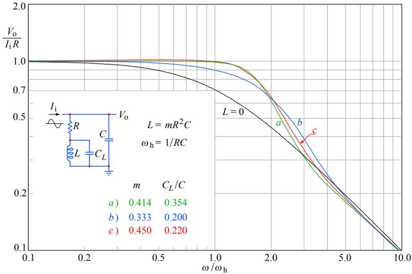
**Fig. 2.8.2:** Three-pole shunt peaking circuit frequency response: **a)** MFA; **b)** MFED; **c)** SPEC. The non-peaking case ( $L = 0$ ) is the reference. The difference of the number of poles and the number of zeros is only 1 for peaking systems, therefore the ending slope of the frequency response is similar to that of the non-peaking system.
