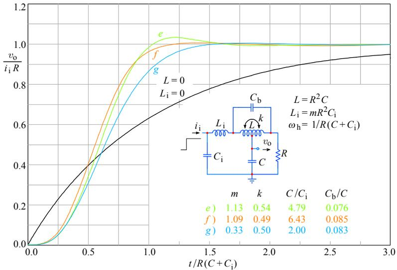
**Fig. 2.6.8:** Some additional four-pole L+T circuit step responses: *e)* Chebyshev 0.05°; *f)* Gaussian to -12dB; *g)* double 2<sup>nd</sup>-order Bessel. Again, the step response confirms that repeating the poles is not optimal; compare the rise times of *g)* and *b)* in Fig. 2.6.7.
