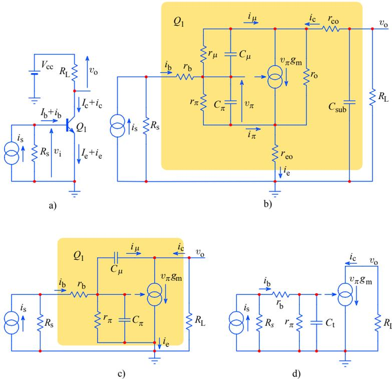
**Fig. 3.1.1:** The common emitter amplifier: a) circuit schematic diagram – the current and voltage vectors are drawn for the NPN type of transistor; b) high frequency small signal equivalent circuit; the components included in the  $Q_1$  model are explained in the text; c) simplified equivalent circuit; d) an oversimplified circuit where  $C_t = C_\pi + AC_\mu = \text{constant}$ .
