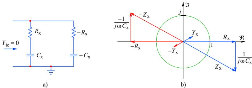
**Fig. 3.9.11:** a) The negative components of the input impedance can be compensated by an equal but positive network, connected in parallel, so that their admittances sum to zero (infinite impedance). In b) we see the corresponding phasor diagram.
