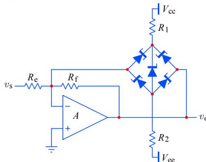
**Fig. 5.3.31:** The output level clipping is more precise if a biased Zener diode in a Schottky diode bridge is controlling the feedback. However, this circuit can be used only with voltage feedback unity gain compensated amplifiers.
