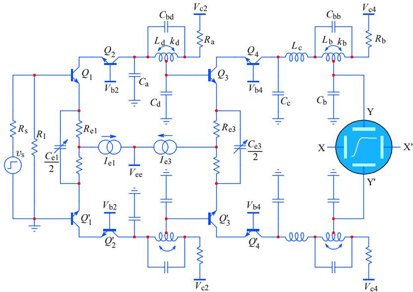
**Fig. 5.1.1:** A simple 2-stage differential cascode amplifier with a 7-pole peaking system: the 3-pole T-coil inter-stage peaking (between the  $Q_2$  collector and the  $Q_3$  base) and the 4-pole L+T-coil output peaking (between the  $Q_4$  collector and the vertical plates of the cathode ray tube). The schematic was simplified to emphasize the important design aspects — see text.
