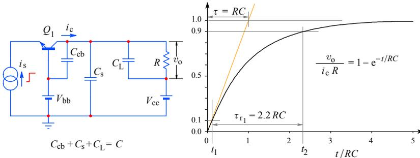
**Fig. 2.1.1:** A common base amplifier with  $RC$  load: the basic circuit and its step response.
