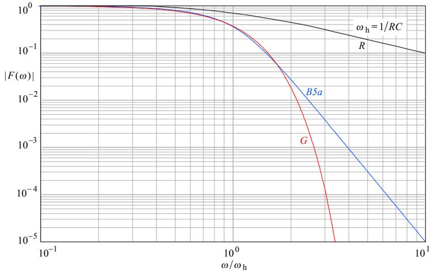
**Fig. 4.4.8:** Frequency response in log-log scale brings into evidence how the ideal Gaussian response  $G$  decreases much more steeply with frequency than the 5<sup>th</sup>-order Bessel response  $B5a$ . The Bessel system would have to be of infinitely high order to match the Gaussian response.
