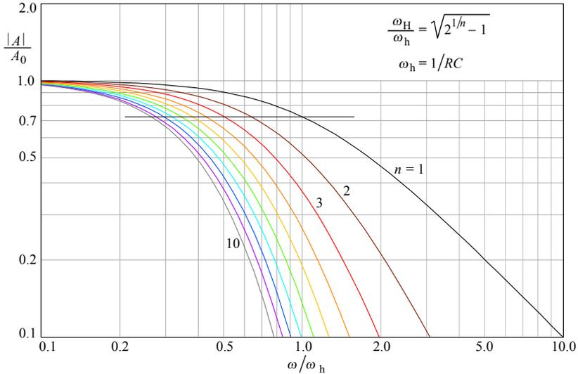
**Fig. 4.1.2:** Frequency response of an  $n$ -stage amplifier ( $n = 1, 2, \dots, 10$ ). To compare the bandwidth, the gain was normalized, i.e., divided by the system DC gain,  $(g_m R)^n$ . For each  $n$ , the bandwidth (the crossing of the 0.707 level) shrinks by  $\sqrt{2^{1/n} - 1}$ .
