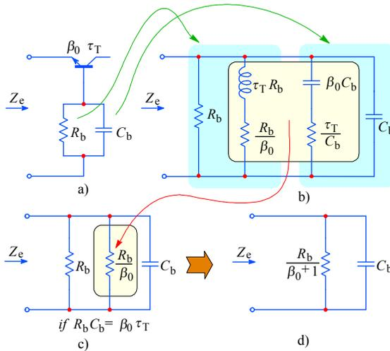
**Fig. 3.2.7:** Base to emitter  $RC$  network transformation: a) schematic; b) equivalent circuit; c) if  $R_b C_b = \beta_0 \tau_T$  the middle components form a resistance; d) final equivalent circuit.
