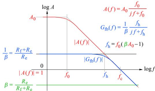
**Fig. 5.4.2:** For a voltage feedback amplifier the closed loop frequency response  $G_{fb}(f)$  depends on the open loop gain  $A_0$ , its dominant pole  $f_0$  and the feedback attenuation factor  $\beta$ . The transition frequency  $f_c$  is equal to the amplifier gain bandwidth product (but only if the amplifier does not have a secondary pole close to or lower than  $f_c$ ).
