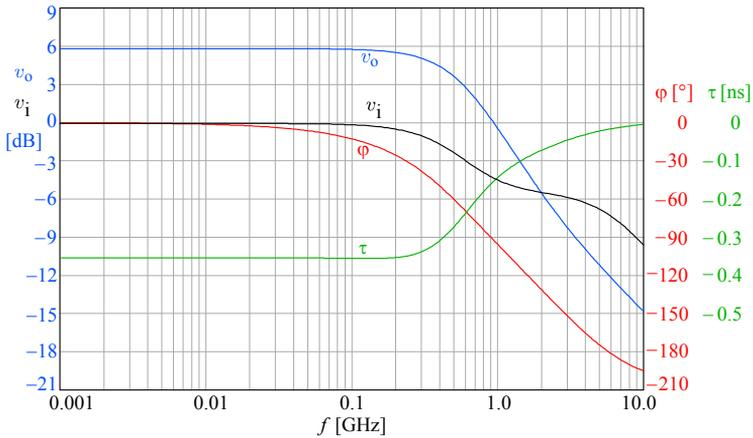
**Fig. 5.4.19:** Frequency domain performance of the circuit from Fig. 5.4.18. The bandwidth can be high (560 MHz), but for a suitable error sensing the required high value of  $R_1$  would compromise it. The plot of  $v_i$  indicates the negative input impedance at high frequencies, which would need additional compensation networks at both inputs and at  $R_1$ .
