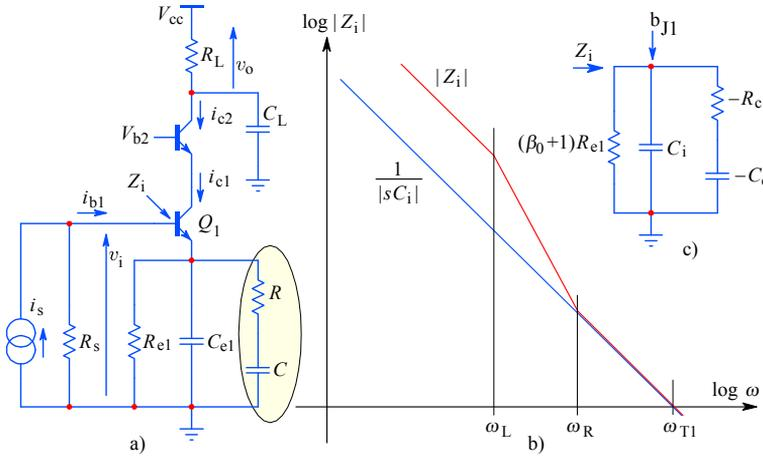
**Fig. 3.5.1:** Emitter peaking in cascode amplifiers. a) By adding a zero at  $\omega_R = 1/RC$  to the emitter network of  $Q_1$ , we modify the input impedance  $Z_i$  at the base junction of  $Q_1$ ; b) the frequency dependent asymptote plot of  $Z_i$ ; c) the equivalent schematic has negative components, too. See the explanation in [Sec. 3.5.2](#).
