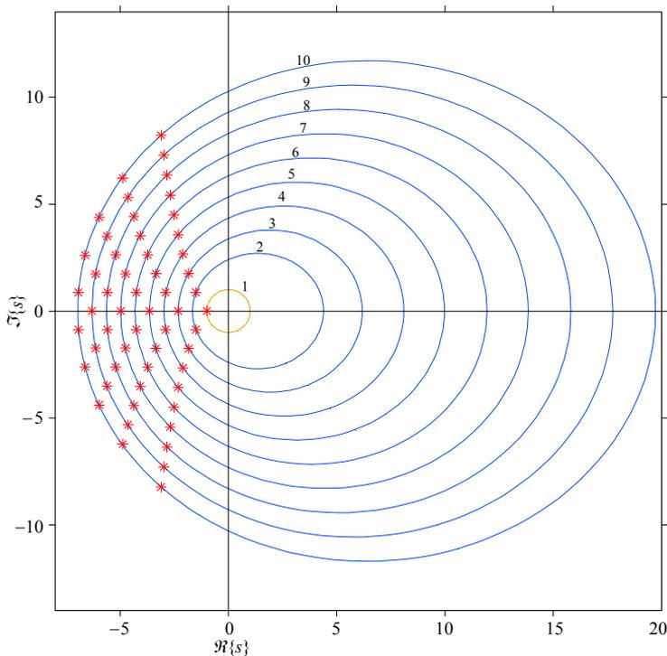
**Fig. 4.4.1:** Bessel poles for order  $n = 1-10$ . Bessel poles lie on a family of ellipses with one focus at the origin of the complex plane and the other focus on the positive real axis. The first-order pole is the same as for the Butterworth system and lies on the unit circle.
