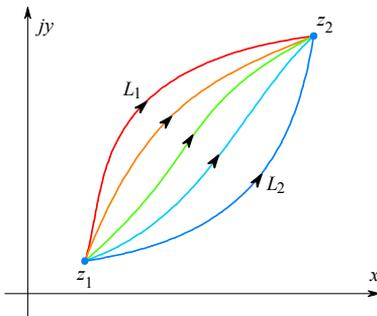
**Fig. 1.8.3:** A line integral from  $z_1$  to  $z_2$  along the line  $L_1$ ,  $L_2$ , or any other line lying between these two yields the same result because between  $L_1$  and  $L_2$  the function has no pole.
