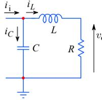
**Fig. 2.2.1:** A two-pole series peaking circuit.
