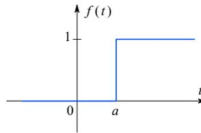
Fig. 1.5.2: Unit step function starting at  $t = a$ .
