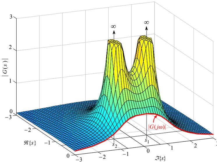
**Fig. 1.14.2:** The magnitude of the system transfer function, Eq. 1.14.8, for  $s_{1,2} = (-1 \pm j)/\sqrt{2}$  and  $K = 1$ . For  $\Re(s) = 0$ , the surface  $|G(s)|$  is reduced to the frequency response's magnitude curve,  $|G(j\omega)|$ . The height at  $s_{1,2}$  is  $\infty$ , but was limited to 3 in order to see  $|G(j\omega)|$  in detail.
