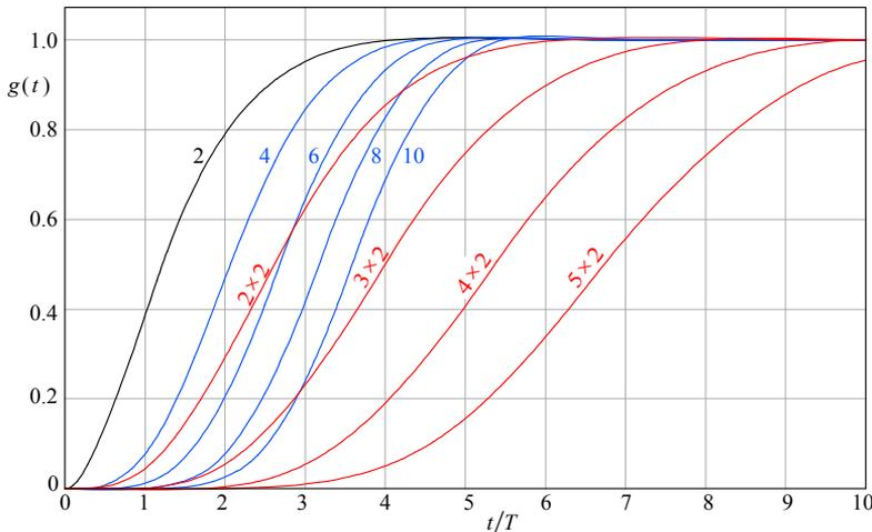
**Fig. 4.6.2:** Step response of systems with staggered poles, compared with systems with repeated second-order pole pairs. The rise times of systems with repeated poles increase with each additional stage, whilst for systems with staggered poles they even decrease slightly!
