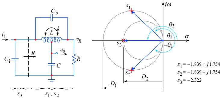
Fig. 2.5.1: The three-pole T-coil network.
