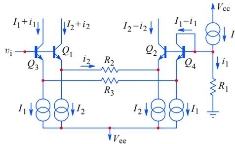
**Fig. 5.4.17:** A simple differential amplifier with feedforward error correction. Accurate matching of transistors is required only for DC error reduction, not for the feedforward linearization. Here  $i_2$  is the differential current, whilst the error current,  $i_1$ , sensed at  $R_1$ , is available at the  $Q_3$  collector to be added to the output current further in the circuit.
