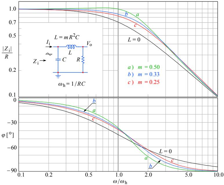
**Fig. 2.2.9:** Input impedance modulus (normalized) and the associated phase angle of the series peaking circuit for the characteristic values of  $m$ . Note that for high frequencies the input impedance approaches that of the capacitance. *a)* MFA; *b)* MFED; *c)* CD.
