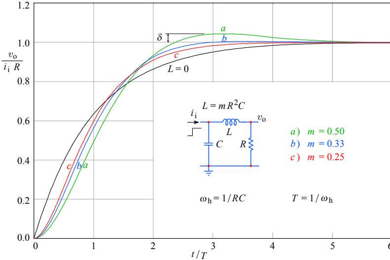
**Fig. 2.2.8:** Step response of the series peaking circuit for the four characteristic values of  $m$ : a) MFA; b) MFED; c) CD. The case  $m = 0$  ( $L = 0$ ) is the reference. The MFA overshoot is  $\delta = 4.3\%$ , whilst for MFED it is only  $\delta = 0.43\%$ .
