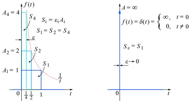
**Fig. 1.6.1:** The Dirac function as the limiting case of narrowing the pulse width, while keeping the time integral constant: **a)** If the pulse length is decreased, its amplitude must increase accordingly. **b)** When the pulse length  $\varepsilon \rightarrow 0$  the amplitude is  $(1/\varepsilon) \rightarrow \infty$ .
