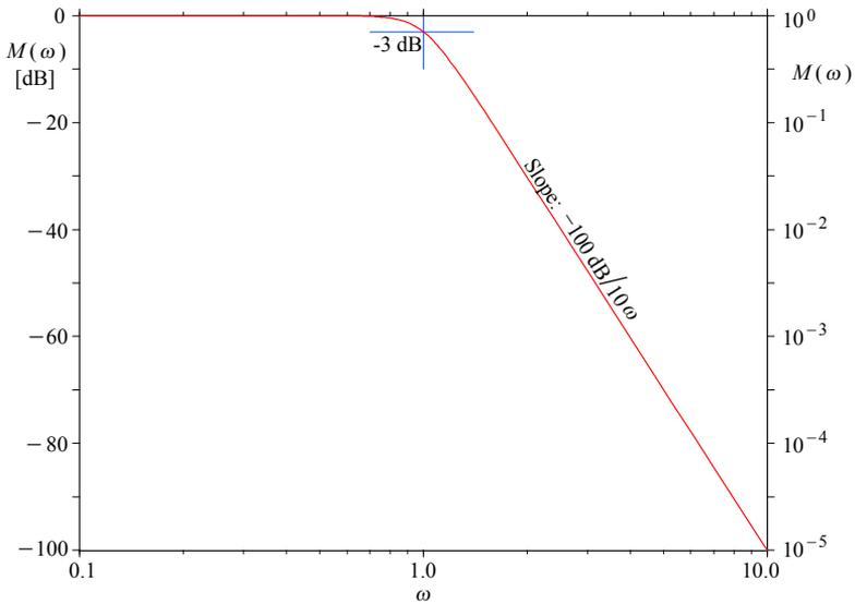
**Fig. 6.4.5:** Bode plot of the 5<sup>th</sup>-order Butterworth system magnitude, as in Fig. 6.4.4, but in a linear dB vs. log frequency scale. In such a scale, all-pole systems have an asymptotically linear attenuation slope, proportional to the system order (a factor of  $10^n$  or  $n \times 20$  dB/10 $\omega$ ). The marked  $-3$  dB reference point is the same half power cut off frequency point as in Fig. 6.4.4.
