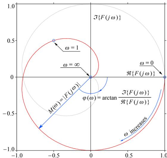
**Fig. 6.4.3:** The Nyquist plot of the 5<sup>th</sup>-order Butterworth system frequency response. The frequency axis is reduced to a single point projection at the origin and is parametrically incremented with the phase angle, from the DC point on the real axis, to the half power bandwidth point at  $[-0.5, 0.5*j]$  and to infinity at the origin.
