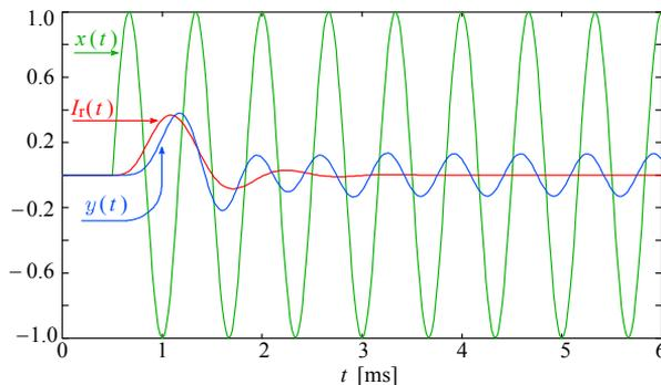
**Fig. 7.1.1:** Convolution example: response  $y(t)$  to a sine wave  $x(t)$  switched-on into a 5<sup>th</sup>-order Butterworth system, whose impulse-response is  $I_r(t)$ , shown here as the ideal response (instead of unity gain); both are delayed by the same switch-on time (0.5 ms). The system responds by phase shifting and amplitude modulating the first few wave periods, reaching finally the forced ('steady state') response.
