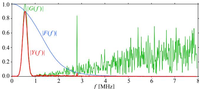
**Fig. 7.1.5:** The spectrum  $G(f)$  of the signal in Fig. 7.1.4a is multiplied by the system's frequency response  $F(f)$  to produce the output spectrum  $Y(f)$ . Along with the modulated signal centered at 560 kHz, there is a strong 2.8 MHz interference from another source and a high level of white noise (rising with frequency), both being substantially reduced by the filter.
