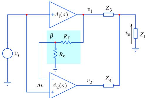
**Fig. 5.4.4:** Grounded load feedforward amplifier. Note the inverted input polarity of the auxiliary amplifier, compared with the circuit in [Fig. 5.4.1b](#). This allows passive signal summing over the output impedances  $Z_3$  and  $Z_4$ .
