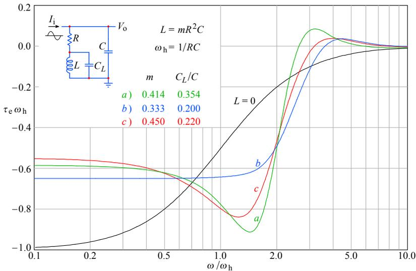
**Fig. 2.8.4:** Three-pole shunt peaking circuit envelope delay: *a)* MFA; *b)* MFED; *c)* SPEC. The non-peaking ( $L = 0$ ) case is shown as the reference. Note the envelope advance in the high frequency range, owed to system zeros.
