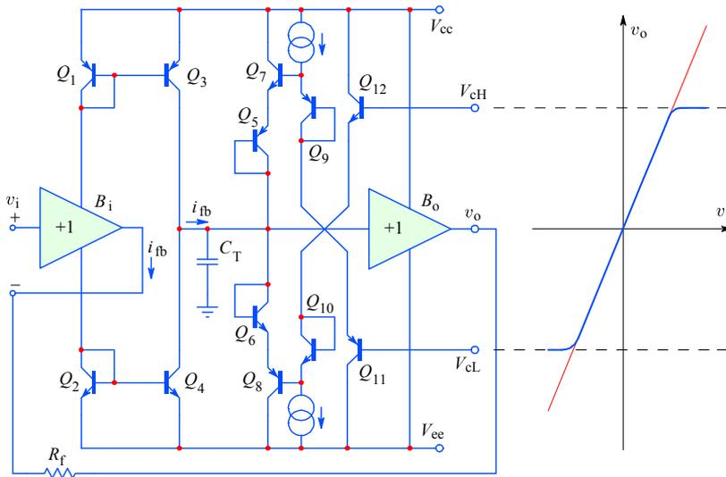
**Fig. 5.3.33:** Output signal clipping by limiting the internal  $C_T$  node of a current feedback amplifier. The transistors  $Q_{5-8}$  are normally reverse biased. For positive voltages  $Q_{6,8}$  ( $Q_{5,7}$  for negative) start conducting only when the voltage at  $C_T$  reaches  $V_{cH}$  ( $V_{cL}$ ).
