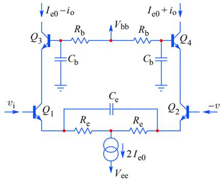
Fig. 5.4.11: This simple differential cascode amplifier, employing no error correction, is used in the test set up circuit of Fig. 5.4.10, representing the reference against which all other amplifiers are compared. The emitter peaking and base impedance are adjusted for a MFED response.
