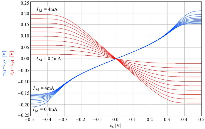
**Fig. 5.4.40:** DC transfer function of the Gilbert multiplier of Fig. 5.4.39, for  $2I_{c1} = 4\text{ mA}$  and modulation current  $2I_{c2} = I_M = 0.4\text{--}4\text{ mA}$ . The signal source ( $v_s$ ) range is  $\pm 0.5\text{ V}$ .
