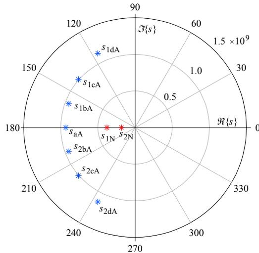
**Fig. 5.1.5:** The polar plot of the 7-pole compensated system (poles with index 'A') and the 2-pole non-compensated system (index 'N'). The radial scale is  $\times 10^9$  rad/s. The angle is in degrees.
