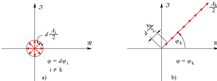
**Fig. 1.2.4:** a) The integral over the full period  $T$  of a rotating phasor is zero; b) the integral over a full period  $T$  of a non-rotating phasor  $d A_k/2$ , gives its amplitude,  $A_k/2$ , (the symbol  $d$  stands for  $dt/T$  — in this figures  $dt \rightarrow \Delta t$  such that  $\Delta t \omega_k = \pi/4$ ). Note that a stationary phasor retains its initial angle  $\varphi_k$ .
