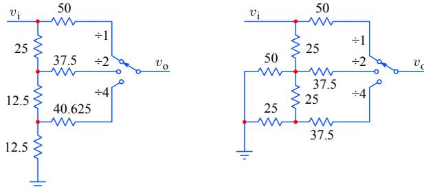
**Fig. 5.2.24:** The low impedance attenuator ( $50\ \Omega$  input and output) can be built as a straight  $\tau$ -type ladder or a  $\pi$ -type ladder. If driven by a current source the series  $50\ \Omega$  in the  $\div 1$  branch can be omitted.
