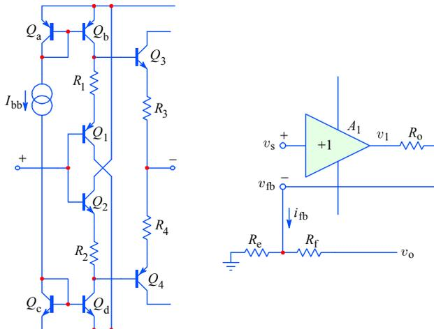
**Fig. 5.3.11:** The resistors  $R_{1-4}$  used to balance the inputs are the cause for the non-zero inverting input resistance,  $R_3 \parallel R_4$ , modeled by  $R_e$ ; this causes an additional voltage drop, reducing the feedback current (see analysis).
