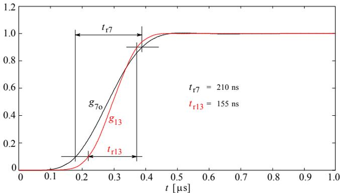
**Fig. 7.2.13:** Step response comparison of the original 7-pole analog only filter  $g_{7o}$  and the improved 13-pole mixed mode (7-pole analog + 6-pole digital) Bessel–Thomson filter,  $g_{13}$ . Note the shorter rise time and longer time delay of  $g_{13}$ . The resulting rise time is also better than that of the 9-pole analog only filter (see [Fig. 7.2.8](#)).
