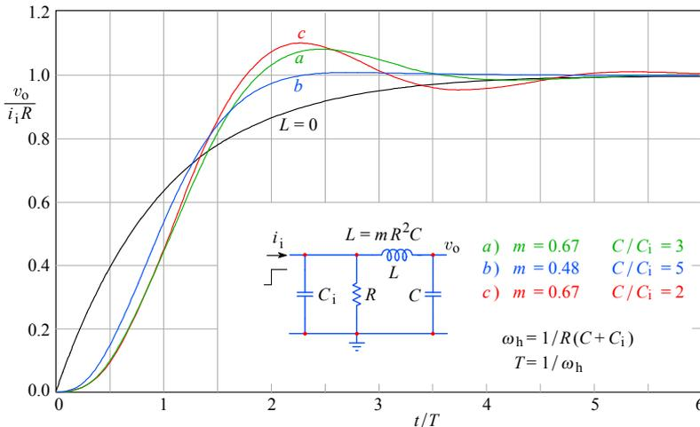
**Fig. 2.3.5:** Step response of the third-order series peaking circuit for some characteristic values of  $m$ : **a)** MFA; **b)** MFED; **c)** SPEC; the non-peaking ( $L = 0$ ) case is the reference. The overshoot of both MFA and SPEC case is too large to be suitable for pulse amplification.
