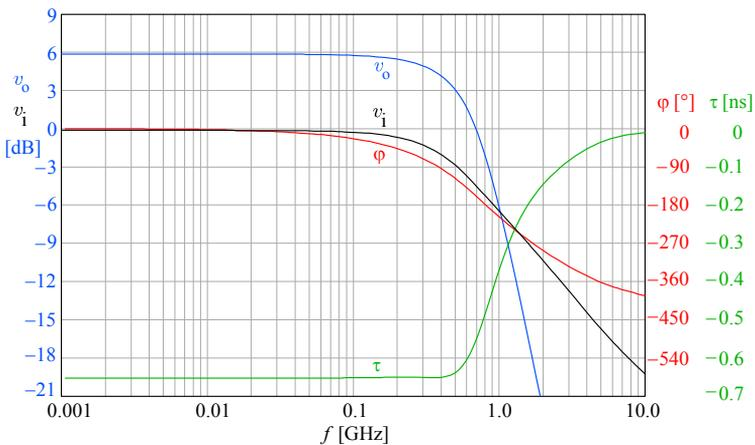
Fig. 5.4.22: Frequency domain performance of the 'Cascomp' amplifier. The bandwidth is about 500 MHz, but note also the high flatness of the envelope delay, right up to the bandwidth limit.
