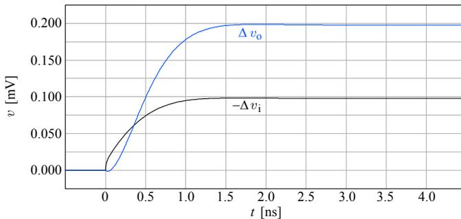
**Fig. 5.4.13:** Time domain performance of a simple differential cascode amplifier of Fig. 5.4.11 (no error correction) used in the test set up circuit of Fig. 5.4.10. This will be used as the reference for all other circuits. The input voltage indicates the input impedance dynamics in the first 100 ps and up to 1.5 ns. Note also the small undershoot at the output, owed to the cross-talk via  $C_{bc}$  of  $Q_{1,2}$ . The output rise time is less than 1 ns.
