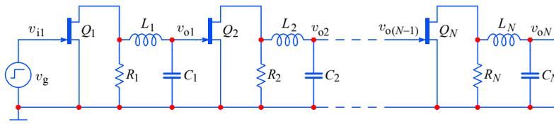
**Fig. 4.3.7:** An example of an amplifier with  $N$  shunt peaking stages. Since each stage has one pair of complex conjugate poles the number of stages is equal to one half of the number of poles,  $N = n/2$ . For odd-order systems one stage (usually the first one) is of a single pole configuration ( $L_1 = 0$ ), and  $N = 1 + (n - 1)/2$ . Of course, instead of the shunt peaking, other peaking networks can be used.
