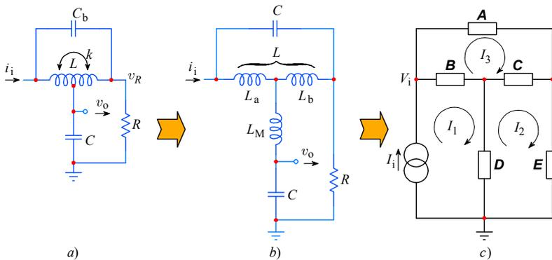
**Fig. 2.4.1:** **a)** The basic T-coil circuit: the voltage output is taken from the center tap node of the inductance  $L$  and its two parts are magnetically coupled by the factor  $0 < k < 1$ ; **b)** an equivalent circuit, with no magnetic coupling between the coils — it has been replaced by the mutual inductance  $L_M$ ; **c)** a simplified generalized impedance circuit, excited by the current generator  $I_i$ , showing the current loops.
