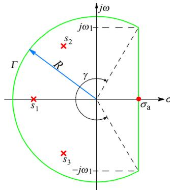
**Fig. 1.13.5:** The integral along the inverted ‘D’ shaped contour encircling the poles is equal to the sum of the residues of each pole. This contour is used to prove the inverse Laplace transform, where the integral along the arc vanishes if  $R \rightarrow \infty$ , provided that the number of poles exceeds the number of zeros by at least 2 (in this example no zeros are shown).
