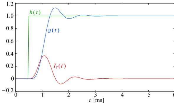
**Fig. 7.1.2:** Checking convolution: response  $y(t)$  of the 5<sup>th</sup>-order Butterworth system to the unit step  $h(t)$ . The system's impulse response  $I_t(t)$  is also shown, but with its ideal size (not unity gain). Apart from the 0.5 ms (25-samples) time delay and the time scale, the step response is identical to the one shown in [Part 6, Fig.6.5.1](#).
