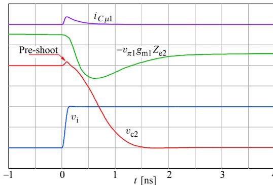
**Fig. 3.4.5:** The step response  $v_{e2}$  has a pre-shoot owed to the signal cross-talk through  $C_{\mu1}$  (arbitrary vertical units, but corresponding to  $A_v = -2$ ).
