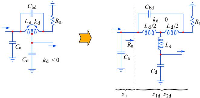
**Fig. 5.1.3:** With the assigned poles and the resulting particular component values the 3-pole stage magnetic coupling  $k_d$  needs to be negative, which forces us to use non-coupled coils and add a positive mutual inductance  $L_c$ . Even with a negative  $k_d$  the T-coil reflects its resistive load to the network input, greatly simplifying the calculations of component values.
