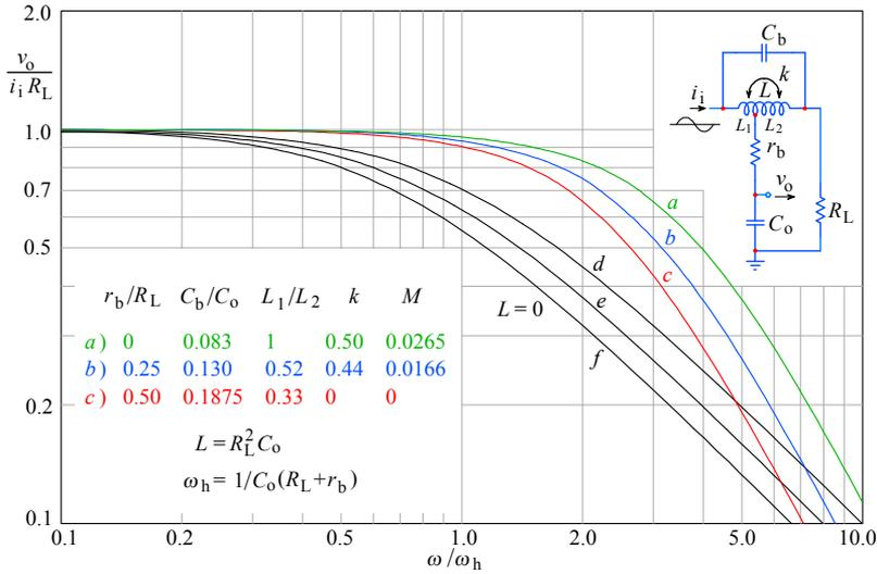
**Fig. 3.6.3:** MFED frequency response of the T-Coil transistor interstage coupling circuit for three different values of  $r_b$ : a)  $r_b = 0$ ; b)  $r_b = 0.25 R_L$ ; c)  $r_b = 0.5 R_L$ . For comparison the three reference cases ( $L = 0$ ): d), e), and f), which correspond to the same three  $r_b/R_L$  ratios, are drawn. The bandwidth improvement factor of the peaking system remains 2.72 times over the non-peaking reference for each value of  $r_b$ .
