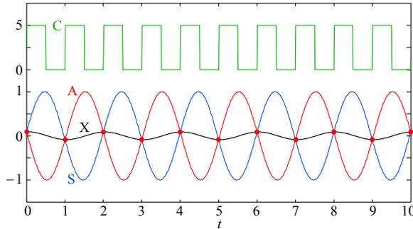
**Fig. 7.2.4:** When the signal frequency is equal to the Nyquist frequency, there are two samples per period and the correct alias signal is of the same amplitude as the original signal. However, the perceived alias amplitude is a function of the phase difference between the signal and the clock. A  $10^\circ$  phase shift results in a low apparent amplitude, as shown by the X waveform.
