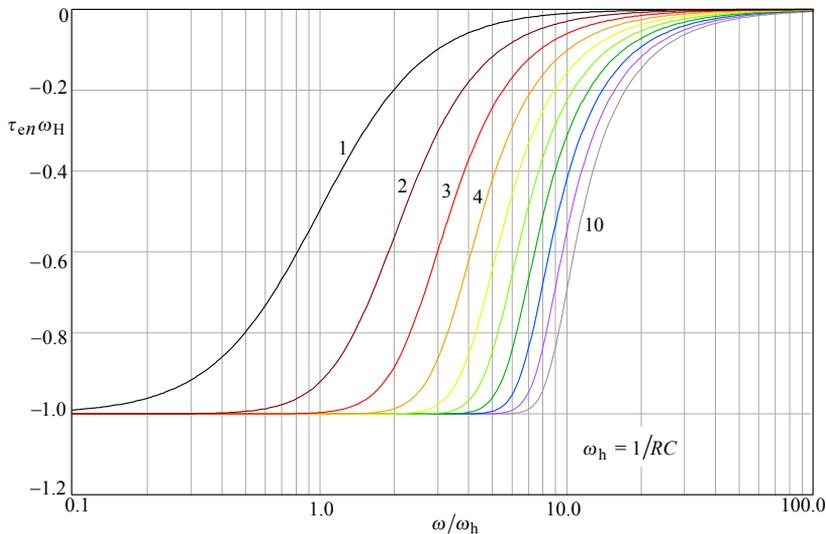
**Fig. 4.4.5:** Envelope delay of the systems with Bessel poles for order  $n = 1-10$ . Note the flat unit delay response increasing with system order. This figure demonstrates the fulfillment of the criterion from which we have started the derivation of MFED.
