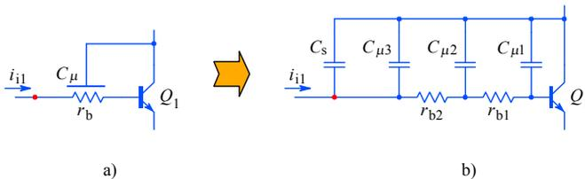
**Fig. 3.6.10:** a) The base–collector reverse capacitance  $C_\mu$  is actually spread across the base resistance  $r_b$ . b) A good approximation is achieved by splitting  $r_b$  in half and  $C_\mu$  in three parts, adding also the external stray capacitance  $C_s$ .
