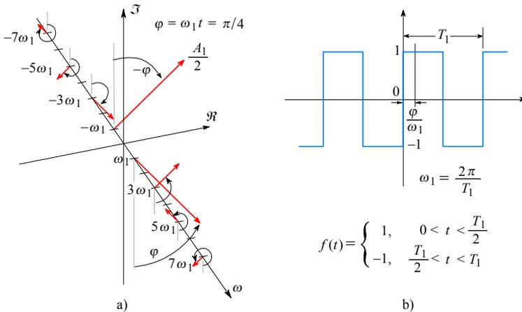
**Fig. 1.2.2:** As in Fig. 1.2.1, but at an instant  $t = (\pi/4 \pm 2n\pi)/\omega_1$ ; **a)** the spectrum, expressed by complex conjugate phasor pairs, corresponds to the instant  $t = \varphi/\omega_1$  in **b)**. To see the movie over one period click this link: [harmovie.gif](#) (we apologize for the bad quality resulting from the poor conversion from vector graphics to the bitmap format; readers who have access to Matlab are invited to run the 'harmovie.m' file).
