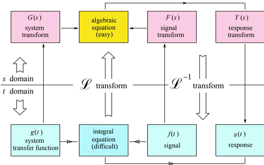
**Fig. 1.15.2:** Equivalence of the system response calculation in the time domain,  $f(t)*g(t)$ , and the frequency domain,  $F(s) \cdot G(s)$ . For analytical work the transform route is the easy way. For computer use the direct method is preferred.
