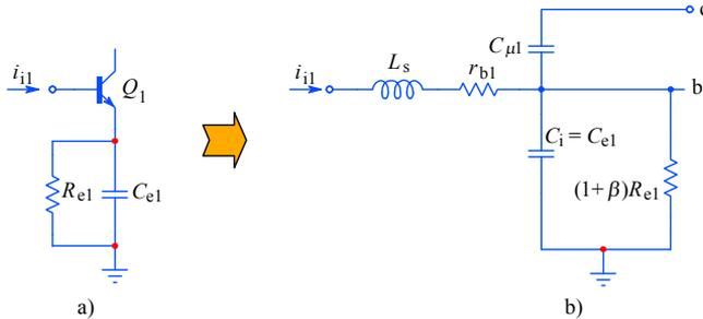
**Fig. 3.6.7:** The complete transistor input impedance: a) schematic; b) equivalent circuit, in which we include also the base lead inductance  $L_{b1}$ . The presence of the shunt resistance  $(1 + \beta) R_{e1}$  requires a modified interstage T-coil circuit.
