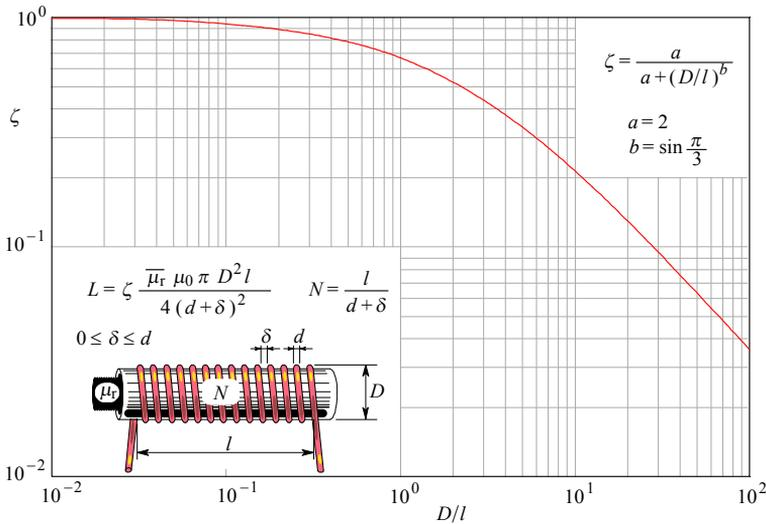
**Fig. 2.11.3:** The  $\zeta$  factor as a function of the coil diameter to length ratio,  $D/l$ . The equation shown in the upper right corner fits experimental data to better than 1%.
