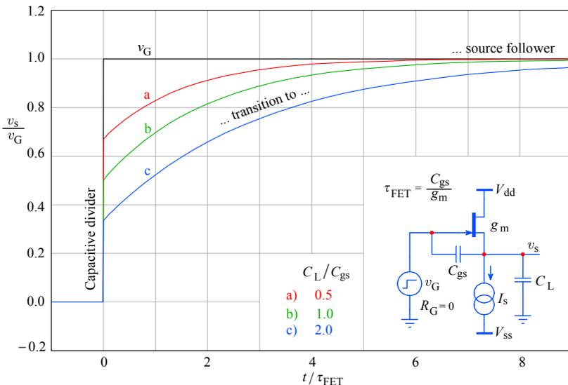
**Fig. 3.9.6:** The JFET source follower step response for the three capacitance ratios.
