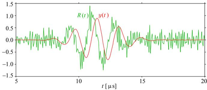
**Fig. 7.1.6:** The output spectrum is returned to time domain as  $y(t)$  and is compared with the input signal  $R(t)$ , in expanded time scale. Note the small change in amplitude, the reduced noise level and the envelope delay (approx.  $1/4$  period time shift), with little change in phase. The time shift is equal to  $1/2$  the number of samples of the filter impulse response.
