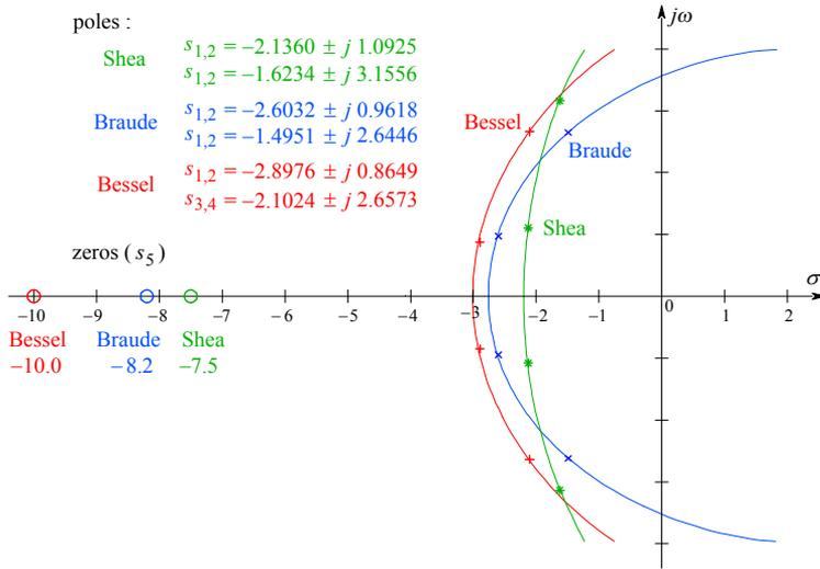
**Fig. 2.9.7:** The MFED shunt–series peaking circuit pole loci of the three different systems. The zero of each system is too far from the poles to have much influence. It is interesting how a similar step response can be obtained using three different optimization strategies. Strictly speaking, only the Bessel system is optimal.
