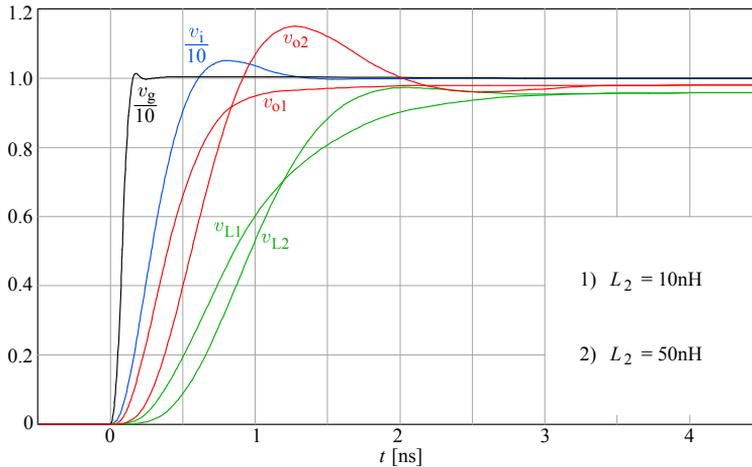
**Fig. 5.2.10:** Step response of the circuit in [Fig. 5.2.9](#). With a low  $L_1$ , a correctly damped  $L_2$ , and a good JFET, a 350 MHz bandwidth ( $v_{L2}$  rise time  $\approx 1$  ns), can be easily achieved. The source follower gain is a little less than one.  $v_o$  and  $v_L$  are drawn for the two  $L_2$  cases.
