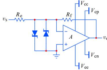
**Fig. 5.3.32:** The output buffer with a separate lower supply voltage can be used for output signal clipping with current feedback amplifiers. Since feedback is lost during clipping, the input stage must be protected from overdrive by anti-parallel Schottky diodes, which, inevitably, increase the input capacitance.
