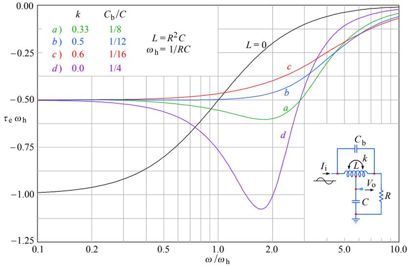
**Fig. 2.4.7:** The envelope delay of the T-coil: *a)* MFA, *b)* MFED, *c)* CD, *d)*  $k = 0$ . The T-coil circuit delay at low frequencies is exactly one half of that in the  $L = 0$  case.
