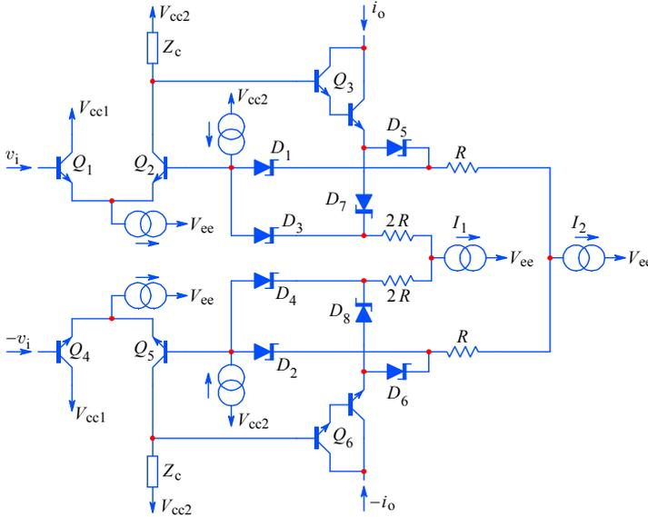
**Fig. 5.4.37:** Gain switching in steps was achieved by adding one or more emitter current sources ( $I_1, I_2, \dots$ ) with appropriate resistor values and Schottky diode pairs and switching on one current source at a time.
