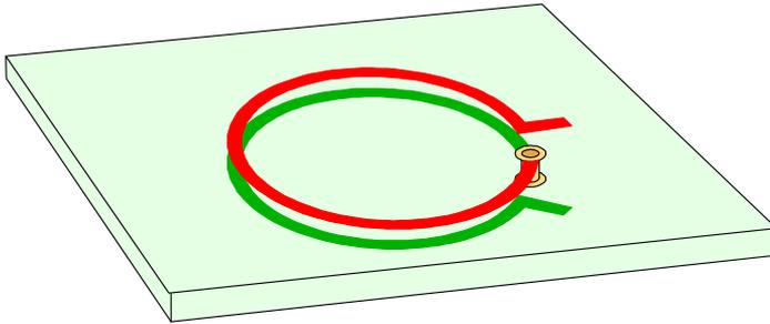
**Fig. 2.11.6:** A planar T-coil with a high coupling factor, realized on a conventional double-sided PCB. Multi-turn spiral structures are also possible, but need at least a three-layer board for making the inner to outer turn connections.
