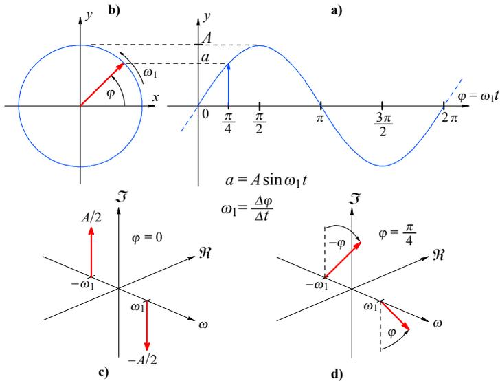
**Fig. 1.1.1:** Three different presentations of a sine wave: **a)** amplitude in time domain; **b)** a phasor of length  $A$ , rotating with angular frequency  $\omega_1$ ; **c)** two complex conjugate phasors of length  $A/2$ , rotating in opposite directions with angular frequency  $\omega_1$ , at  $\omega_1 t = 0$ ; **d)** the same as **c)**, except at  $\omega_1 t = \pi/4$ . To see the movie click on this link: [sinemovie.gif](#).
