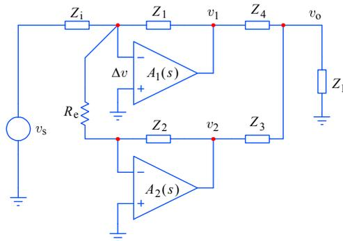
**Fig. 5.4.5:** ‘Error take off’ principle. The error  $\Delta v$  of the main amplifier, left by feedback, is taken by the auxiliary amplifier and fed forward to the load, where it is passively summed to the main output. The impedances  $Z_1$  to  $Z_4$  form the balancing bridge.
