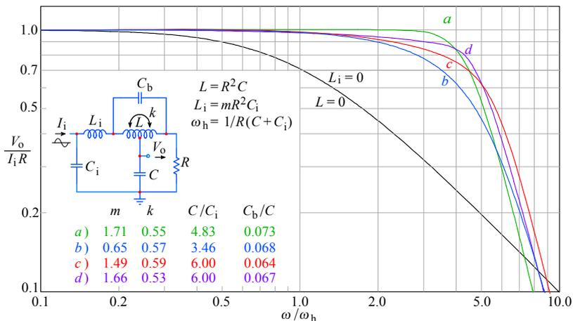
**Fig. 2.6.3:** Four-pole L+T peaking circuit frequency-response: *a)* MFA; *b)* MFED; *c)* Group C; *d)* Group A. In the non-peaking reference case both inductances are zero.
