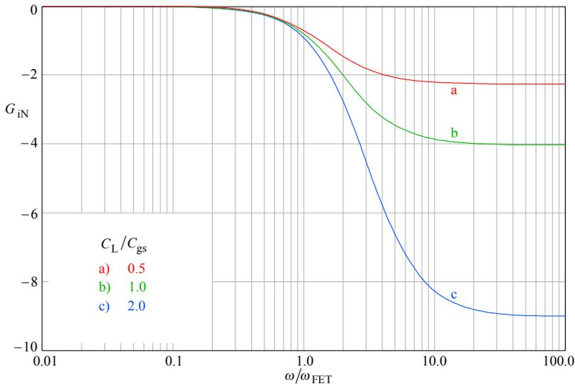
Fig. 3.9.10: Normalized negative input conductance  $G_{\text{IN}}$  vs. frequency.
