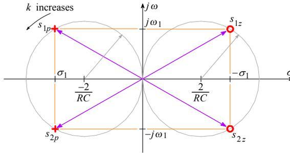
**Fig. 2.4.3:** The poles ( $s_{1p}$  and  $s_{2p}$ ) and zeros ( $s_{1z}$  and  $s_{2z}$ ) of the all pass transimpedance function corresponding to Eq. 2.4.26 and Fig. 2.4.1a. By changing the bridge capacitance  $C_b$  and the mutual inductance  $L_M$  (by the coupling factor  $k$ ) according to Eq. 2.4.19, both poles and both zeros travel along the circles shown.
