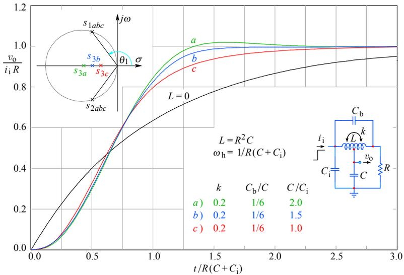
Fig. 2.5.11: Low coupling factor, Group 2: step response. The pole  $s_{3a}$  is slightly further away from the real axis than  $s_{3b}$  or  $s_{3c}$ , therefore causing an overshoot larger than in the MFED case. Both responses  $b$  and  $c$  are over-damped, reaching the final value much later than in the MFED case.
