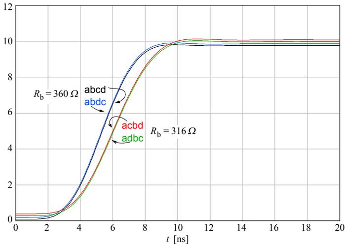
**Fig. 5.1.10:** If the high gain responses are recalculated by reducing  $R_b$  from the original  $360 \Omega$  to  $316 \Omega$ , the gain is nearly equal in all four cases. However, those pole assignments which put the poles with the higher imaginary part at the output stage still result in a slightly slower system.
