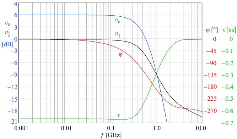
**Fig. 5.4.27:** Frequency domain performance of the Cascomp evolution amplifier. The bandwidth is a little over 400 MHz.
