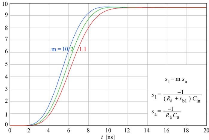
**Fig. 5.1.11:** If the real input pole  $s_1$  is at least twice as large as the system's real pole  $s_a$ , its influence on the step response can be seen merely as an increased envelope delay and a reduced overshoot, whilst the rise time remains nearly identical.
