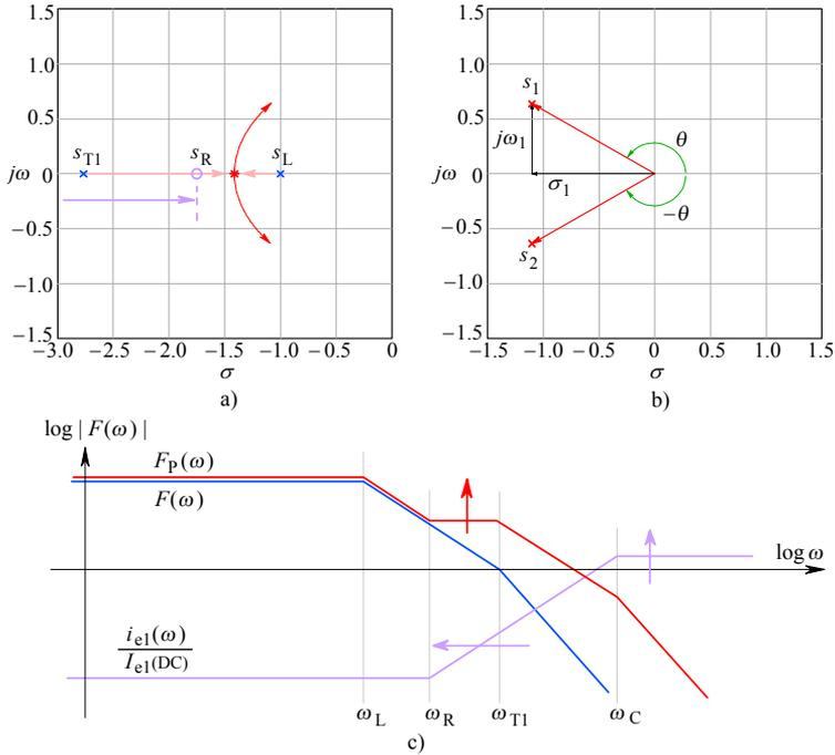
**Fig. 3.5.2:** Emitter peaking: a) two real poles travel towards each other when the emitter network zero goes from  $-\infty$  towards  $s_L$ , forming eventually a complex conjugate pair; b) poles for Eq. 3.5.14 for the 2<sup>nd</sup>-order Bessel (MFED) response. c) frequency response asymptotes — the bandwidth is extended to  $\omega_{T1}$  if  $\omega_R = \omega_L$ .
