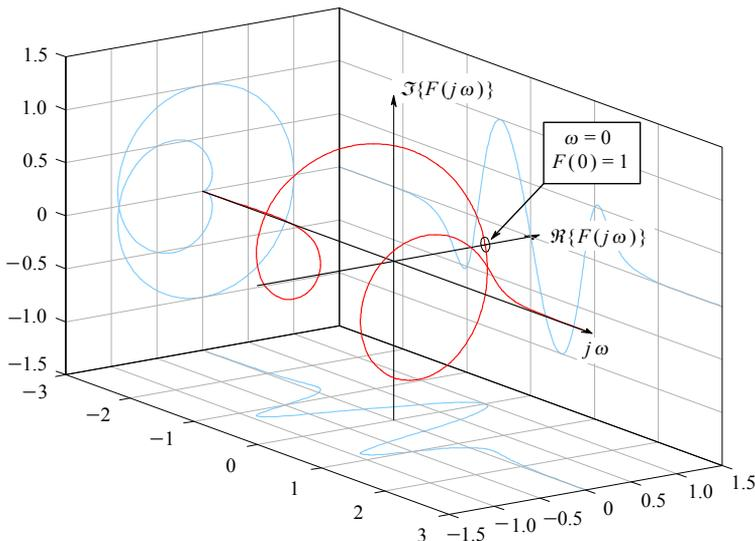
**Fig. 6.4.2:** The complex 3D plot of  $F(j\omega)$ . The response phasor rotates clockwise, going from negative to positive frequency. The distance from the frequency axis is the magnitude. The circle on the real axis marks the DC response point. The Nyquist plot (see [Fig. 6.4.3](#)) usually shows only the  $\omega > 0$  part, viewing in the  $-j\omega$  direction. The three projections are plotted to help those readers who do not have access to Matlab to visualize the shape.
