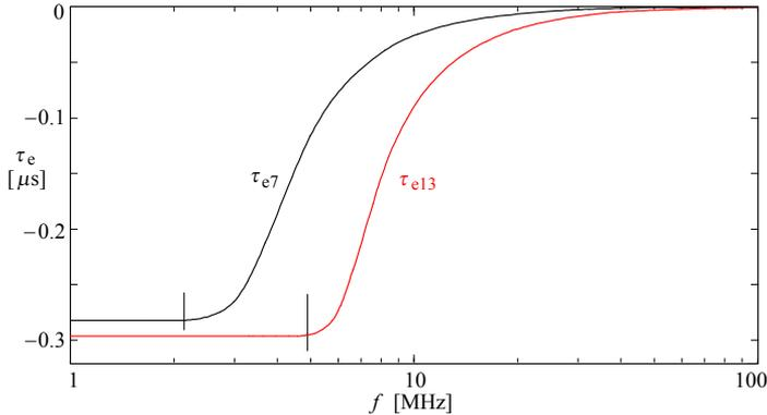
**Fig. 7.2.14:** Envelope delay comparison of the original 7-pole analog only filter  $\tau_{e7}$  and the mixed mode 13-pole Bessel–Thomson filter  $\tau_{e13}$ . The 7-pole analog only filter is linear to a little over 2 MHz, while the 13-pole mixed mode filter is linear well into the stop band, up to almost 5 MHz, more than doubling the useful linear phase bandwidth.
