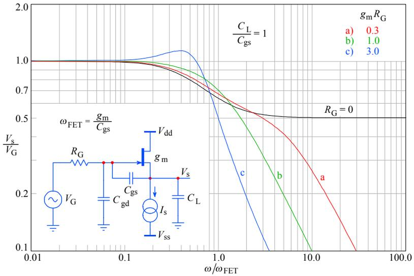
**Fig. 3.9.7:** The JFET source follower frequency response for a ratio  $C_L/C_{gs} = 1$  and a variable signal source impedance, so that  $R_G g_m$  is 0.3, 1, and 3, respectively. Note the response peaking for  $g_m R_G = 3$ .
