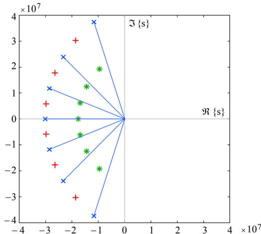
**Fig. 7.2.11:** The 13-pole mixed mode system, the analog part marked by 'x', the digital by '+'; compared with the original 7-pole analog only filter, marked by '\*'. Note the difference in pattern size (proportional to bandwidth!).
