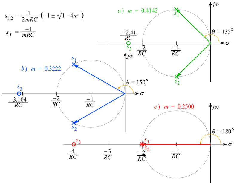
**Fig. 2.7.6:** Shunt peaking circuit placement of the poles and the zero: **a)** MFA; **b)** MFED; **c)** CD. Note the position of the zero  $s_3$  at the far left of the real axis. Although far from the poles, its influence on the response is notable in each case.
