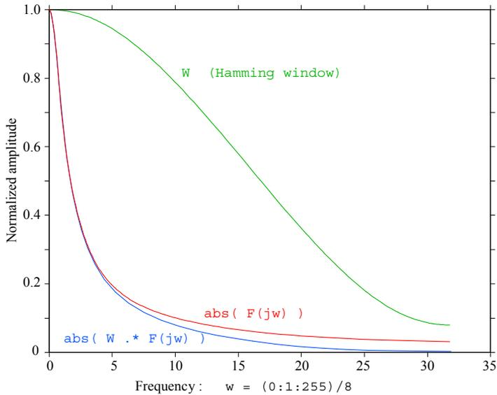
**Fig. 6.5.4:** Windowing example. The 1<sup>st</sup>-order frequency response (only the magnitude is shown on plot) is multiplied element by element by the Hamming type of window function in order to reduce the influence of high frequencies and improve the impulse response calculation accuracy. Note that the window function is real only, affecting equally the system real and imaginary part, thus the phase information is preserved and only the magnitude is corrected.
