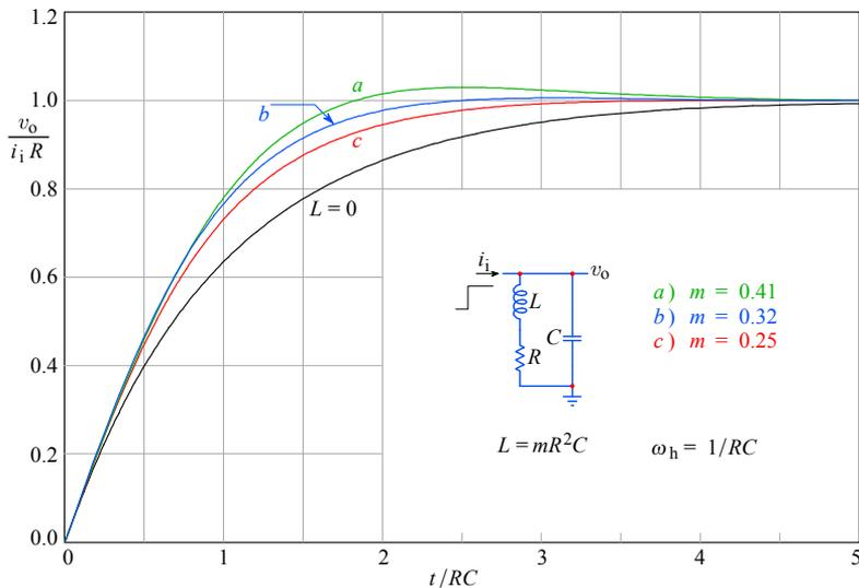
**Fig. 2.7.5:** Shunt peaking circuit step response: **a)** MFA; **b)** MFED; **c)** CD. The non-peaking case ( $L = 0$ ) is the reference. The difference between the number of poles and the number of zeros is only 1 for the shunt peaking systems, therefore the starting slope of the step response is similar to that of the non-peaking first-order system.
