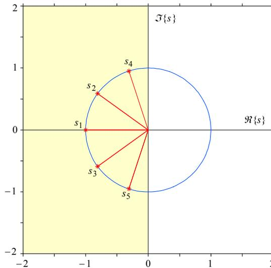
**Fig. 6.3.1:** The 5<sup>th</sup>-order Butterworth system poles in Cartesian coordinates of the complex plane. The left half of the figure is the  $s$  domain over which the magnitude in [Fig. 6.4.1](#) is plotted.
