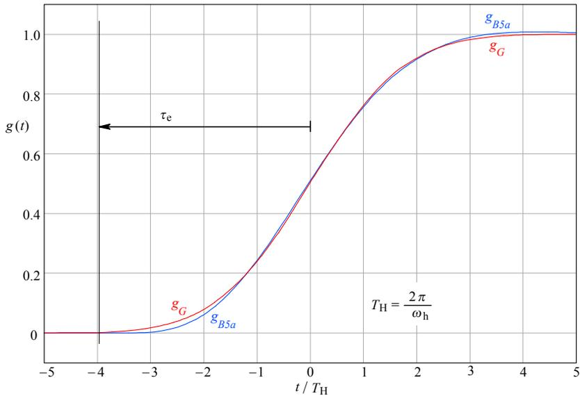
**Fig. 4.4.9:** Step response of a hypothetical system,  $g_G$ , having the ideal Gaussian frequency response with no phase shift, as the one in Fig. 4.4.7 and 4.4.8. Compare it with the step response of a 5<sup>th</sup>-order Bessel system,  $g_{B5a}$ , with modified Bessel poles, Table 4.5.1, and envelope delay compensated ( $\tau_e = -3.94 T_H$ ) for minimal difference in the half amplitude region.
