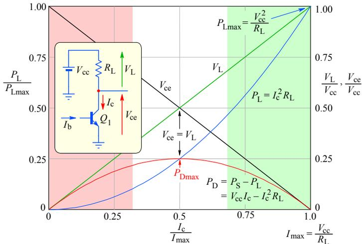
**Fig. 3.4.9:** The optimum bias point is when the voltage across the load is equal to the voltage across the transistor. This is optimal both in the sense of thermal stability, as well as in the available signal range sense.
