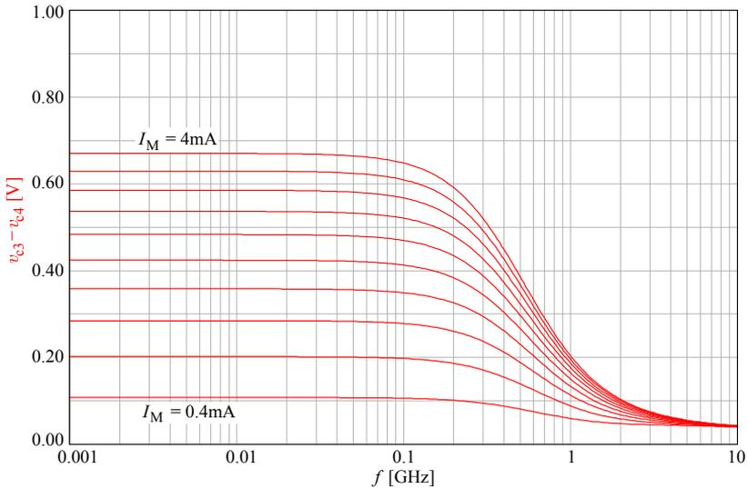
**Fig. 5.4.41:** The Gilbert multiplier bandwidth is almost constant over the 10:1 modulation current range.
