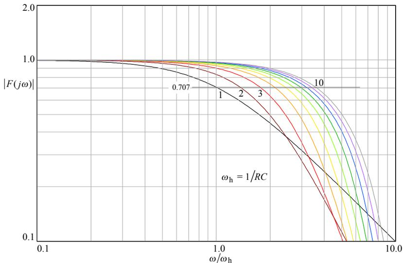
**Fig. 4.4.2:** Frequency-response magnitude of systems with Bessel poles for order  $n = 1 \dots 10$ .
