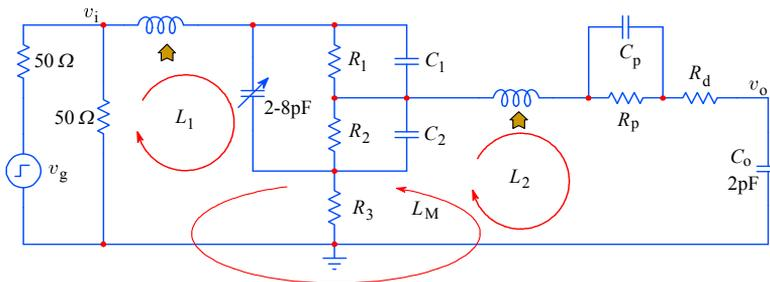
**Fig. 5.2.8:** Inductances owed to circuit loops can be modeled as inductors in series with the signal path. Note that in addition to the two self inductances there is also a mutual inductance between the two. The actual values depend on the loop's size, which in turn depends on the size of the components and the circuit's layout. Smaller loops have less inductance. Mutual inductance can be reduced by shielding, although this can increase the stray capacitances.
