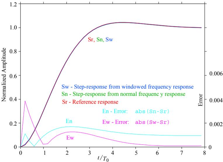
**Fig. 6.5.7 and 6.5.8:** As in Fig. 6.5.5 and 6.5.6, but with 40 samples of a 2<sup>nd</sup>-order Butterworth system. The impulse response error for the windowing procedure is higher at the beginning, but falls off more quickly, therefore the step response final value error is still much lower (note that the step response error plots are enlarged 100×). The oscillations in error plots, owed to the Gibbs' effect, also begin to show.
