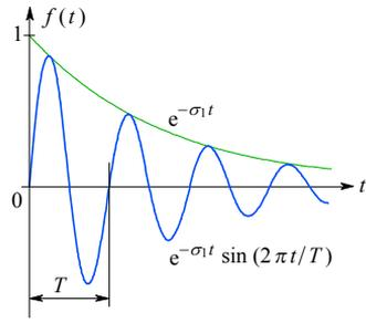
Fig. 1.5.6: Damped oscillations.
