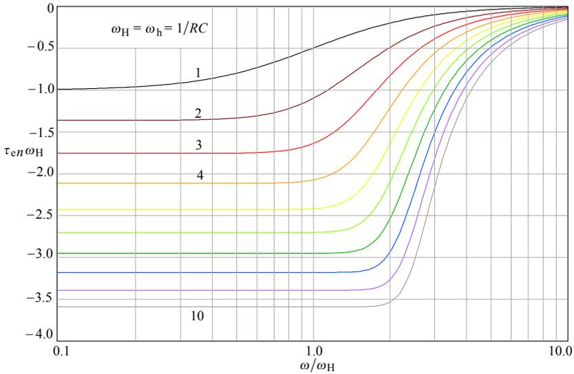
**Fig. 4.4.12:** Envelope delay of systems with normalized Bessel poles of the order  $n = 1-10$ . Although the bandwidth is the same, the delay flatness extends progressively with system order, already reaching beyond the system cut off frequency for  $n = 5$ .
