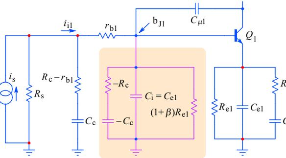
**Fig. 3.5.3:** The impedances in the emitter are reflected into the base junction of  $Q_1$ . The emitter peaking components  $R$  and  $C$  are reflected into **negative** elements  $-R_c$  and  $-C_c$ , which must be compensated by adding externally an equal and positive  $R_c$  and  $C_c$ ; for proper compensation  $r_{b1}$  must be subtracted from  $R_c$ .
