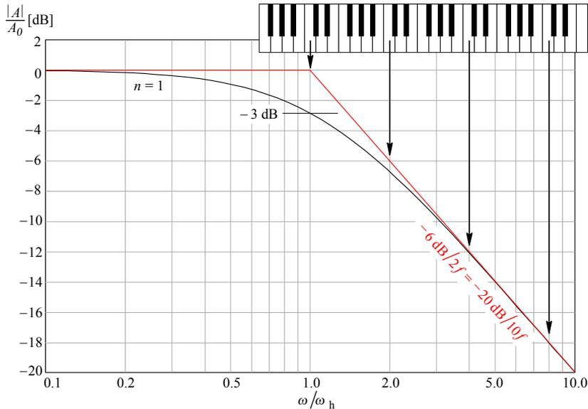
**Fig. 4.1.3:** The first-order system response and its asymptotes. Below the cut off, the asymptote is the level equal to the system gain at DC (normalized here to 0 dB). Above the cut off, the slope is  $-6$  dB/octave (an octave is a frequency span from  $f$  to  $2f$ ), which is also equal to  $-20$  dB/decade (a frequency decade is a span from  $f$  to  $10f$ ).
