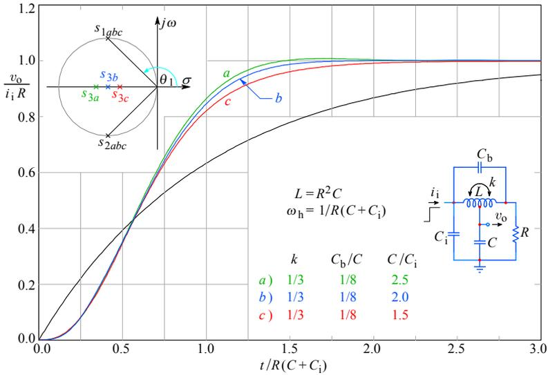
Fig. 2.5.9: Low coupling factor, Group 1: step response. In all three cases the real pole  $s_3$  is placed closer to the origin (becoming dominant) than in the MFA and MFED case, making the responses more similar to the CD case. The characteristic circle of the complex conjugate pole pair has a slightly different diameter in each case.
