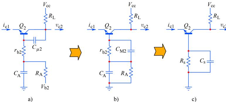
**Fig. 3.4.7:** The  $Q_2$  emitter input impedance compensation by the added base network  $R_A$  and  $C_A$  (see also [Fig. 3.2.7](#)), making it capacitive at high frequencies. By altering the value slightly it can also be used to compensate the stray base inductance.
