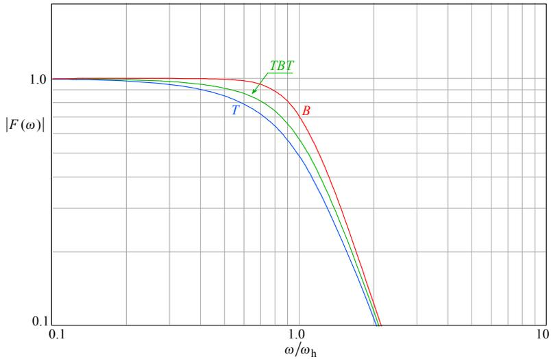
**Fig. 4.5.2:** Frequency response's magnitude of the Transitional Bessel-Butterworth three-pole system (TBT), along with the modified Bessel (T) and Butterworth (B) responses.
