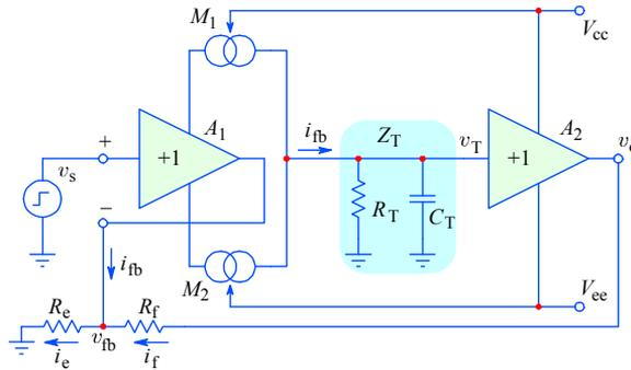
Fig. 5.3.8: Current feedback amplifier model used for the analysis.
