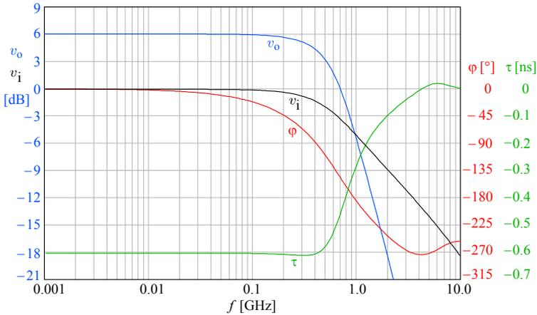
**Fig. 5.4.35:** Frequency domain performance of the amplifier in Fig. 5.4.34. The bandwidth of the simulated circuit is about 500 MHz, but this is owed to the transistor used (BF959) and the frequency compensation network adjusted in accordance, therefore the graph is not representative of the actual M377 IC performance.
