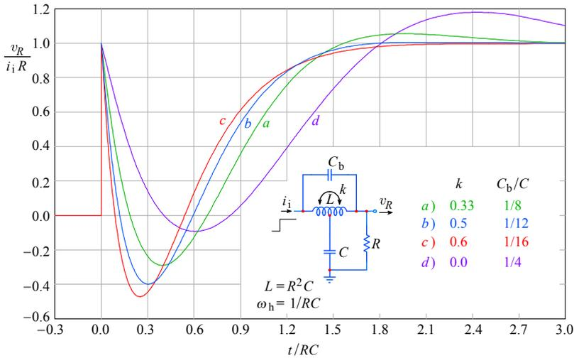
**Fig. 2.4.9:** The step response of the T-coil circuit, but now with the output from the loading resistor  $R$  (this is interesting for cascading stages, as explained later). As before, *a*) MFA, *b*) MFED, *c*) CD, and *d*)  $k = 0$ . The system has the characteristics of an all pass filter.
