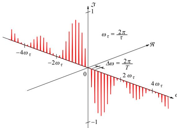
**Fig. 1.3.2:** Complex spectrum of the waveform in Fig. 1.3.1.
