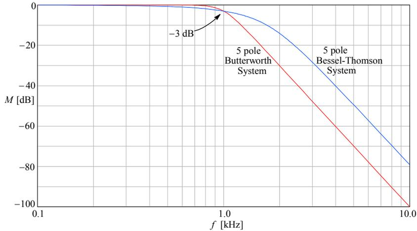
**Fig. 6.7.2:** Frequency responses of the Butterworth and Bessel–Thomson system. For an equal cut off frequency ( $f_h = 1$  kHz), the Butterworth system stop band attenuation is about an order of magnitude ( $10\times$  or 20 dB) better than that of the Bessel–Thomson.
