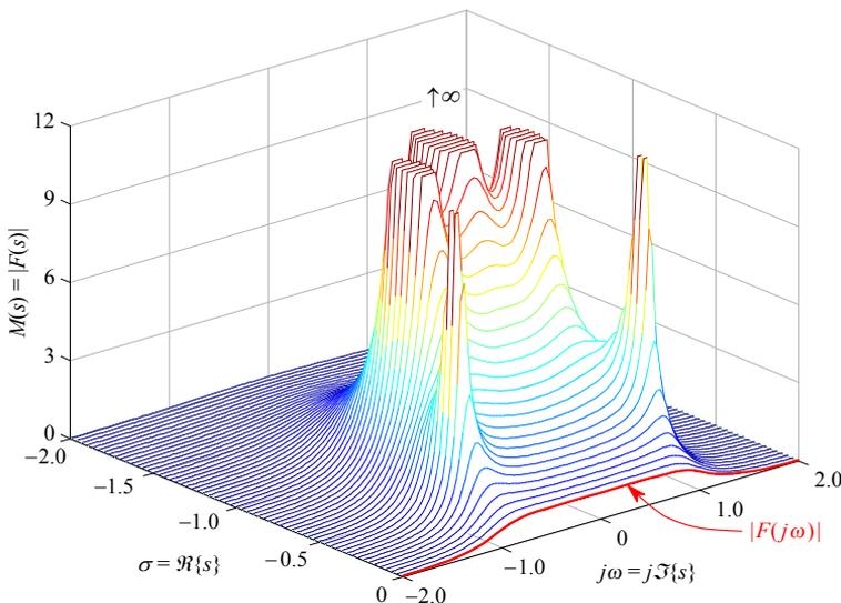
**Fig. 6.4.1:** The 5<sup>th</sup>-order Butterworth system magnitude, plotted over the same  $s$ -domain as the shaded left half of Fig. 6.3.1. The surface represents  $|F(s)|$ , but limited in height in order to reveal the low level details. Its shape above the  $j\omega$  axis is  $|F(j\omega)| = M(\omega)$ .
