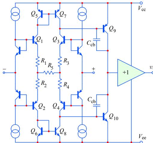
**Fig. 5.3.24:** An interesting combination of circuits in Fig. 5.3.22 and 5.3.23 is the so called ‘Quad Core’ structure, [Ref. 5.32]. Here both the inverting and the non-inverting input buffer currents are combined by the current mirrors to drive the  $C_{cb}$  of  $Q_{9,10}$ . The non-labeled transistors provide the  $V_{be}$  compensation for  $Q_{1-4}$ . Typical representatives are Analog Devices’ AD-8047, AD-9631, AD-8041 and others.
