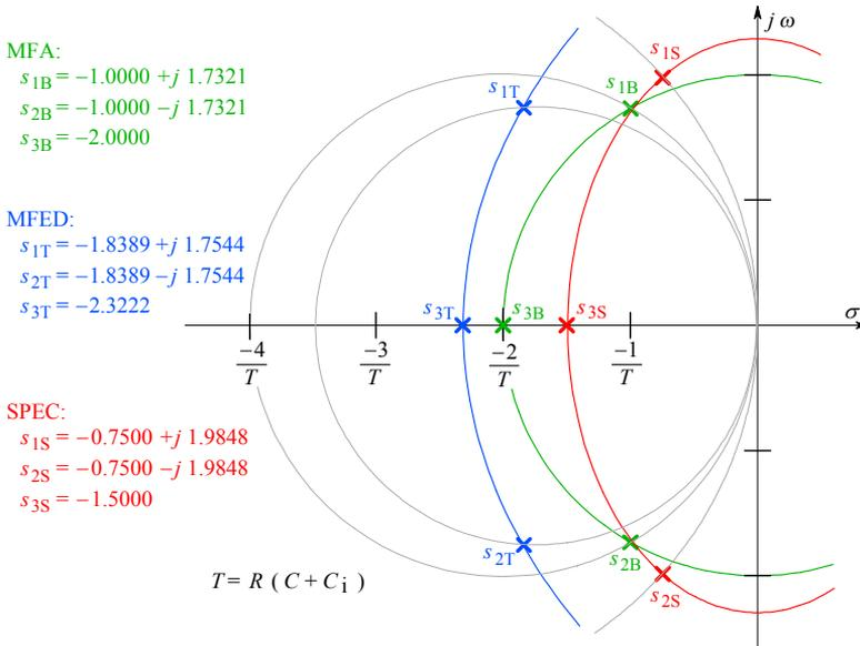
**Fig. 2.3.6:** Pole patterns of the 3-pole series peaking circuit for the MFA, the MFED, and the SPEC case. The curves on which the poles lie are: a circle with the center at the origin for MFA; an ellipse with both foci on the real axis (the nearer at the origin) for the MFED; and an ellipse with both foci on the imaginary axis for the SPEC case (which is effectively a Chebyshev-type pole pattern). Also shown are the characteristic circles of each complex conjugate pole pair.
