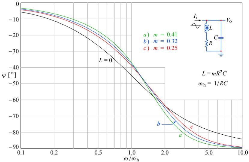
**Fig. 2.7.3:** Shunt peaking circuit phase response: *a)* MFA; *b)* MFED; *c)* CD. The non-peaking case ( $L = 0$ ) is the reference. The system zero causes the high frequency phase to be  $-90^\circ$ , the same as for the non-peaking system.
