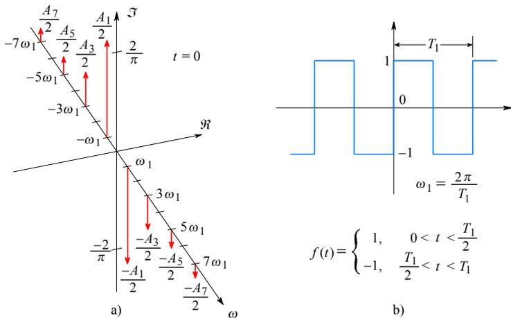
**Fig. 1.2.1:** A square wave, as shown in **b)**, has an infinite number of odd-order frequency components, of which the first 4 complex-conjugate phasor pairs are drawn in **a)** at time  $t = (0 \pm 2n\pi)/\omega_1$ , where  $n$  is an integer representing the number of the period.
