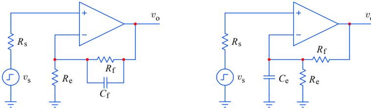
**Fig. 5.3.13:** a) A unity gain compensated voltage feedback amplifier remains stable with capacitive feedback, whilst in b) it is unstable. In contrast, the stability of a current feedback amplifier is upset by either a)  $C_f$  in parallel with  $R_f$ , or b)  $C_e$  in parallel with  $R_e$ .
