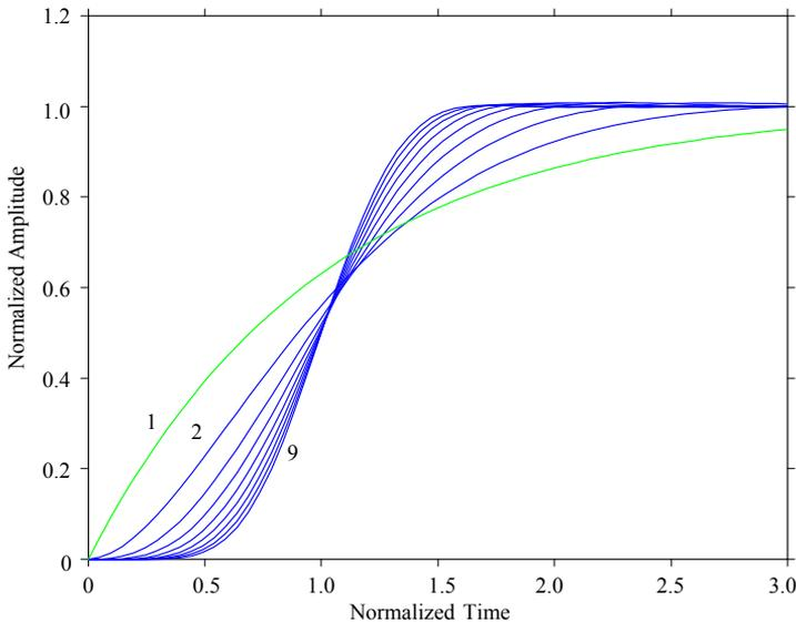
**Fig. 6.5.11:** Step responses of Bessel–Thomson systems (normalized to equal envelope delay), of order 2 to 9, including the 1<sup>st</sup>-order step response for comparison. Note the half amplitude delay approaching 1 and the bandwidth improving (shorter rise time) as the system order increases. The TRESP algorithm execution speed was tested by creating this figure.
