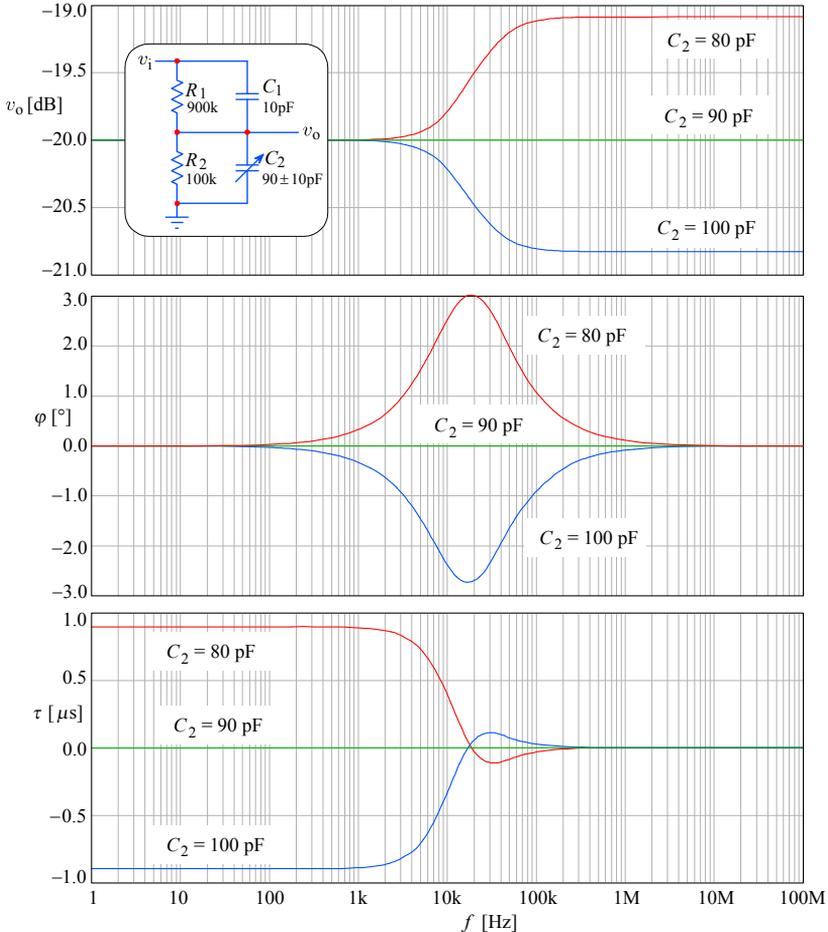
**Fig. 5.2.3:** The attenuator magnitude, phase, and envelope delay responses for the correctly compensated case (flat lines), along with the under- and over-compensated cases ( $C_2$  is trimmed by  $\pm 10$  pF). Note that these same figures apply also to oscilloscope passive probe compensation, demonstrating the importance of correct compensation when making single channel pulse measurements and two channel differential measurements.
