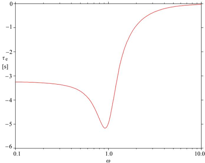
**Fig. 6.4.8:** The envelope (group) delay vs. frequency of the 5<sup>th</sup>-order Butterworth system. The delay is the largest for frequencies where the phase has the greatest slope.
