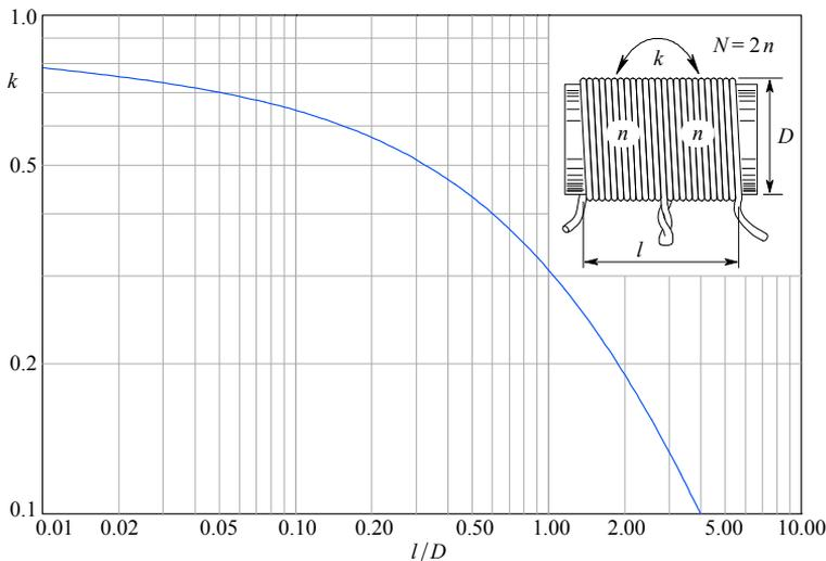
Fig. 2.11.2: T-coil coupling factor  $k$  as a function of the coil's length to diameter ( $l/D$ ) ratio.
