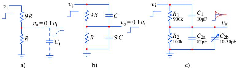
**Fig. 5.2.2:** The 10:1 attenuator; **a) resistive:** with  $R = 100$  k $\Omega$ , the following stage input capacitance of just 1 pF would limit the bandwidth to only 1.77 MHz; **b) compensated:** the capacitive divider takes over at high frequencies but the input capacitance of the following stage of 1 pF would spoil the division by 1%; **c) adjustable:** in practice, the capacitive divider is trimmed for a perfect step response.
