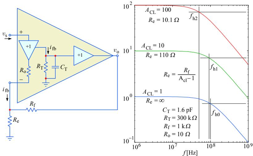
**Fig. 5.3.12:** The bandwidth of an actual current feedback amplifier is gain dependent, owing to a small but finite inverting input resistance  $R_o$ . The nominal bandwidth of 100 MHz at unity gain is reduced to 90 MHz at the gain of 10 and to only 50 MHz at the gain of 100 if  $R_o$  is 10  $\Omega$ . Nevertheless, this is still much better than in voltage feedback amplifiers.
