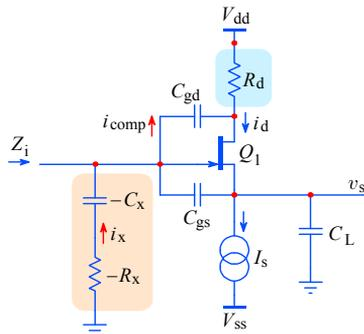
**Fig. 3.9.13:** Alternative compensation of the input impedance negative components, using negative feedback from the JFET drain.
