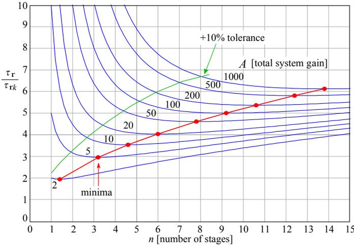
**Fig. 4.1.9:** Minimal relative rise time as a function of the number of stages  $n$  and the total system gain  $A$ . Close to the minima the curves are relatively flat, so in practice we can trade off, say, a 10% increase in the system rise time and reduce the required number of stages accordingly; i.e., to achieve the gain of 100, only 5 stages could be used instead of 9, with a slight rise time increase.
