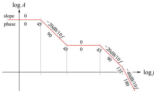
**Fig. 5.3.15:** An arbitrary example of the phase angle estimated from the gain magnitude, its slopes and various breakpoints. If two breakpoints are relatively close the phase would not actually reach the value predicted from the slope value, but an intermediate value instead.
