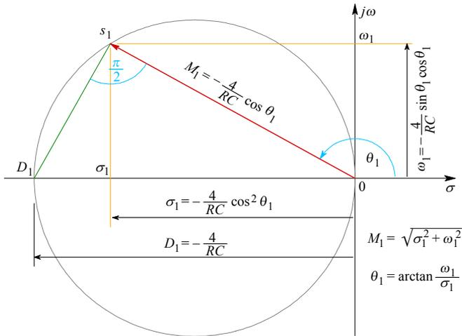
**Fig. 2.5.3:** The basic trigonometric relations of the main parameters for one of the poles of the T-coil circuit. Knowing one pair of parameters, it is possible to calculate the rest by these simple relations.
