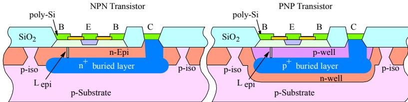
**Fig. 5.3.6:** Cross-section of the Complementary-Bipolar process.
