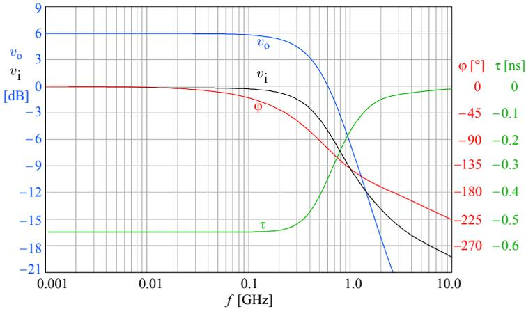
**Fig. 5.4.12:** Frequency domain performance of a simple differential cascode amplifier of Fig. 5.4.11 (no error correction) used in the test set up circuit of Fig. 5.4.10. This will be used as the reference for all other circuits. The bandwidth achieved is a little over 400 MHz.
