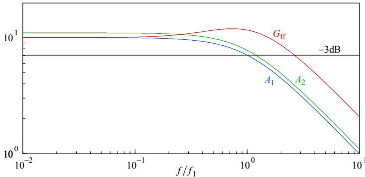
**Fig. 5.4.3:** The feedforward amplifier bandwidth  $G_{ff}$  is highest (and optimized in the sense of lowest gain  $\times$  bandwidth requirement of the auxiliary amplifier) if both amplifiers have the same bandwidth and the gains equal to  $1/\beta$ . In this figure  $1/\beta = 10$ ,  $A_{01} = 10$ , and  $A_{02} = 11$  (in order to distinguish  $A_2$  from  $A_1$  more easily). If  $s_1 \neq s_2$  the  $G_{ff}$  bandwidth will be lower.
