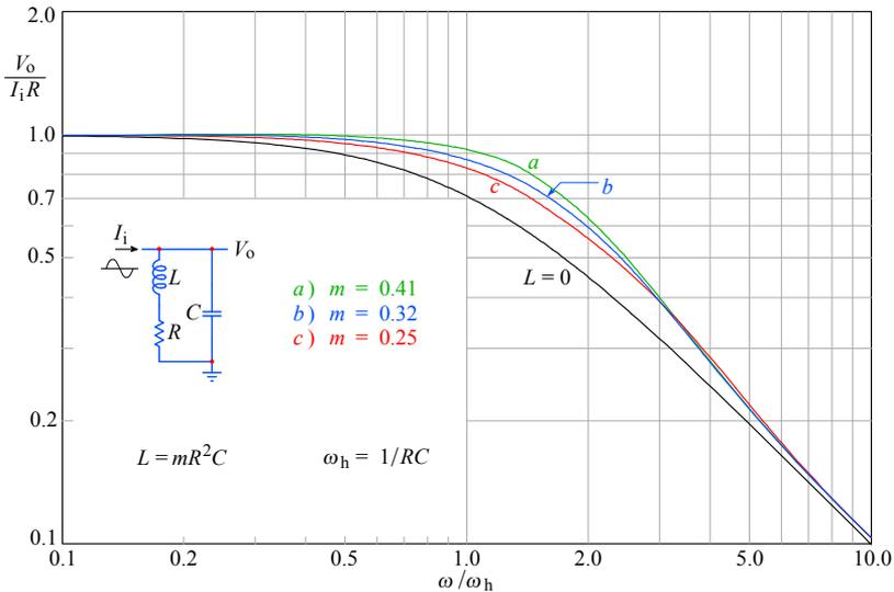
**Fig. 2.7.2:** Shunt peaking circuit frequency response: *a*) MFA; *b*) MFED; *c*) CD. As usual, the non-peaking case ( $L = 0$ ) is the reference. The system zero causes the high-frequency asymptote to be the same as for the non-peaking system.
