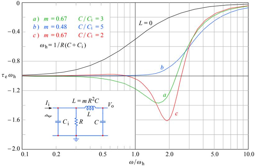
**Fig. 2.3.4:** Envelope delay of the third-order series peaking circuit for some characteristic values of  $m$ : *a*) MFA; *b*) MFED; *c*) SPEC; the non-peaking ( $L = 0$ ) case is the reference. Note the MFED flatness extending beyond  $\omega_h$ .
