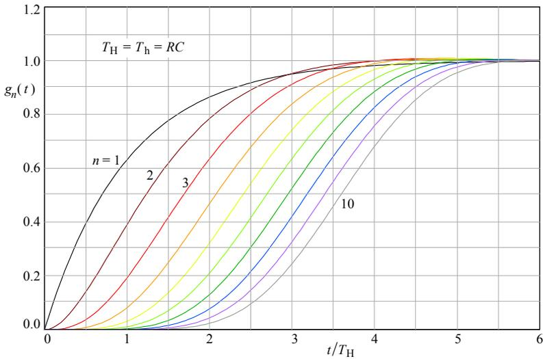
**Fig. 4.4.13:** Step response of systems with normalized Bessel poles of order  $n = 1-10$ . Note the half amplitude slope being almost equal for all systems, indicating an equal system cut off frequency.
