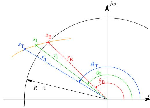
**Fig. 4.5.1:** Pole interpolation procedure. Butterworth (index B) and Bessel poles (index T) are expressed in polar coordinates,  $s(r, \theta)$ . The trajectory going through both poles is the interpolation path required to obtain the transitional pole  $s_I$ .
