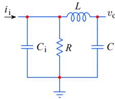
Fig. 2.3.1: The three-pole series peaking circuit.
