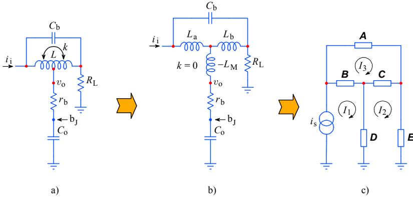
**Fig. 3.6.2:** a) The T-coil loaded by the simplified input impedance; b) the equivalent T-coil circuit in which  $k$  is substituted by  $-L_M$ ; c) the equivalent branch impedances and the three current loops.
