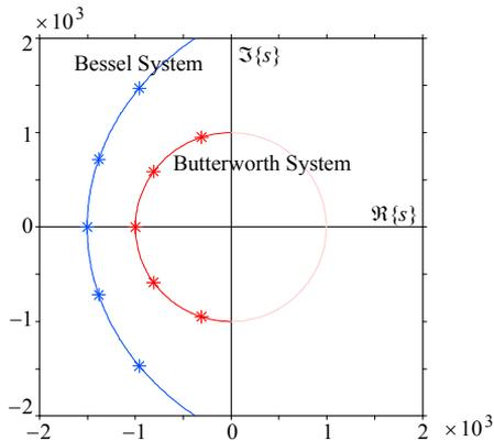
**Fig. 6.7.1:** The Butterworth poles (on the unit cycle) and the Bessel–Thomson poles (on the fitted ellipse). Note that for the same bandwidth (1 kHz) the values of Bessel–Thomson poles are much larger, but with a lower ratio of the imaginary to the real part.
