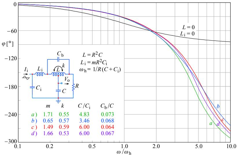
**Fig. 2.6.5:** Four-pole L+T peaking circuit phase response: *a*) MFA; *b*) MFED; *c*) Group C; *d*) Group A. The non-peaking case, in which both inductors are zero, has a  $90^\circ$  maximum phase shift; all other cases, being of 4<sup>th</sup>-order, have a  $360^\circ$  maximum phase shift.
