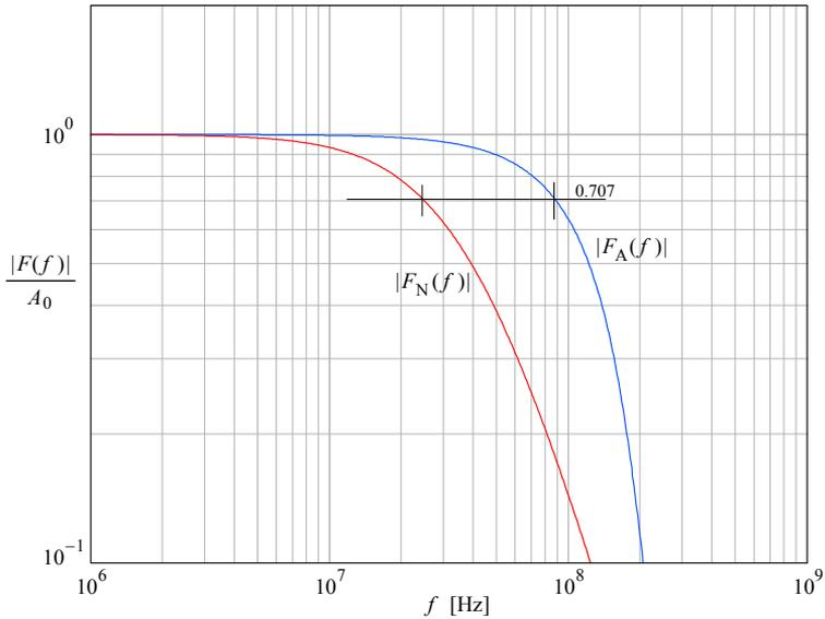
**Fig. 5.1.6:** The gain normalized magnitude vs. frequency of the 7-pole compensated system  $|F_A(f)|$  and the 2-pole non-compensated system,  $|F_N(f)|$ . The bandwidth of  $F_N$  is about 25 MHz and the bandwidth of  $F_A$  is about 88 MHz, more than 3.5 times larger.
