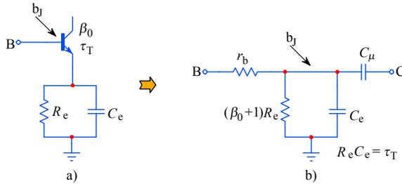
**Fig. 3.2.9:**  $R_e C_e$  network transformation: a) schematic; b) equivalent circuit. The symbol  $b_j$  represents the internal base junction.
