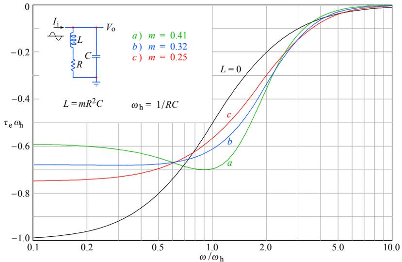
**Fig. 2.7.4:** Shunt peaking circuit envelope delay: *a)* MFA; *b)* MFED; *c)* CD. The non-peaking case ( $L = 0$ ) is the reference. The peaking systems have a higher bandwidth, and consequently a lower delay at DC than the non-peaking system.
