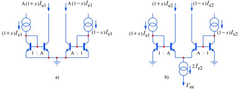
**Fig. 5.4.42:** Another way of developing the Gilbert multiplier is by interconnecting two current mirrors into a differential amplifier, whose input nonlinearity is compensated by the nonlinearity of the two grounded transistors.
