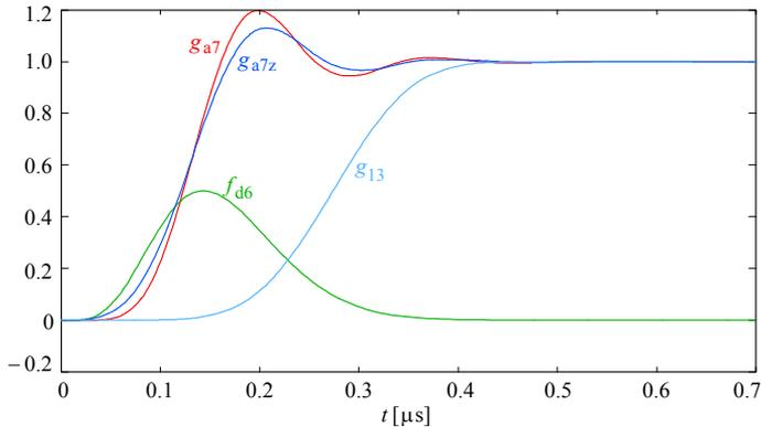
**Fig. 7.2.19:** The step response of the 7-pole analog filter  $g_{a7}$  is modified by the 4 zeros into  $g_{a7z}$ . Because the alias spectrum is narrower the bandwidth can be increased. The mixed mode system step response  $g_{13}$  has a rise time of less than 150 ns (in contrast with the 180 ns for the case with no zeros).
