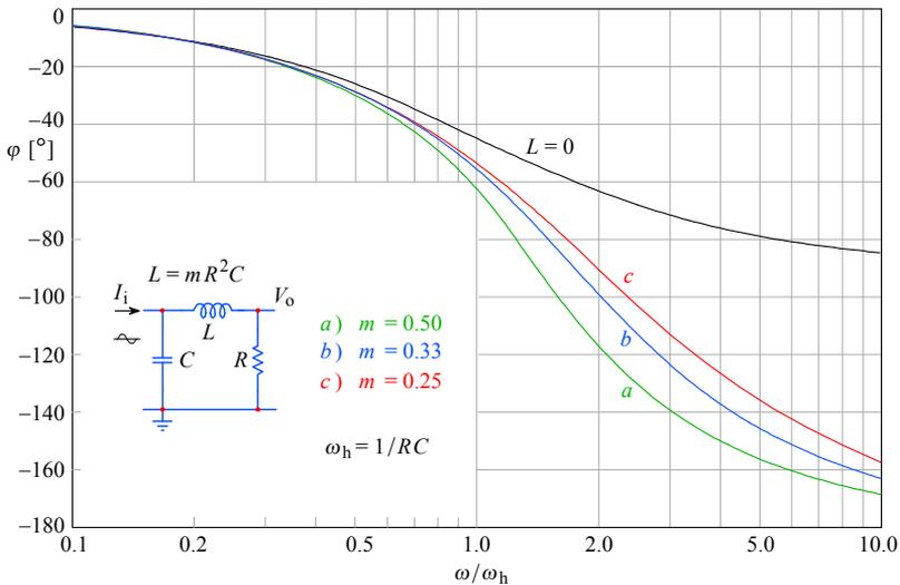
**Fig. 2.2.4:** Phase response of the series peaking circuit for *a)* MFA, *b)* MFED and *c)* CD case, compared with the non-peaking response ( $L = 0$ ). The phase angle scale was converted from radians to degrees by multiplying it by  $180/\pi$ . For  $\omega \rightarrow \infty$  the non-peaking (single-pole) response has its asymptote at  $90^\circ$ , whilst the second-order peaking systems have their asymptote at  $180^\circ$ .
