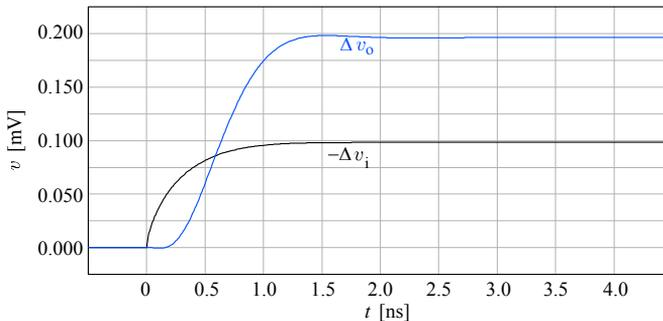
Fig. 5.4.23: Time domain performance of the 'Cascomp' amplifier. The rise time is about 0.7 ns and the initial undershoot is very low.
