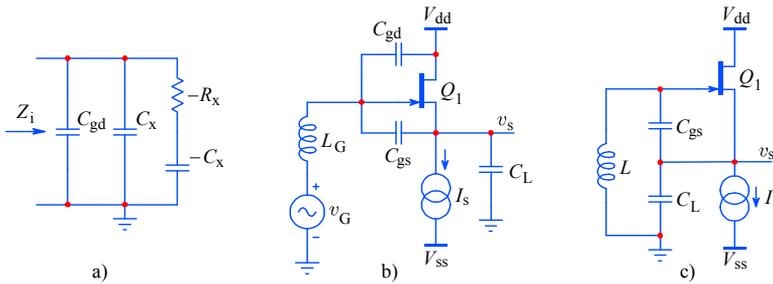
**Fig. 3.9.9:** a) The equivalent input impedance of the capacitively loaded JFET source follower has negative components which can be a nuisance if, as in b), the signal source has an inductive impedance, forming c) a familiar Colpitts oscillator. If  $C_{gd}$  is small, the circuit will oscillate for a broad range of inductance values.
