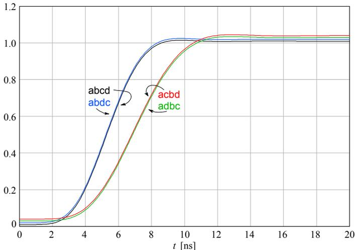
**Fig. 5.1.8:** The normalized step responses of the four possible combinations of pole assignments. There are two pairs of responses, here spaced vertically by a small offset to allow easier identification. One of the two faster responses (labeled ‘abcd’) is the one for which the detailed analysis has been given in the text.
