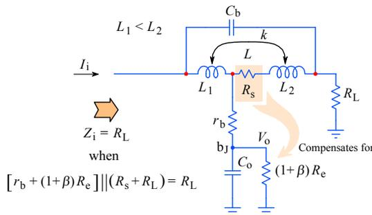
**Fig. 3.6.8:** The resistance  $R_s$  in series with  $L_2$  is inserted near the T-coil tap to compensate the error in the impedance seen by the input current at low frequencies, owed to the parallel connection of  $R_L || [r_b + (1 + \beta) R_e]$ .
