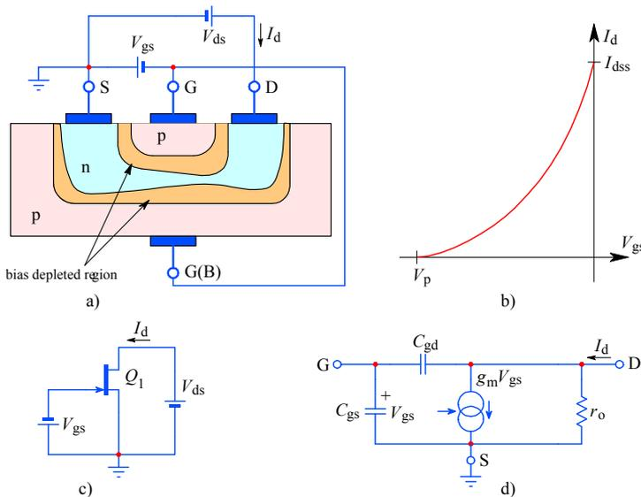
**Fig. 5.2.19:** a) A typical n-channel JFET structure cross-section under the bias condition. The p-type substrate is in contact with the p-type gate. The n-type channel is formed between the source and the drain. The bias voltage depletes the channel. b) The  $V_{gs}$ – $I_d$  characteristic. c) The symbolic circuit. d) The equivalent circuit model.
