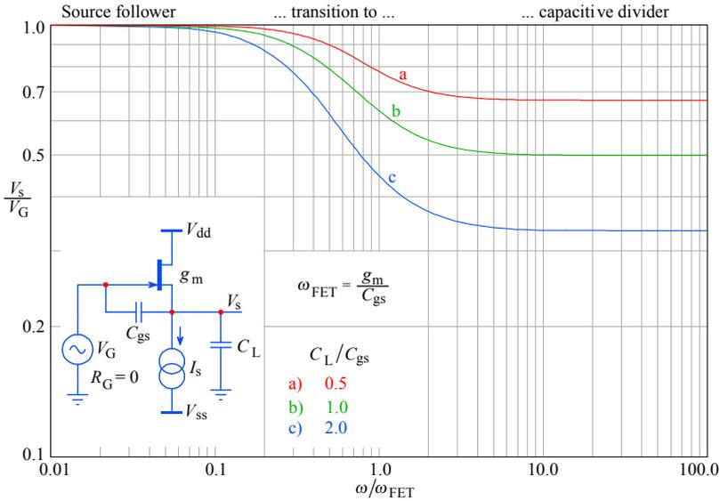
**Fig. 3.9.3:** Magnitude of the frequency response of the JFET source follower for three different capacitance ratios  $C_L/C_{gs}$ . The pole  $s_3 = -1/R_G C_i$  has not been taken into account here (see Fig. 3.9.7 and Fig. 3.9.8).
