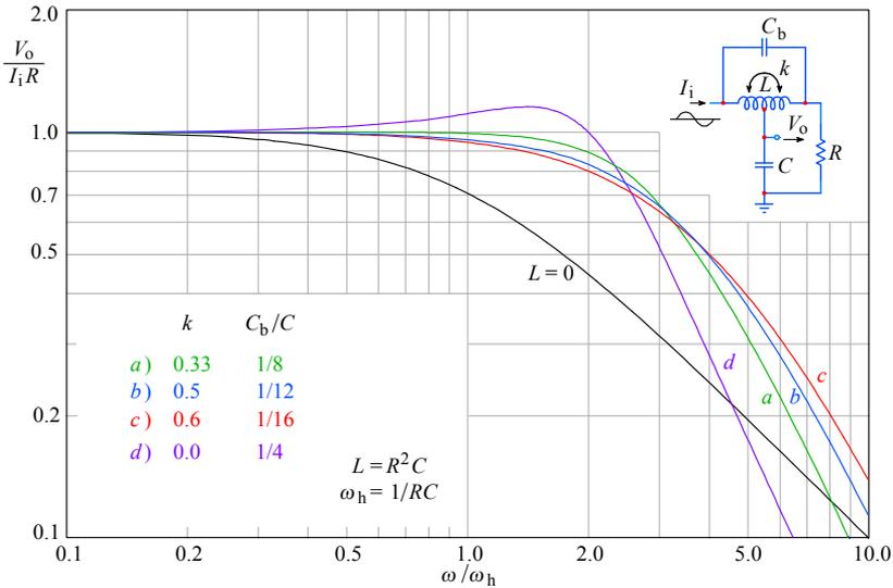
**Fig. 2.4.5:** The frequency response magnitude of the T-coil, taken from the coil center tap. The curve *a*) is the MFA (Butterworth) case, *b*) is the MFED (Bessel) case, *c*) is the critical damping (CD) case and *d*) is the no-coupling ( $k = 0$ ) case. The non-peaking ( $L = 0$ ) case is the reference. The bandwidth extension is notably larger, not only compared with the two-pole series peaking, but also to the three-pole series peaking circuit.
