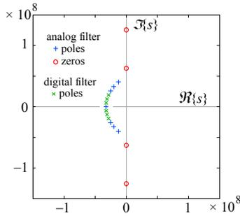
**Fig. 7.2.16:** An example of a similar mixed mode filter, but with the analog filter using two pairs of imaginary zeros, one pair at the sampling frequency and the other pair at the Nyquist frequency.
