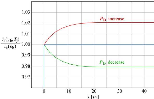
**Fig. 3.4.8:** The collector current step response is distorted by a long term thermal drift following the transient. Depending on the chosen DC bias point, the output can either increase or decrease relative to the ideal response. In addition to the junction thermal time constant, there can also be a slower one, owed to the transistor case temperature change.
