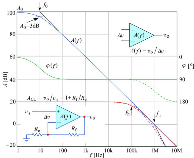
**Fig. 5.3.2:** A typical opamp open loop gain and phase compared to the closed loop gain. The dashed lines show the influence of a secondary pole (usually the input differential stage pole), which, for stability requirements, must be set at or above the unity gain transition frequency,  $f_1 = 1$  MHz.  $f_h$  is the closed loop cutoff frequency.
