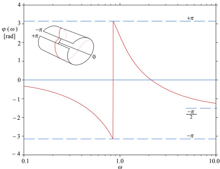
**Fig. 6.4.6:** The phase angle vs. frequency plot of the 5<sup>th</sup>-order Butterworth system. The circularity of trigonometric functions, defined within the range  $\pm\pi$  radians, is the cause of the discontinuous phase vs. frequency relationship.
