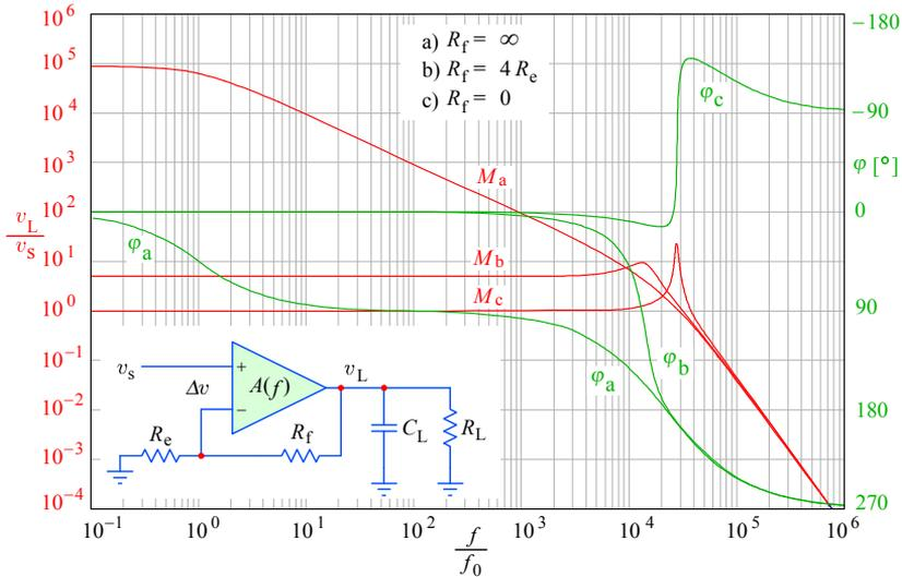
**Fig. 5.3.27:** An amplifier driving a capacitive load can become unstable if its close loop gain is decreased too much: a) with no feedback and b) with a gain of 5, the amplifier is stable, although in the latter case there is already a pronounced peaking; whilst in c) with the closed loop gain reduced to 1 the peaking is very high and the phase goes over  $360^\circ$  and oscillation is excited at the frequency at which the phase equals  $360^\circ$ .
