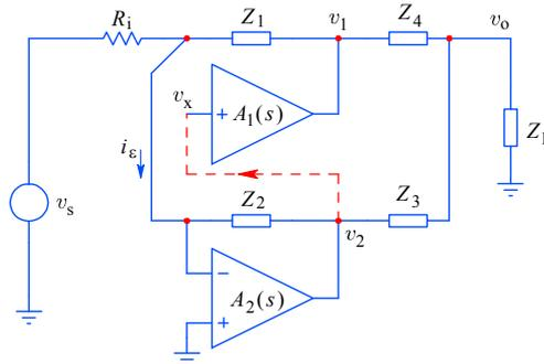
**Fig. 5.4.6:** Current dumping: by taking the main amplifier input signal ( $v_x$ ) from the auxiliary amplifier ( $v_2$ ), we obtain the original Quad 405 amplifier configuration. Although it is effective in error cancellation, its main disadvantages are the requirement for large voltage at the auxiliary amplifier output and a relatively low cut off frequency. In the Quad 405,  $Z_1$  and  $Z_3$  are resistors,  $Z_2$  is a capacitor and  $Z_4$  is an inductor.
