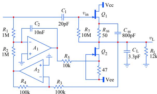
**Fig. 5.2.17:** By inverting the output the error amplifier becomes an inverting integrator and the offset correction is independent from the attenuator settings. The bootstrapping of  $R_7$  produces an effective input resistance of about  $2.4\text{ G}\Omega$ .
