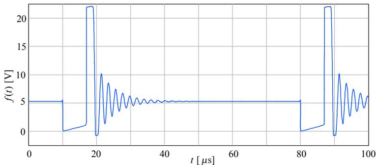
**Fig. 1.2.8:** An example of a periodic waveform (a typical flyback switching power supply), having a finite number of discontinuities within one period. Its frequency spectrum can also be calculated using the Fourier transform, if needed (e.g., to analyze the possibility of electromagnetic interference at various frequencies), in the same way as we did for the square wave.
