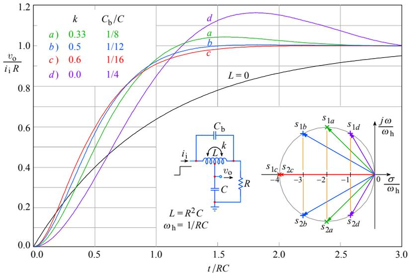
**Fig. 2.4.8:** The step response of the T-coil circuit. As before, **a)** is MFA, **b)** is MFED, **c)** is CD and **d)** is the case  $k = 0$ . The non-peaking case ( $L = 0$ ) is the reference. The no-coupling case has excessive overshoot, 16.3%, but MFA overshoot is also high, 4.3%. Note the pole pattern of the four cases: the closer the poles are to the imaginary axis, the greater is the overshoot. The diameter of the circle on which the poles lie is  $4/RC$ .
