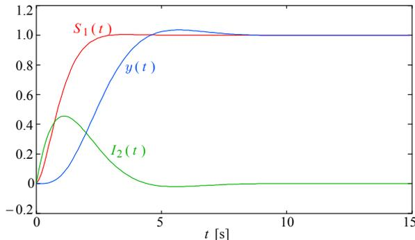
**Fig. 7.1.3:** Convolution example of [Part 1, Sec. 1.15](#). A Bessel–Thomson 2-pole system step response  $S_1(t)$  has been fed to the 2-pole Butterworth system and convolved with its impulse response  $I_2(t)$ , resulting in the output step response  $y(t)$ . Compare it with [Fig. 1.15.1g](#).
