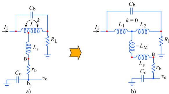
**Fig. 3.6.9:** a) The base lead inductance  $L_s$  decreases the value of mutual inductance, as indicated by the equivalent circuit in b). This can be compensated by recalculating the circuit with an increased coupling factor.
