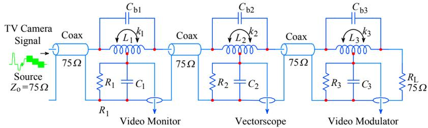
**Fig. 2.4.11:** Input impedance compensation by T-coil sections prevents signal reflections. Each section of the coaxial cable sees the terminating  $75\ \Omega$  resistor at the end of the chain. The bandwidth is affected only slightly. The circuit values are shown in the text above.
