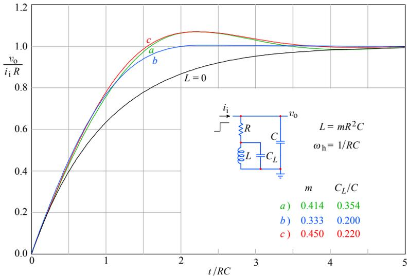
**Fig. 2.8.5:** Three-pole shunt peaking circuit step response: **a)** MFA; **b)** MFED; **c)** SPEC. The non-peaking case ( $L = 0$ ) is the reference. The initial slope is similar to the non-peaking response, since the difference between the number of system poles and zeros is one only.
