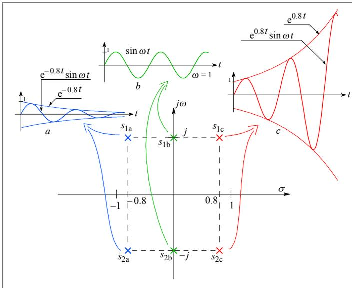
**Fig. 4.3.1:** Impulse response of three different complex conjugate pole pairs: The real part determines the system stability:  $s_{1a}$  and  $s_{2a}$  make the system unconditionally stable, since the negative exponent forces the response to decrease with time;  $s_{1b}$  and  $s_{2b}$  make the system conditionally stable, whilst  $s_{1c}$  and  $s_{2c}$  make it unstable.
