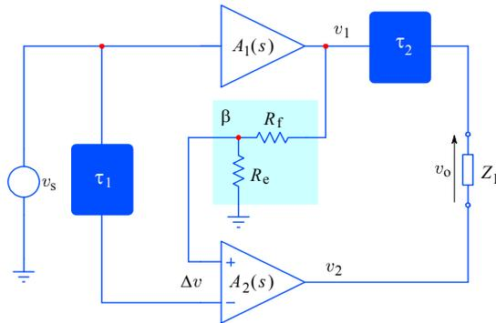
**Fig. 5.4.7:** Time delay compensation principle for the basic feedforward amplifier:  $\tau_1$  compensates the delay introduced by the main amplifier and  $\tau_2$  compensates the delay introduced by the auxiliary amplifier.
