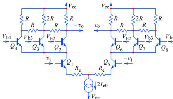
**Fig. 5.4.38:** With an  $R-2R$  network the attenuation can be switched in steps by applying a positive DC voltage  $V_{b2,3,4}$  to  $Q_{2,6}, Q_{3,7}, Q_{4,8}$ , one pair at a time; at each collector the load is  $R \parallel 2R = 2R/3$ . With  $Q_{2,6}$  on the gain is  $A = 2R/3R_e$ , with  $Q_{3,7}$  on  $A = R/3R_e$ , and with  $Q_{4,8}$  on  $A = R/6R_e$ , effectively halved by each step. A similar circuit was used in the Tek 2465.
