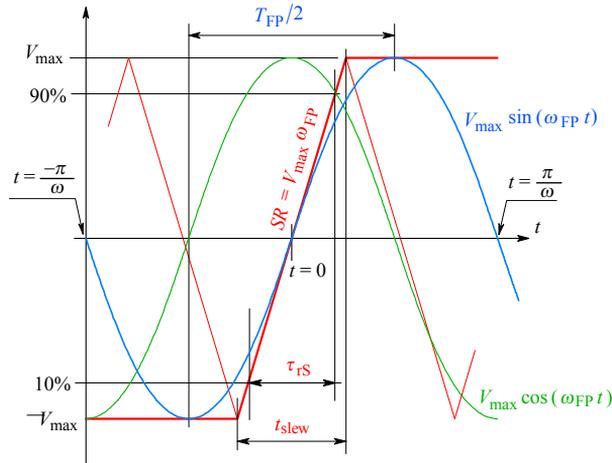
**Fig. 4.1.8:** Slew rate limiting: definitions of parameters.
