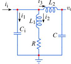
Fig. 2.9.1: The shunt–series peaking circuit.
