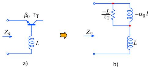
**Fig. 3.2.6:** The inductive source is reflected into the emitter with **negative** components.
