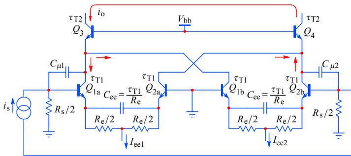
**Fig. 3.8.2:** The basic  $f_T$  doubler circuit. We assume equal transistors for  $Q_{1a,2a}$  and  $Q_{1b,2b}$ . The low input impedance of  $Q_{3,4}$  emitters allows summing the collector current of each pair, but cross-coupled for in phase signal summing.
