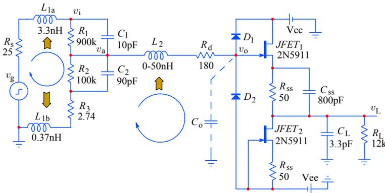
**Fig. 5.2.9:** The attenuator and the source follower JFET<sub>1</sub> (JFET<sub>2</sub> acts as a constant current source bias for JFET<sub>1</sub>). The input loop inductance  $L_1$  should be low, but the attenuation can be compensated by  $L_{1b}$ . The inductance  $L_2$  of the second loop can be ‘tuned’ and damped by an appropriate value of  $R_d$  to provide a Bessel step response, as seen in Fig. 5.2.10.
