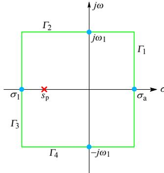
**Fig. 1.13.6:** By using a rectangular contour as shown it is possible to prove the inverse Laplace transform by means of the contour integral, even if the number of poles exceeds the number of zeros by only one. In this integral, encircling the single simple pole, we let  $\sigma_1 \rightarrow \infty$  and  $\omega_1 \rightarrow \infty$ , so that the integrals along  $\Gamma_2$ ,  $\Gamma_3$  and  $\Gamma_4$  vanish.
