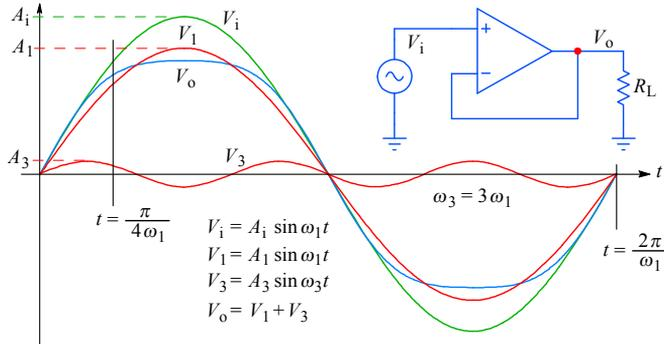
**Fig. 1.1.2:** The amplifier is slightly overdriven by a pure sinusoidal signal,  $V_i$ , with a frequency  $\omega_1$  and amplitude  $A_i$ . The output signal  $V_o$  is distorted, and it can be represented as a sum of two signals,  $V_1 + V_3$ . The fundamental frequency of  $V_1$  is  $\omega_1$  and its amplitude  $A_1$  is somewhat lower. The frequency of  $V_3$  (the third harmonic component) is  $\omega_3 = 3\omega_1$  and its amplitude is  $A_3$ .
