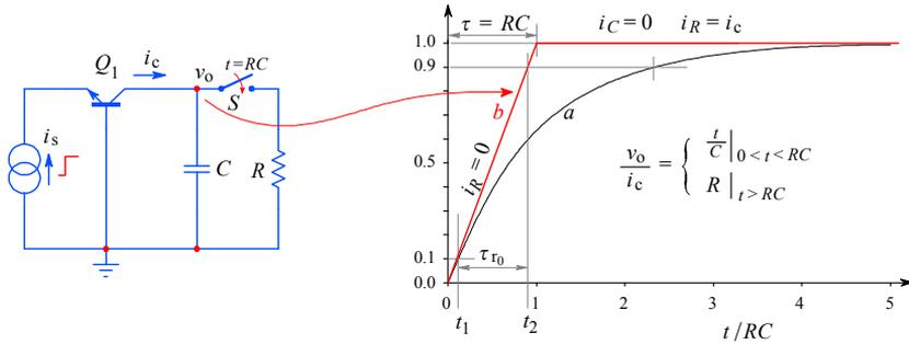
**Fig. 2.1.2:** A hypothetical ideal rise time circuit. The switch disconnects  $R$  from the circuit, so that all of  $i_c$  is available to charge  $C$ ; but after a time  $t = RC$  the switch is closed and all  $i_c$  flows through  $R$ . The resulting output voltage is shown in *b*, compared with the exponential response in *a*.
