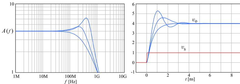
**Fig. 5.3.21:** a) Frequency response; b) Step response of the amplifier in Fig. 5.3.20. The closed loop gain  $A_{cl} = 1 + R_f/R_e = 4$ ,  $R_f = 150 \Omega$ ,  $R_e = 50 \Omega$ , the source resistance  $R_s = 50 \Omega$ , the stray capacitances,  $C_{s1,2} = 1$  pF, the amplifier transcapacitance  $C_T = 1$  pF, while  $R_b$  is varied from  $150 \Omega$  for highest peaking to  $750 \Omega$  for lowest peaking.
