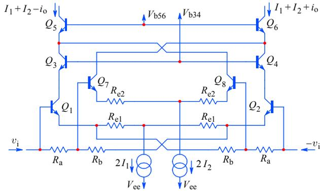
**Fig. 5.4.26:** Another evolution of the Cascomp is realized by feedback derived error sensing and feedforward error correction. The junction of  $R_a$  and  $R_b$  is at the ‘virtual ground’ at which the error of the  $Q_{1,2}$  pair is sensed and amplified by the auxiliary amplifier  $Q_{7,8}$ . The error is subtracted from the output current at the emitters of  $Q_{5,6}$ .
