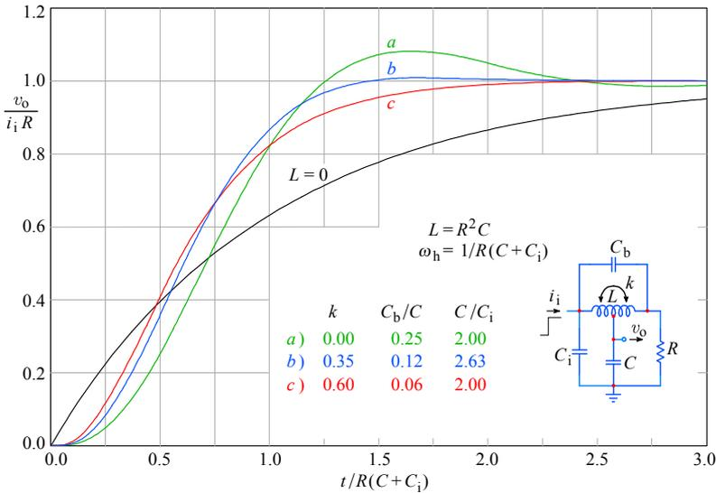
**Fig. 2.5.7:** The step response of the three-pole T-coil circuit: **a)** MFA; **b)** MFED; **c)** CD. The non-peaking case ( $L = 0$ ) is the reference. Since the total capacitance  $C + C_i$  is equal to  $C$  of the two-pole T-coil circuit, the MFED rise time is also nearly identical. However, the three-pole circuit is much easier to realize in practice, owing to the lower  $k$  required.
