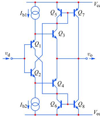
Fig. 5.3.25: Output buffer stage with improved current handling.
