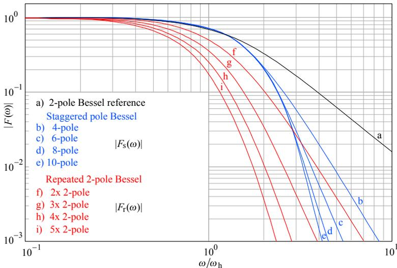
**Fig. 4.6.1:** Frequency response magnitude of systems with staggered poles, compared with systems with repeated second-order pole pairs. By using staggered poles the bandwidth is preserved, whilst for systems with repeated poles it decreases with each additional stage.
