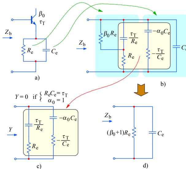
**Fig. 3.2.8:** Transformation of the emitter  $RC$  network as seen from the base: a) schematic; b) equivalent circuit; c) if  $RC = \tau_T$  and  $\alpha_0 = 1$ , the sum of the middle frame component's admittances is zero; d) final equivalent circuit.
