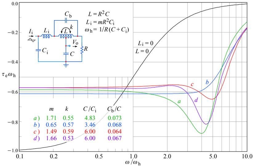
**Fig. 2.6.6:** Four-pole L+T peaking circuit envelope delay: **a)** MFA; **b)** MFED; **c)** Group C; **d)** Group A. For the non-peaking case at DC, the envelope delay is 1; all other cases have a larger bandwidth and consequently a lower delay. Note the MFED flatness up to nearly  $3.3 \omega_h$ .
