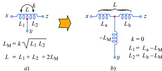
**Fig. 2.4.2:** Modeling the coupling factor: **a)** The T-coil coupling factor  $k$  between the two halves  $L_1$  and  $L_2$  of the total inductance  $L$  can be represented by **b)** an equivalent circuit, having two separate (non-coupled) inductances, in which the magnetic coupling is modeled by the mutual inductance  $L_M$  (negative in value), so that  $L_1 = L_a - L_M$  and  $L_2 = L_b - L_M$ .
