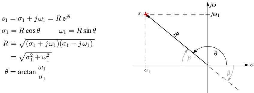
**Fig. 1.13.4:** Cartesian and polar representations of a complex number (note:  $\tan \theta$  is equal for the counterclockwise defined  $\theta$  from the positive real axis and for the clockwise defined  $\beta = \theta - \pi$ ).
