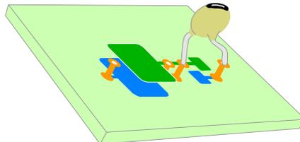
**Fig. 5.2.12:** Canceling the hook-effect in the common PCB material is achieved by intentionally adding two capacitances in form of large PCB pads, with areas in the same ratio as required by the attenuation (since the area is proportional to the square of the linear dimensions, for a 9:1 capacitance ratio, a 3:1 dimension ratio is needed). Trimming is possible by drilling small holes in the larger pad.
