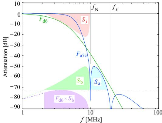
**Fig. 7.2.18:** The spectrum  $S_a$  is aliased into  $S_b$ . The difference between the ADC resolution and  $S_b$  (both in dB) gives  $S_r$ , the envelope of which determines the minimum attenuation required by  $F_{d6}$  to suppress  $S_b$  below the ADC resolution.
