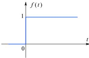
Fig. 1.5.1: Unit step function.
