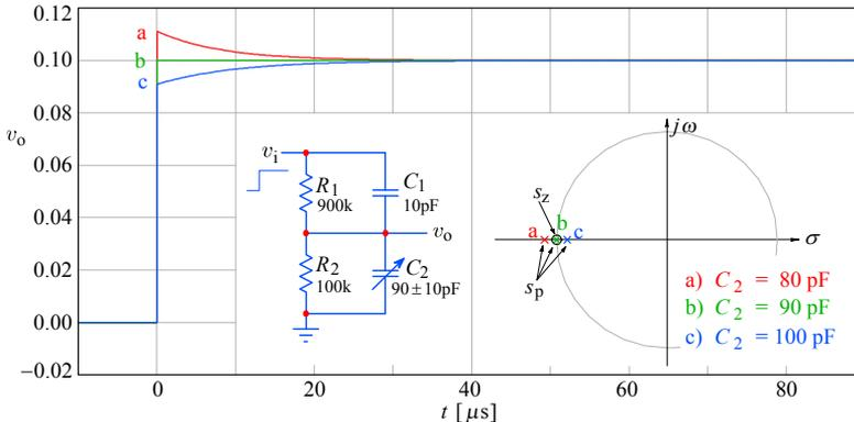
**Fig. 5.2.4:** The attenuator's step response for the correctly compensated case, along with the under- and over-compensated cases ( $C_2$  is trimmed by  $\pm 10$  pF). Note that by changing  $C_2$  the system pole also changes but the system zero remains the same.
