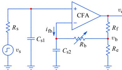
**Fig. 5.3.20:** This circuit exploits the ability of current feedback amplifiers to adjust the bandwidth and gain peaking independently of the gain. The price to pay is the lower slew rate limit. See the frequency and the step response below.
