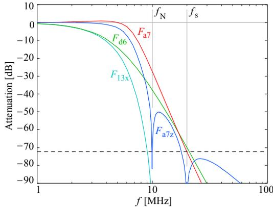
**Fig. 7.2.17:** By adding the zeros the analog filter frequency response is modified from  $F_{a7}$  to  $F_{a7z}$ .  $F_{d6}$  is the digital filter response and  $F_{13x}$  is the composite mixed mode response.
