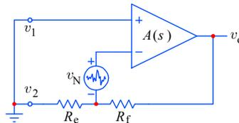
**Fig. 5.3.14:** Noise gain definition: A noisy amplifier is modeled as a noise generator  $v_N$  in series with the input of a noiseless amplifier. The inverting signal gain is  $v_o/v_2 = -R_f/R_e$ ; the non-inverting signal gain is  $v_o/v_1 = 1 + R_f/R_e$ ; the noise gain is  $v_o/v_N = -(1 + R_f/R_e)$ . The noise generator polarity is indicated only as a reference for the noise gain polarity inversion.
