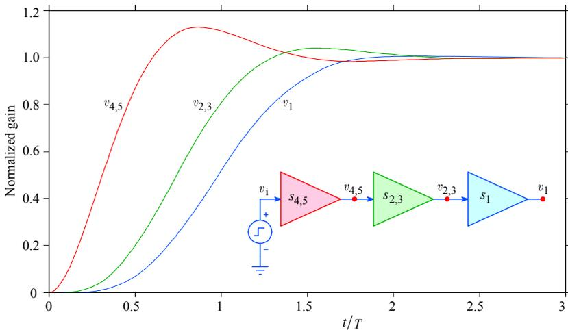
**Fig. 4.6.4:** Step response of the complete amplifier with reverse pole order at each stage. Although the second stage had no overshoot of its own, it overshoots by nearly 5% when processing the  $v_{4,5}$  output.
