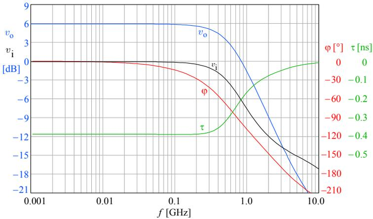
**Fig. 5.4.15:** Frequency domain performance of the differential cascode amplifier using the circuit of Fig. 5.4.14b. The bandwidth is about 560 MHz. Note the input voltage changing slope above 2 GHz.
