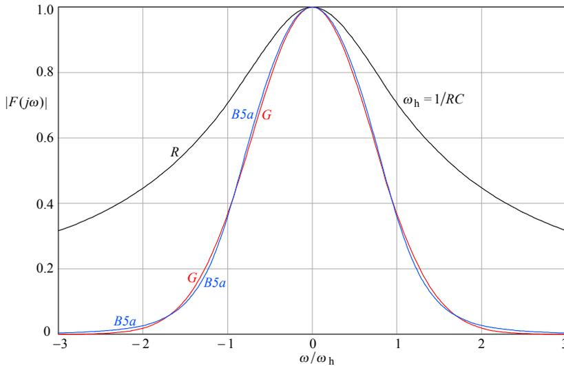
**Fig. 4.4.7:** Ideal Gaussian (MFED) frequency response  $G$  (real only, with no phase shift), compared to the magnitude of a 5<sup>th</sup>-order modified Bessel system  $B5a$  (identical cutoff asymptote, [Table 4.5.1](#)). The frequency scale is two-sided, linear, and normalized to  $\omega_h = 1/RC$  of the first-order system, which is shown as the reference  $R$ .
