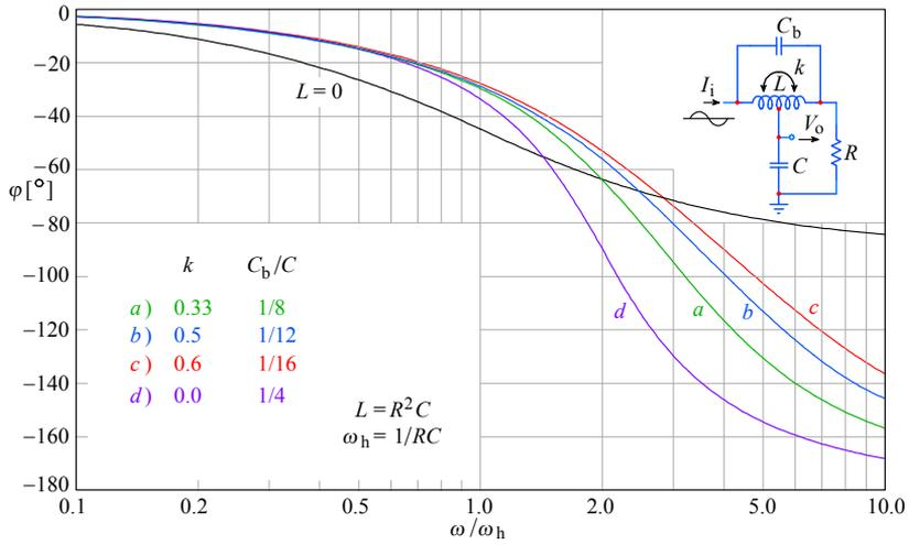
**Fig. 2.4.6:** The transfer function phase angle of the T-coil circuit, for the same values of coupling and capacitance ratio as for the frequency response magnitude. *a)* is MFA, *b)* is MFED, *c)* is CD and *d)* is the no-coupling case. The non-peaking ( $L = 0$ ) case is the reference.
