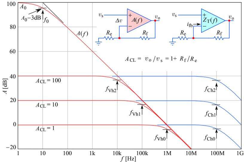
**Fig. 5.3.10:** Comparison of closed loop cut off frequency vs. gain of a conventional and a current feedback amplifier. The conventional amplifier has a constant GBW product (higher gain, lower cut off). But the current feedback cut off frequency is (almost) independent of gain.
