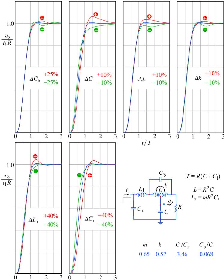
**Fig. 2.11.1:** Four-pole L+T peaking circuit step response sensitivity on component tolerances. Such graphs were drawn originally by *Carl Battjes* for a class lecture at Tektronix, but with another set of parameters as the reference. The responses presented here were obtained using the MicroCAP-5 circuit analysis program. [Ref.2.36].
