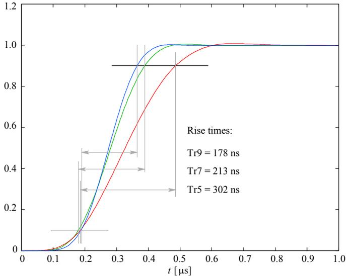
**Fig. 7.2.8:** Step responses of the 5-, 7-, and 9-pole Bessel–Thomson systems, having equal attenuation at the Nyquist frequency. The rise times are calculated from the number of samples between the 10% and 90% of the final value of the normalized amplitude.
