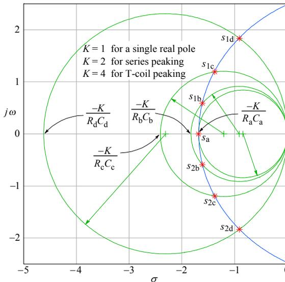
**Fig. 5.1.2:** The 7 normalized Bessel–Thomson poles. The characteristic circle of each pole (pair) has a diameter determined by the appropriate  $RC$  constant and the peaking factor  $K$ , which depends on the type of network chosen.
