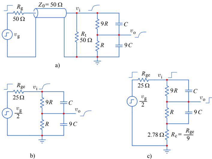
**Fig. 5.2.5:** **a)** When working with  $50 \Omega$  impedance the terminating resistance must match the generator internal resistance, forming a  $\div 2$  attenuator with an effective output impedance of  $25 \Omega$ ; **b)** With a  $9 \text{ pF}$  attenuator input capacitance, a HF cut off at  $707 \text{ MHz}$  results; **c)** The cut off for the  $\div 10$  attenuator can be compensated by a  $25/9 \Omega$  resistor between the lower end of the attenuator and the ground.
