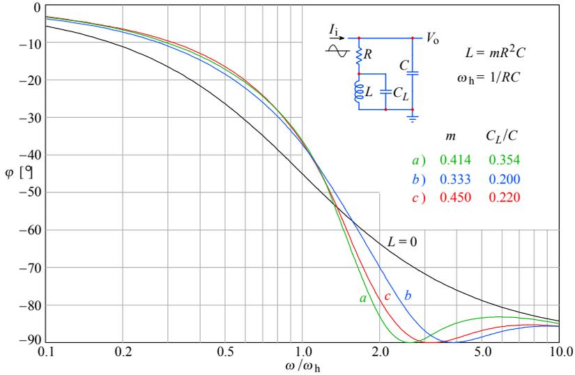
**Fig. 2.8.3:** Three-pole shunt peaking circuit phase response: *a)* MFA; *b)* MFED; *c)* SPEC. The non-peaking case ( $L = 0$ ) is the reference. The system zeros cause the phase response bouncing up at the  $-90^\circ$  boundary and then returning back.
