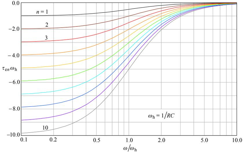
**Fig. 4.1.5:** Envelope delay of the amplifier in Fig. 4.1.1, for  $n = 1-10$  amplifying stages. The delay at  $\omega = \omega_h$  is 1/2 of the low frequency asymptotic value. Note that if we were using  $f/f_h$  for the abscissa, we would have to divide the  $\tau_e$  scale by  $2\pi$ .
