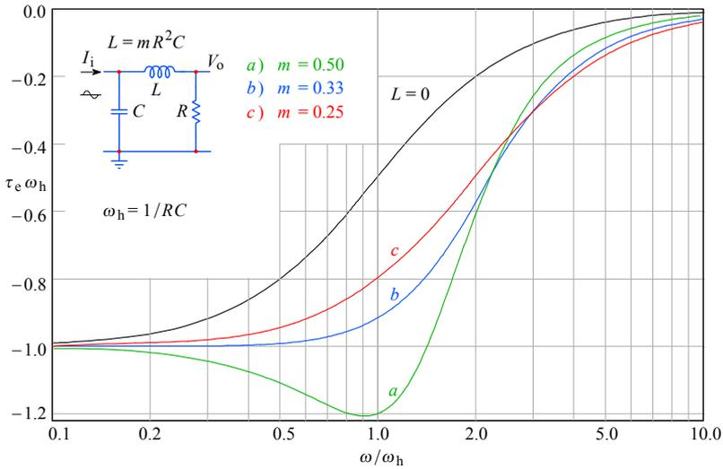
**Fig. 2.2.7:** Envelope delay of the series peaking circuit for the same characteristic values of  $m$  as before: *a)* MFA, *b)* MFED, *c)* CD. Note the MFED plot being flat up to nearly  $0.5 \omega_h$ .
