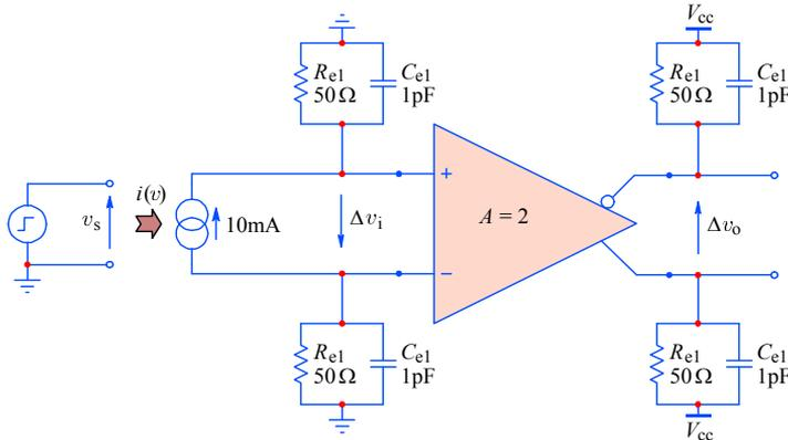
Fig. 5.4.10: Test set up used to compare different amplifier configurations.
