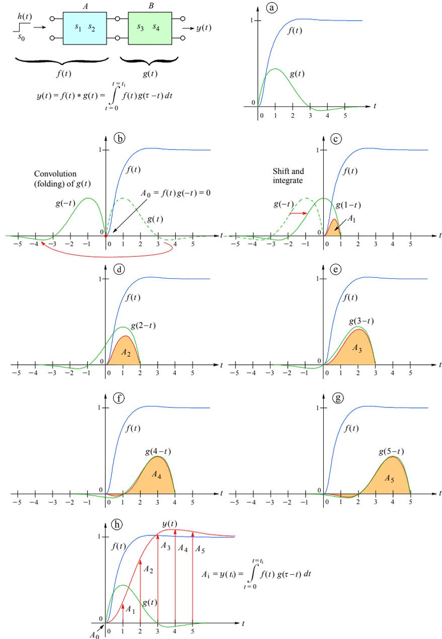
**Fig. 1.15.1:** Graphic presentation of the mathematical course of the convolution integral,  $f(t)*g(t)$ . See the text for the description. To see the movie click on this link: [convmovie.gif](#) (we apologize for the bad quality resulting from the poor conversion from vector graphics to bitmap format; readers who have access to Matlab are invited to run the 'convmovie.m' file).
