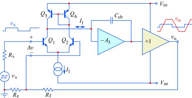
**Fig. 5.3.3:** Simplified conventional opamp circuit with the current mirror as the active load to  $Q_1$ . The second stage is modeled as a Miller integrator with large gain. This circuit exhibits symmetrical slew rate limiting. The dominant pole  $s_0 = -g_m/C_M$ , where  $g_m$  is the differential amplifier's transconductance and  $C_M = C_{cb}(1 + A_3)$ .
