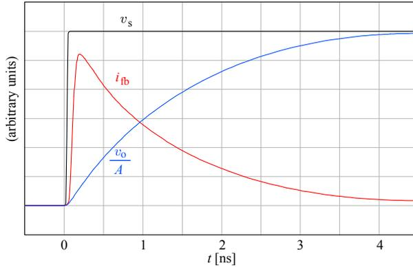
**Fig. 5.3.9:** ‘Current on demand’: The step response reveals that the feedback current is proportional to the difference between the input and output voltage, essentially a high pass version of the output voltage, as shown by [Eq. 5.3.27](#).
