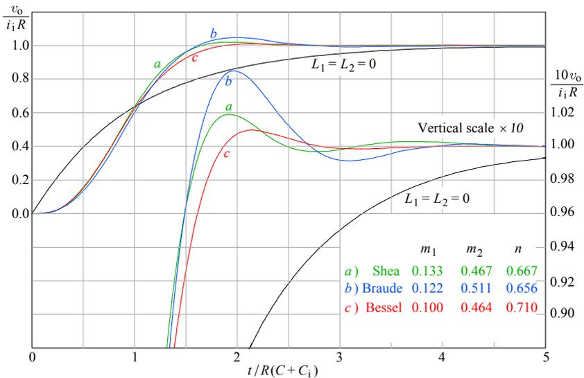
Fig. 2.9.6: The MFED shunt-series peaking circuit step response: a) by Shea; b) by Braude; c) a true Bessel system. The  $\times 10$  vertical scale expansion shows the top 10% of the response. The overshoot in the Braude case is excessive, whilst the Shea version has a prolonged ringing. Although slowest, the Bessel system is the first to settle to  $< 0.1\%$  of the final value.
