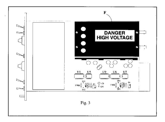
3. If the polarity must be changed, remove the four screws and the cover. The two multipliers enclosed in silicon black rubber will appear, channel A on the top, and a large diode bridge with a white dot at one side ( see fig. 4 ) will be available in the middle of each multiplier section. A positive channel has the white dot on the diode bridge towards the output connector.
