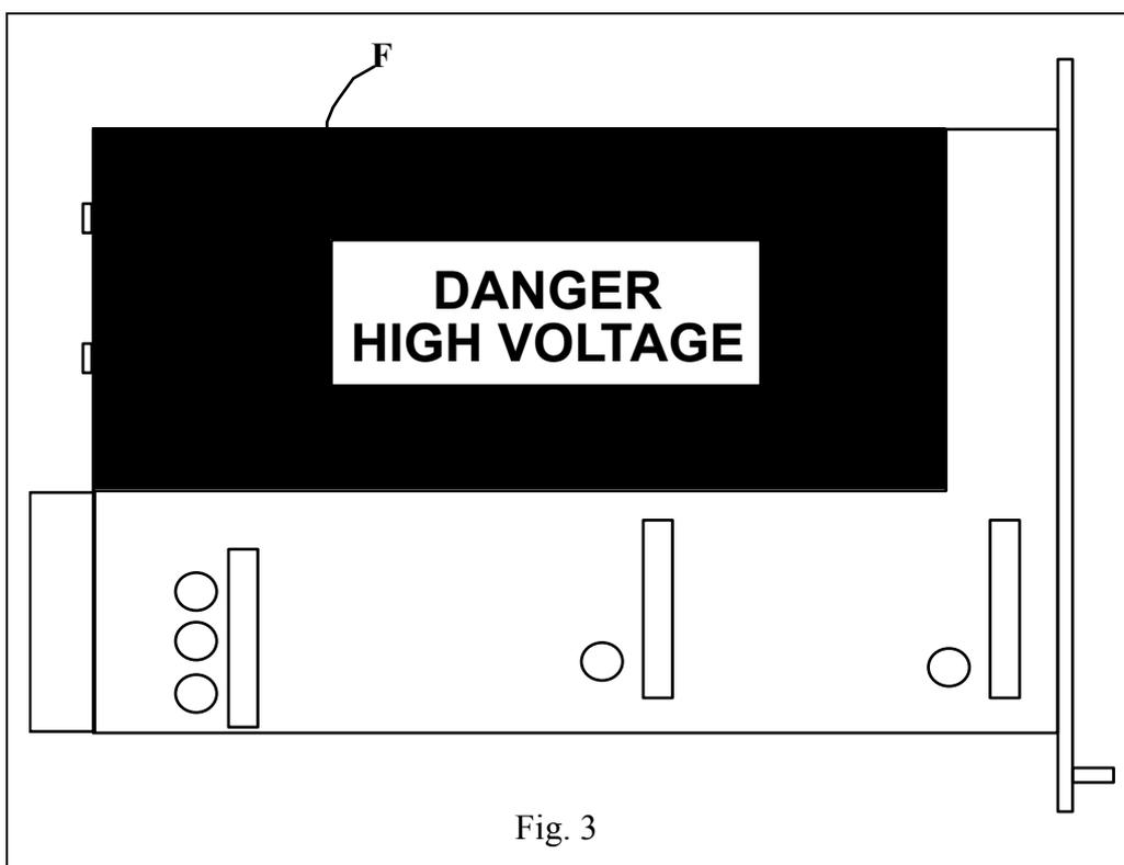
A large module (labelled F in the figure) appears on the Board. This is the High-Voltage block housing the two multipliers of the channels and bears a "High-Voltage Danger" sign. The cover is fixed to the base through several screws; remove them and the cover.
