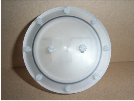
**Figure 31:** Top view of the plexiglas source with TUM logo inside. The logo gets filled with activity, the cap can be taken off. The two screws in the middle of the cap are for filling and de-aeration.
