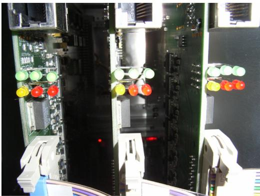
**Figure 37:** LEDs at the SADCs, in loaded state.
