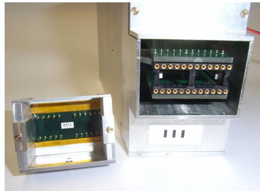
**Figure 26:** Connection of the APDs to the detector module and the preamplifiers.
