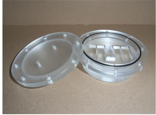
**Figure 32:** View of a source with removed cap. The o-ring between cap and base seals the source.
