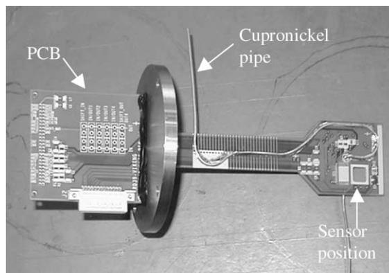
Fig. 2. Picture of a cryogenic module: a thin cupronickel pipe is soldered on the PCB. A flow of cold nitrogen gas in the pipe cools down the module.
