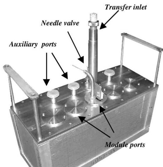
Fig. 1. The low-mass cryostat has several access ports. Five ports are to insert the cryogenic modules, one port is for the inlet of the LN<sub>2</sub> transfer line, and three additional ports are for instrumentation connections. A needle valve allows the liquid to refill the box.
