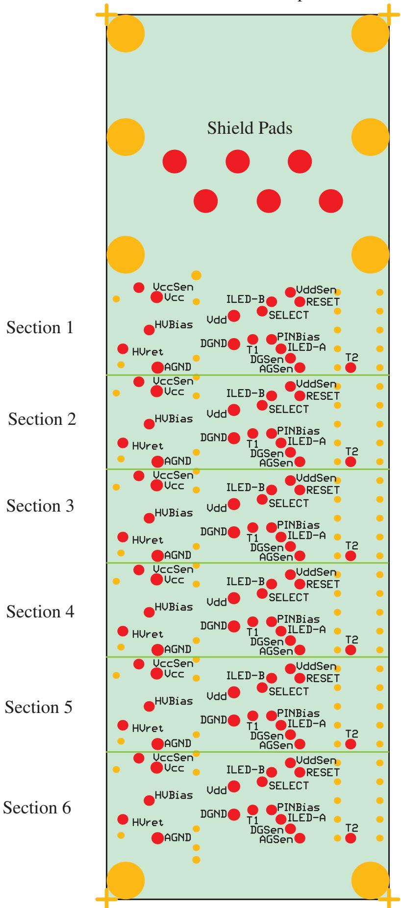
The pad names are silk-screen printed on the PCB.
