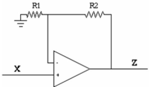
$$\frac{0 - \eta}{R_1} + \frac{z - \eta}{R_2} + I_{bias} = 0$$
