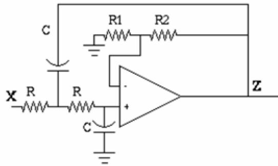
$$T(\hat{p}) = \frac{\alpha}{1 + \varphi(3 - \alpha) + \tau^2 p^2}, \quad \alpha = 1 + \frac{R_2}{R_1}$$
