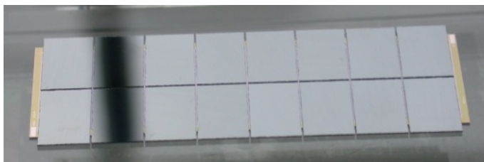
poly-CVD (16 chip ATLAS pixel module)
