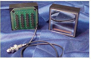
technique with an alternate voltage divider network. The dual MCP multiplier provides excellent time response, good gain, and extremely high pulse linearity. Response uniformity over the full 2" square active area is exceptional, typically 1:1.5. The assembly comes with terminated anode and high voltage cables for ease of use. Applications include specialized medical imaging, ring imaging Cherenkov counters, fluorescence microscopy, and high-speed applications such as LIDAR.
