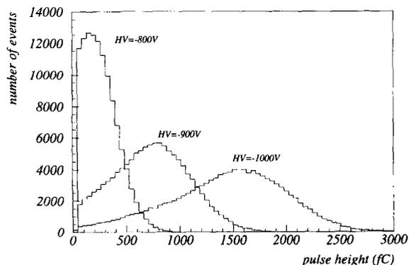
Fig. 4. Pulse height distributions for single photoelectrons ejected from the photocathode of the H-6568 photomultiplier.
