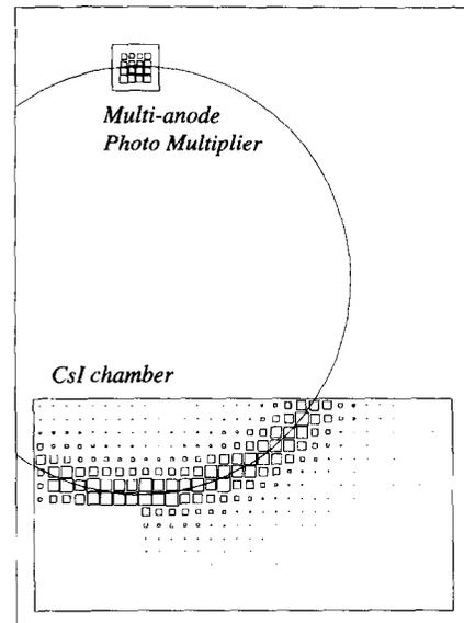
Fig. 3. The distribution of hits for Cherenkov rings intercepted by the CsI-MWPC and the multi-anode PMT.
