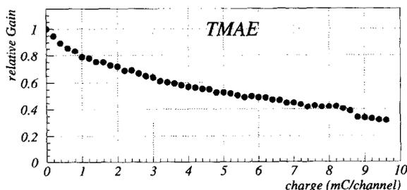
Fig. 2. Ageing of the TMAE detector. The dependence of the anode wire relative gain on the charge collected per channel.
