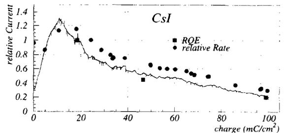
Fig. 1. Ageing of the CsI-MWPC detector. The dependence of the normalized current  $I/I_0$  (full line), of the normalized rate (full circles) and the relative quantum efficiency (full squares) on the accumulated charge per  $\text{cm}^2$  of the CsI-MWPC detector.
