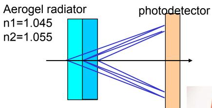
Multi-pixel photodetector to measure single photon positions in B=1.5T → HAPD/MCP-PMT/G-APD
