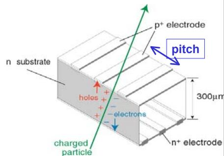
Two coordinates measured at the same time; strip pitch: 50 μm (75 μm); resolution about 15 μm (20 μm).
