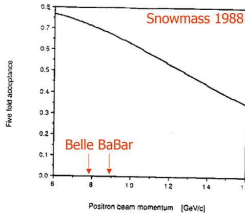
Figure 4. The acceptance of a detector covering  $|\cos \theta_{lab}| < 0.95$  for five uncorrelated particles as a function of the energy of the more energetic beam in an asymmetric collider at the T(4S).
