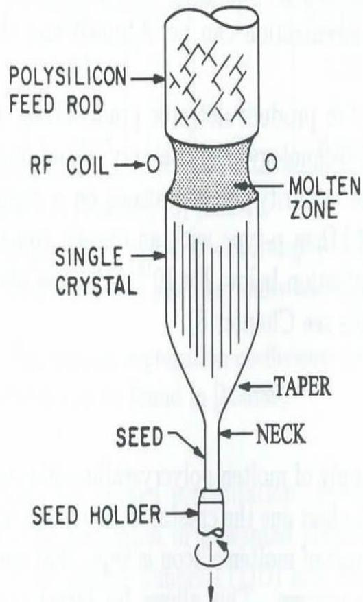
No contact of the liquid semiconductor with the walls – higher purity of the material.
