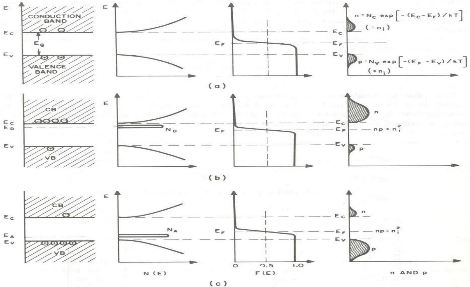
**Fig. 14** Schematic band diagram, density of states, Fermi-Dirac distribution, and the carrier concentrations for (a) intrinsic, (b) n-type, and (c) p-type semiconductors at thermal equilibrium. Note that  $pn = n_i^2$  for all three cases.
