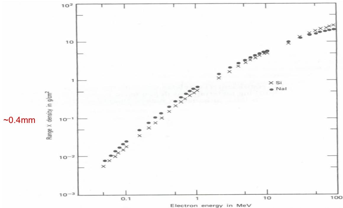
Figure 2.14 Range–energy plots for electrons in silicon and sodium iodide. If units of material thickness (distance  $\times$  density) are used for the range as shown, values at the same electron energy are similar even for materials with widely different physical properties or atom number. (Data from Mukoyama.<sup>24</sup>)
