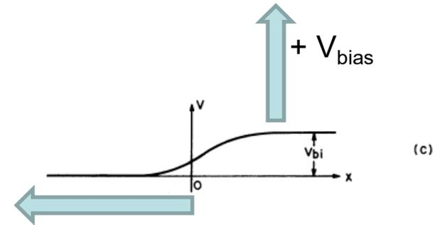
The height of the potential barrier:  $V_B = V_{bias} + V_{bi}$
