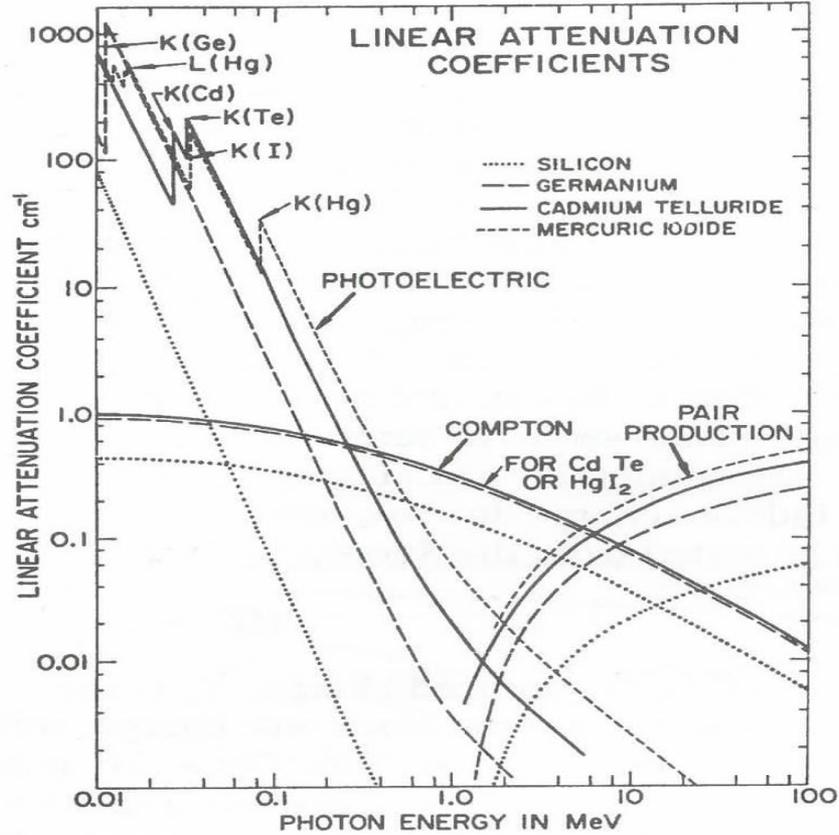
**Figure 13.22** Photoelectric, Compton, and pair production linear attenuation coefficients for Si, Ge, CdTe, and HgI<sub>2</sub>. K-shell absorption edges are shown. (From Malm.<sup>46</sup>)
