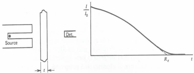
Figure 2.13 Transmission curve for monoenergetic electrons.  $R_e$  is the extrapolated range.
