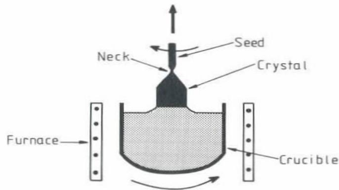
**Figure 3.4** A schematic illustration of the basic features of a Czochralski crystal growth process.
