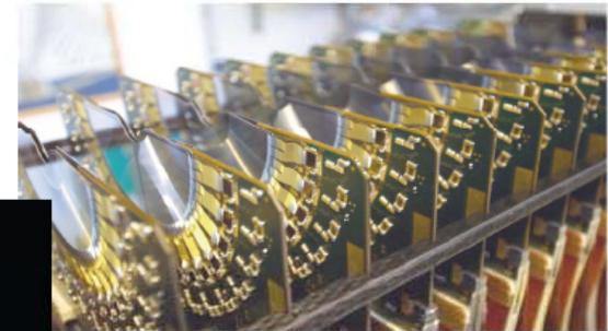
21 stations of Si wafer pairs with  $r$  and  $\phi$  strip readout
