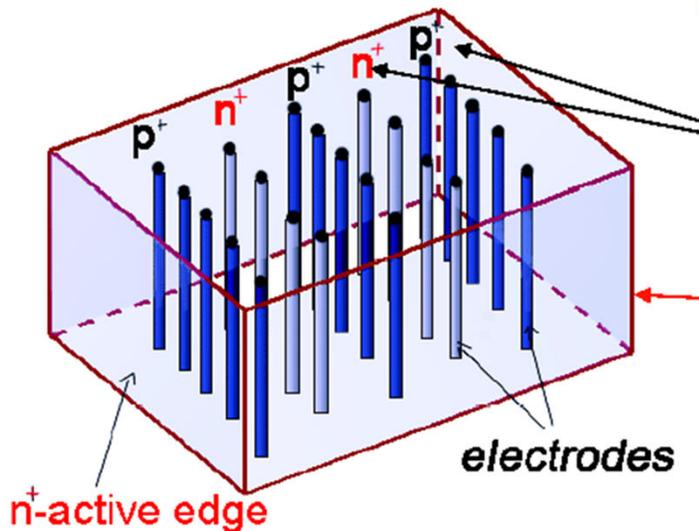
Both electrode types are processed inside the detector bulk instead of being implanted on the wafer's surface.
