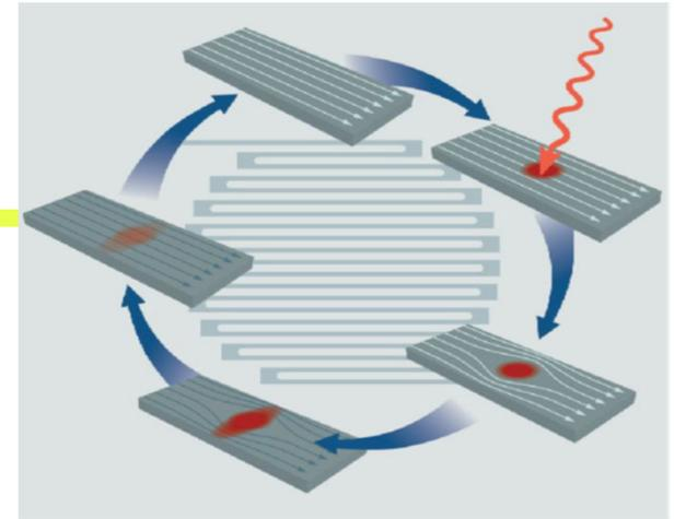
Example: superconducting nano-wire single photon detector (SNSPD): a thin (4 nm) and narrow (100-250 nm) superconducting nanostrip that is current-biased just below its critical current.
