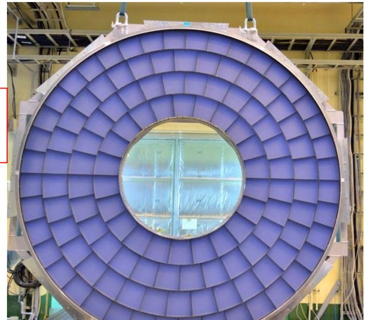
Radiator plane covered with 2 x 124 High Energy tiles water-jet cut tiles (~ 17x17cm)
