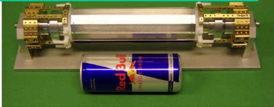
Prototype DEPFET pixel sensor and readout
