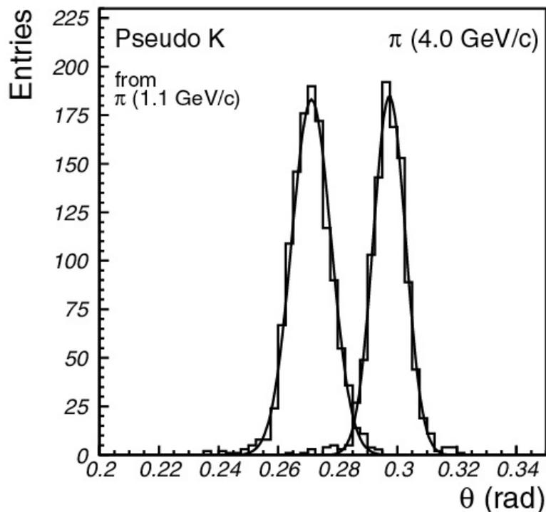
From typical values (single photon resolution 13mrad and 6 detected photons) we can estimate the Cherenkov resolution per track: 5.3mrad;
