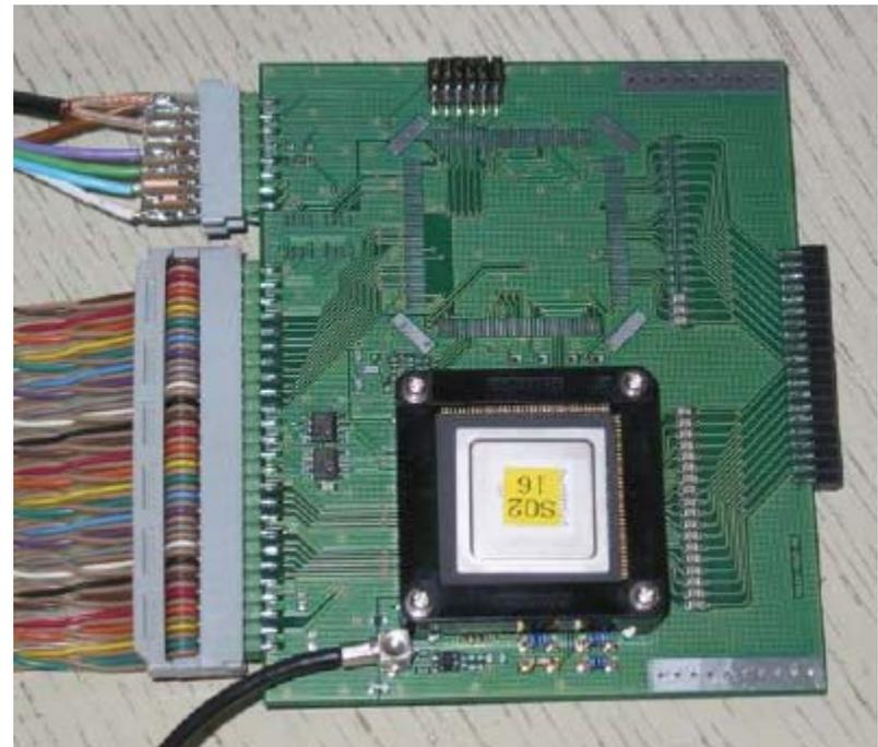
Backup options use chips from Ideas: a VA/TA based system developed by the K2K group at KEK and VA64TAP+LS64
