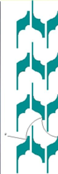
Multianode PMTs (MaPMTs) with metal foil dynodes and 2x2, 4x4 or 8x8 anodes Hamamatsu R5900 (and follow up types 7600, 8500)
