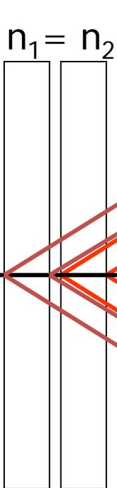
→ stack two tiles with different refractive indices: “focusing” configuration
