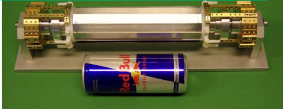
Prototype DEPFET pixel sensor and readout
