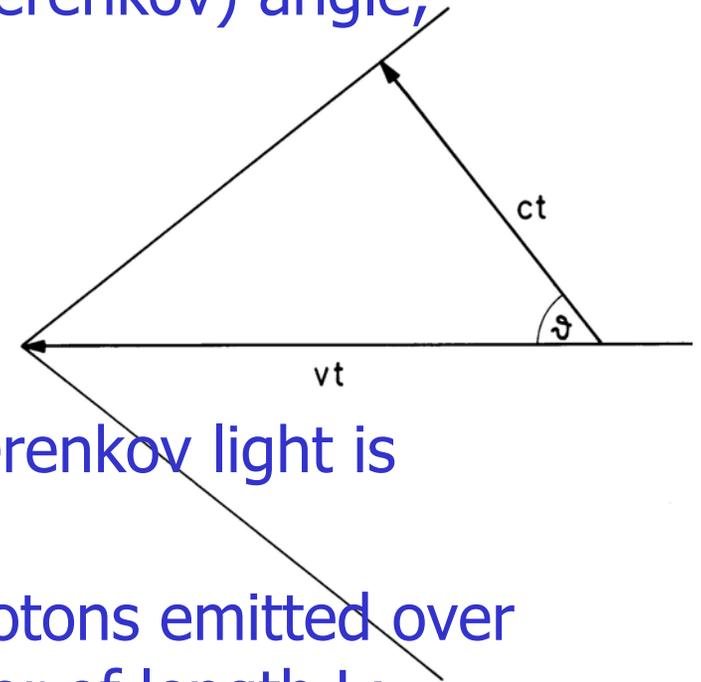
$$\frac{dN}{dE} = n_e L \frac{d\sigma}{dE} = n_e L \frac{\alpha}{\hbar c} \sin^2 \theta = 370(\text{cm})^{-1} (\text{eV})^{-1}$$
