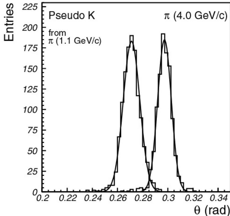
From typical values (single photon resolution 15mrad and 6 detected photons) we can estimate the Cherenkov resolution per track: 5.3mrad;
