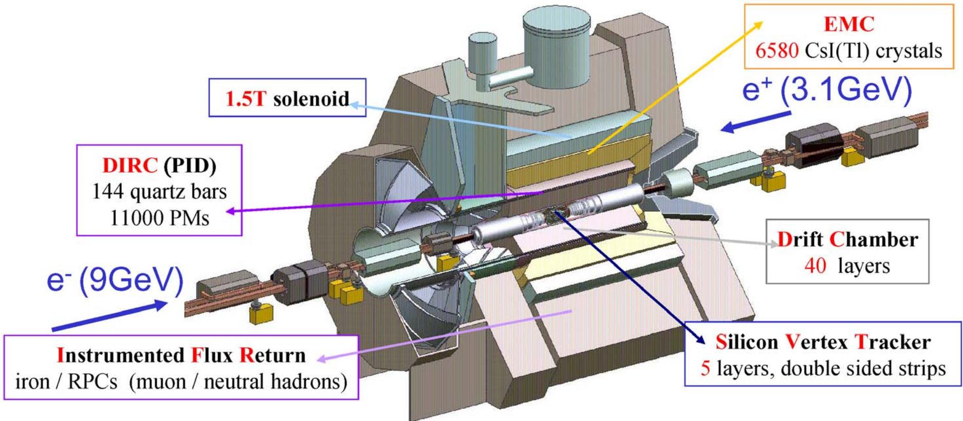
**DIRC - detector of internally reflected Cherenkov light**
