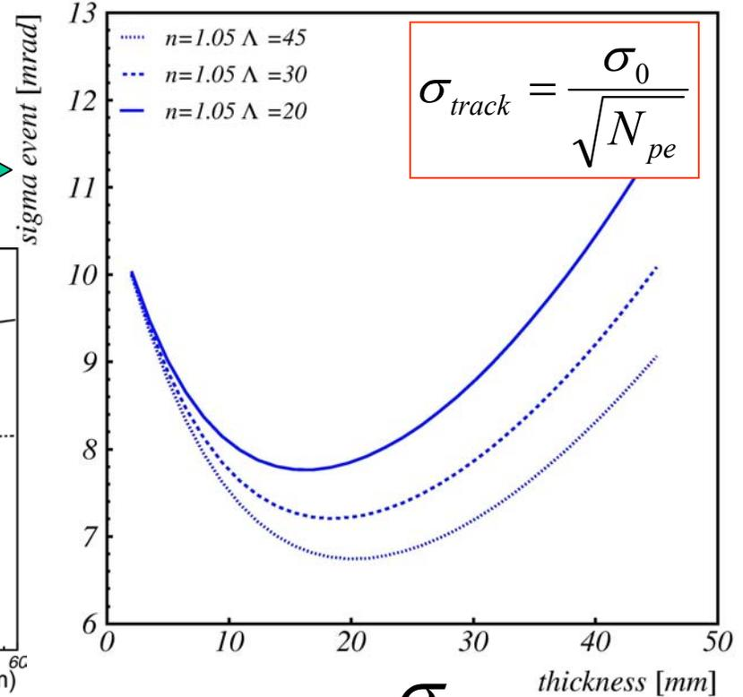
Minimize the error per track:  $\sigma_{track} = \frac{\sigma_0}{\sqrt{N_{pe}}}$
