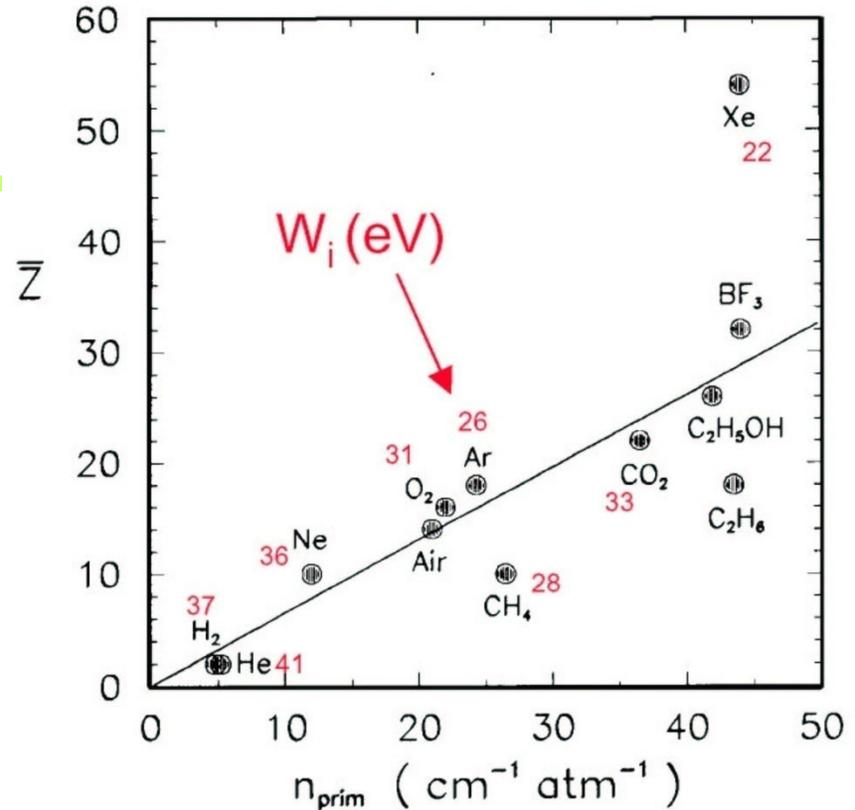
Can this be detected? 120 e-ion pairs make a pulse of  $V = ne/C = 2\text{mV}$  (at typical  $C = 10\text{pF}$ ) → NO
