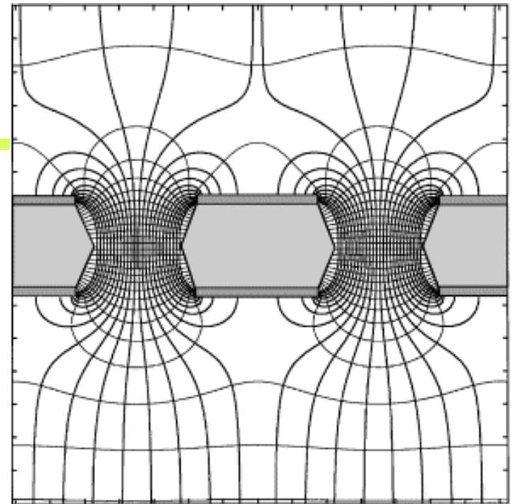
The E field in the holes is non-uniform – large enough to get gas amplification of about 100.
