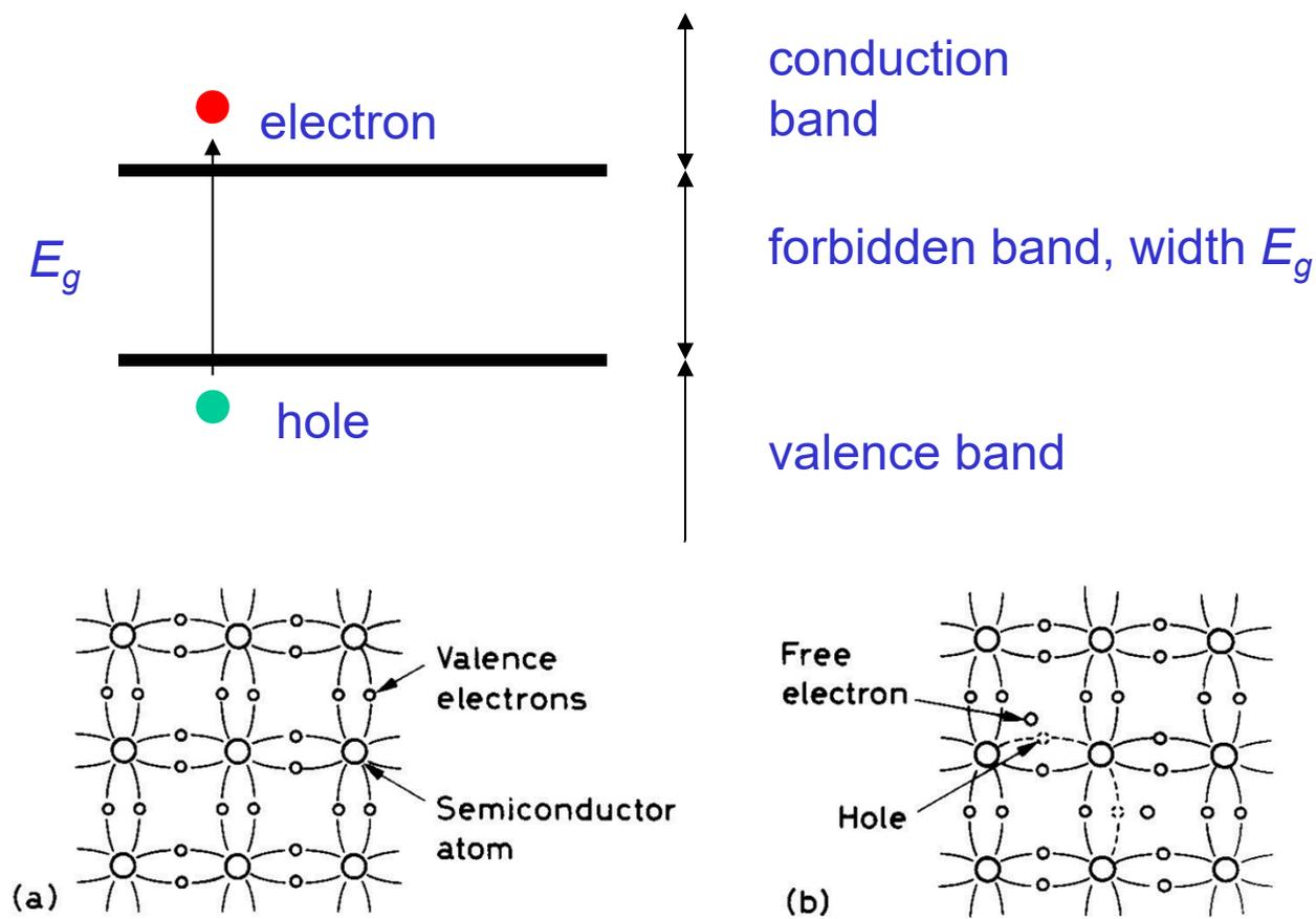
**Fig. 10.2.** Covalent bonding of silicon: (a) at 0 K, all electrons participate in bonding, (b) at higher temperatures some bonds are broken by thermal energy leaving a *hole* in the valence band
