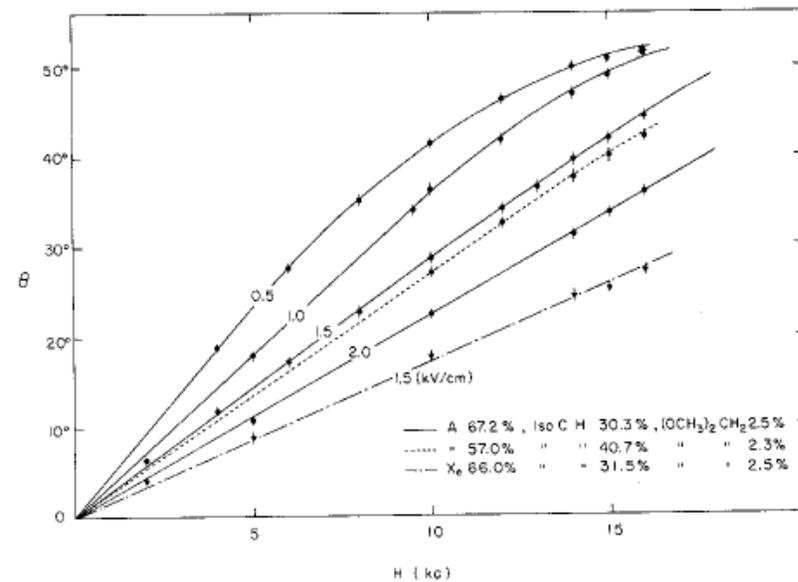
Fig. 38 Measured drift angle (angle between the electric field and the drift directions) as a function of electric and magnetic field strength<sup>9</sup>.
