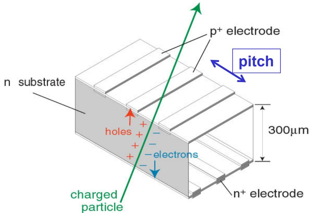
Subdivide electrodes into strips, read out each of the strips, record hit yes/no (digital) or charge (analog).
