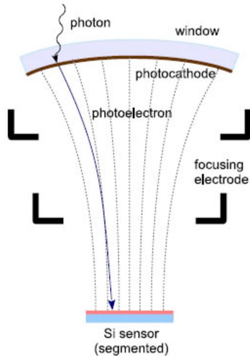
Instead of secondary multiplication: accelerate photoelectrons over a large voltage difference ( $\sim 10kV$ ), and let them hit a Si sensor.
