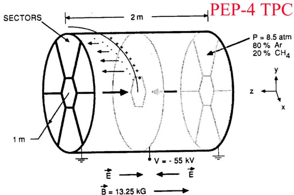
Diffusion: no problem for the transverse coordinate in spite of the very long drift distance because B parallel to E (drift direction).
