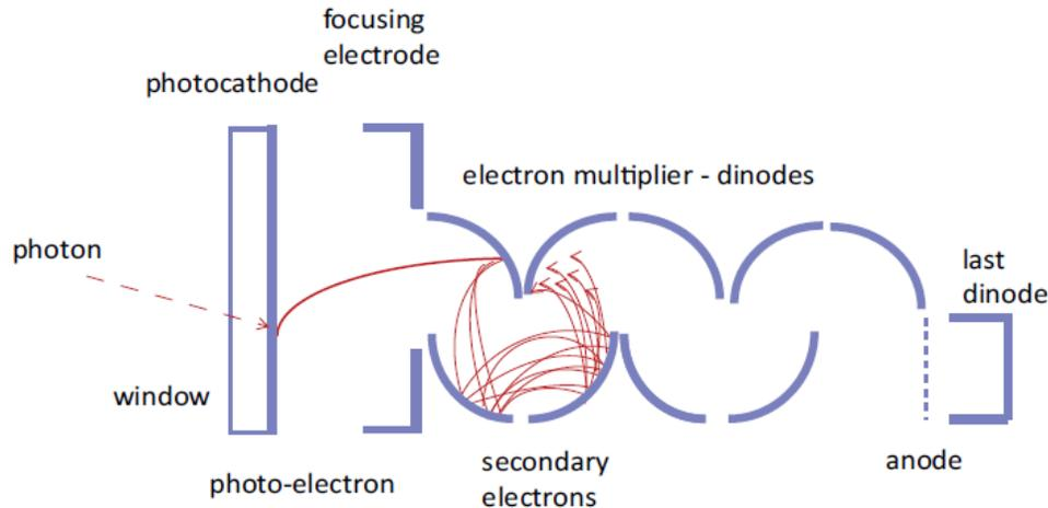
Transform light into an electric signal
