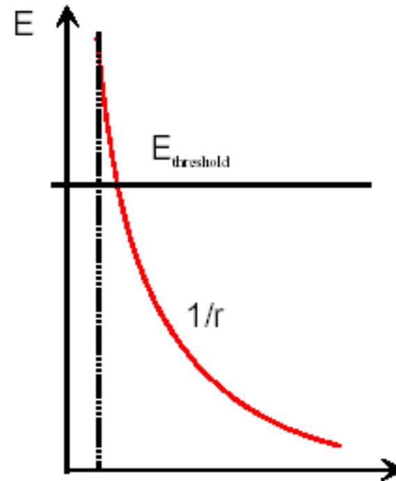
If the energy  $eEd$  gained over several mean free paths ( $d$  around 10mm) exceeds the ionisation energy  $\rightarrow$  new electron
