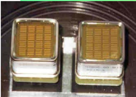
We employed R5900 PMTs with a rather low active area fraction (36% for dense packing) + optical system.
