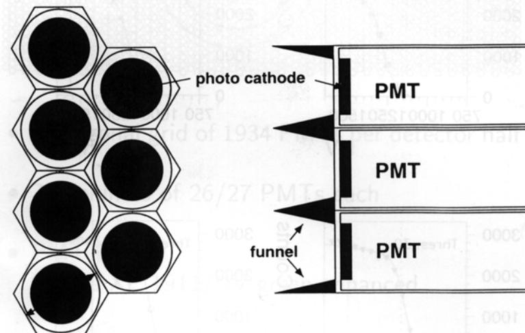
Photocathodes cover only 38% of the focal plane. This is increased to 92% by soft steel funnels with aluminum foil inserts.
