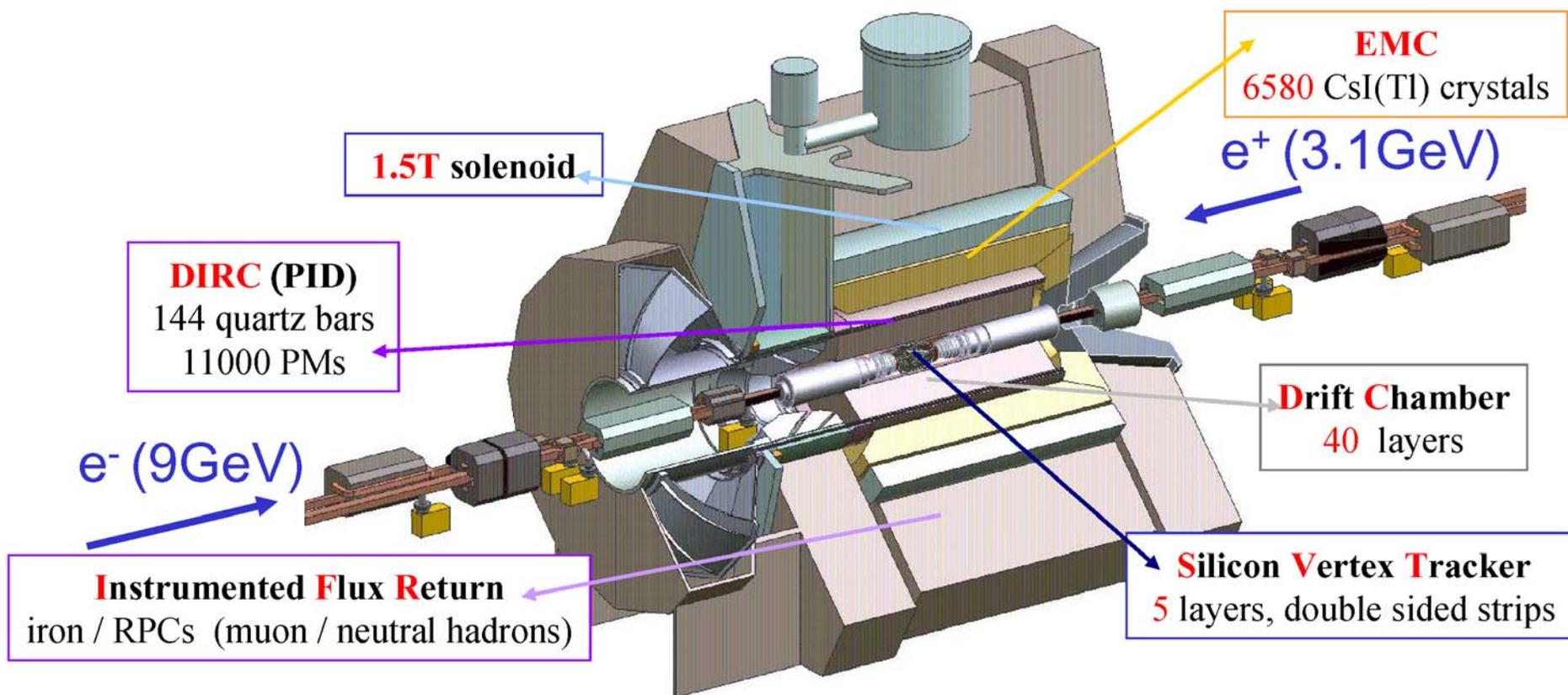
**DIRC - detector of internally reflected Cherenkov light**
