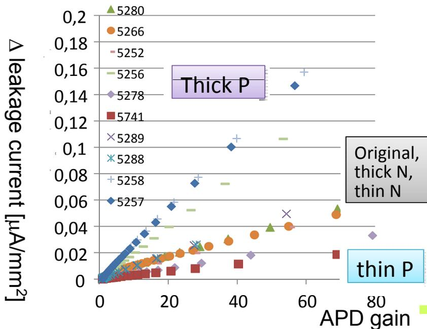
As expected, the increase of the leakage current is smaller with thin p
