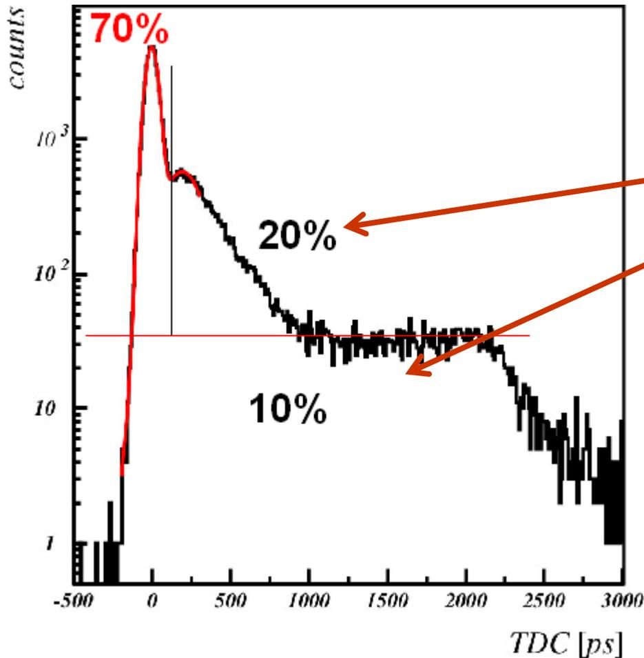
Tails understood (scattering of photoelectrons off the MCP)
