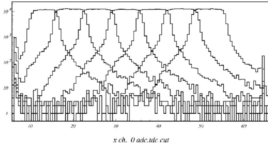
Number of detected hits on individual channels as a function of light spot position.
