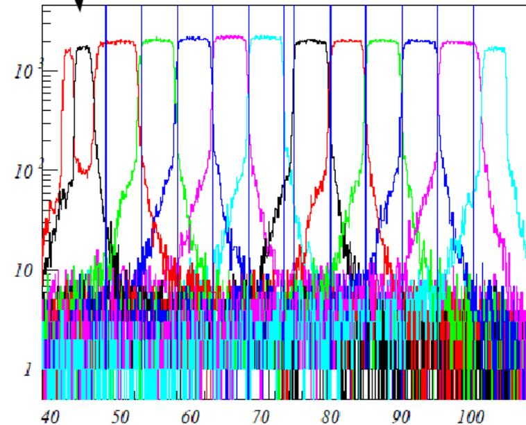
In non-perpendicular mag. field the image shifts and part of the active area is lost!
