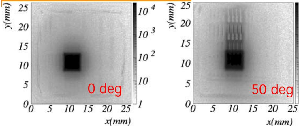
Scans across the PMT. In the 50 deg scan shift of the original image can be observed due to photon reflections and photo-effect at the dynode structure.
