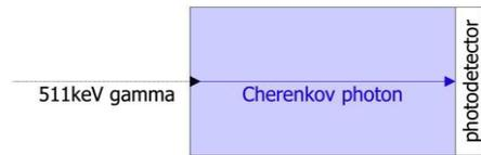
$d = 15 \text{ mm}, n = 1.8: t = d \cdot n / c_0 = 90 \text{ ps}$
