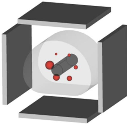
Simulated arrangement of 30x30 cm<sup>2</sup> flat panel detectors
