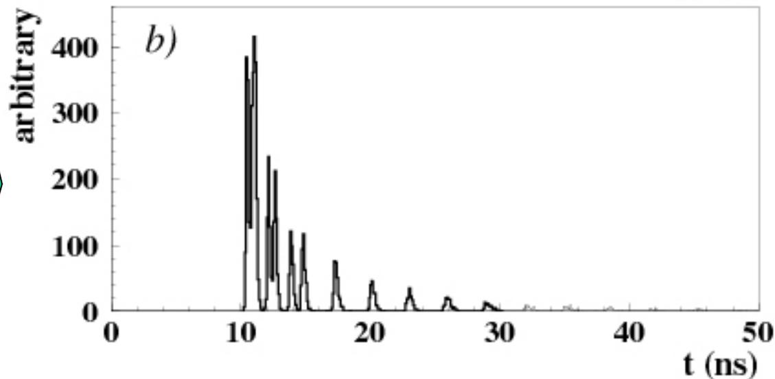
Pattern in the coordinate-time space ('ring') of a pion hitting a quartz bar with  $\sim 80$  MAPMT channels
