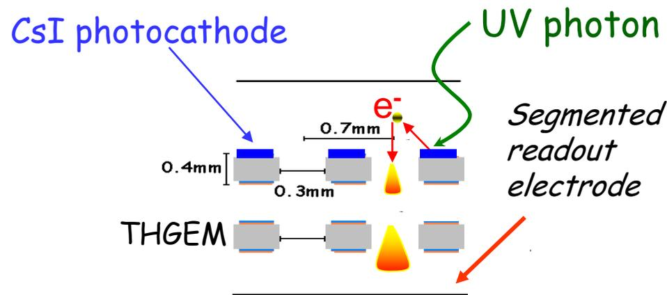
Ion damage of the photocathode: ions can be blocked
