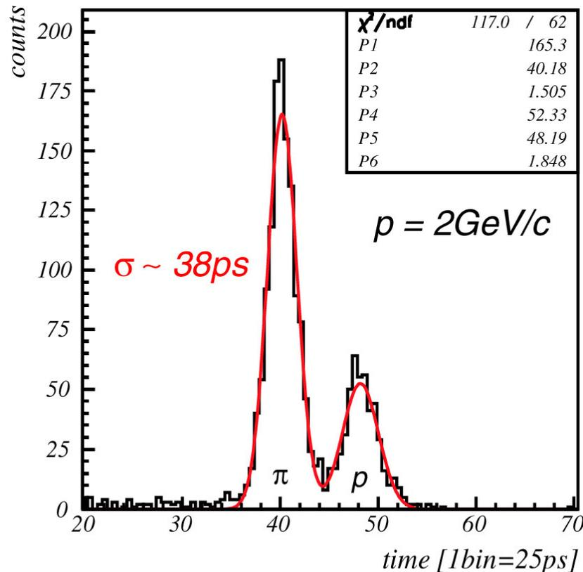
TOF test with pions and protons at 2 GeV/c.
