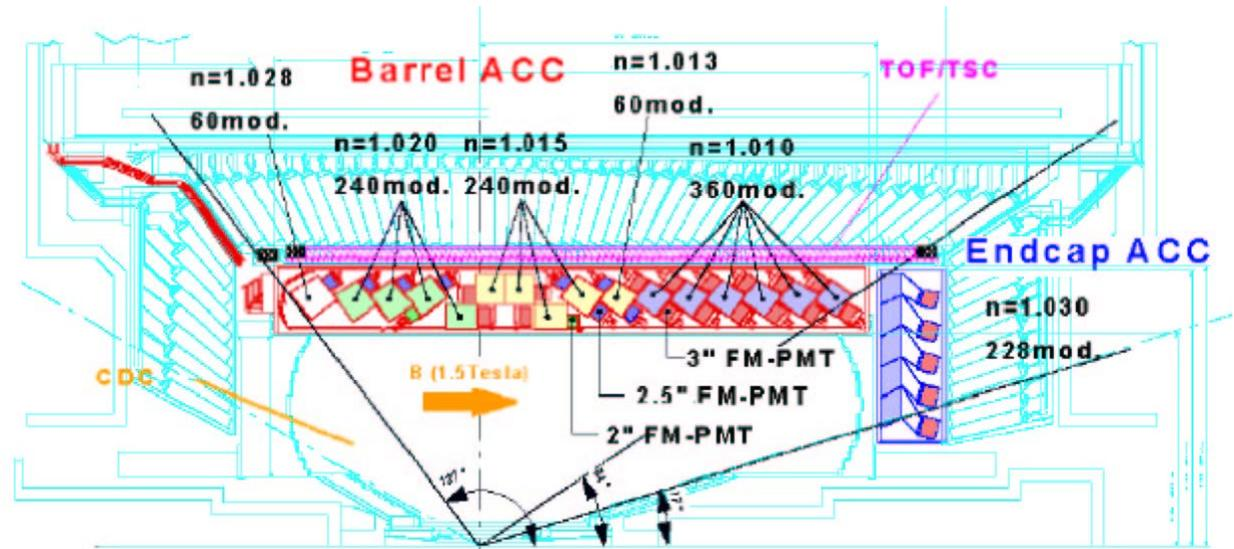
Fine-mesh PMT: works in high B fields
