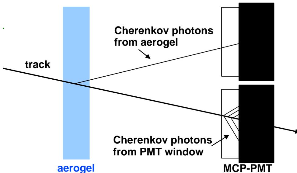
For time of flight: use Cherenkov photons emitted in the **PMT window**
