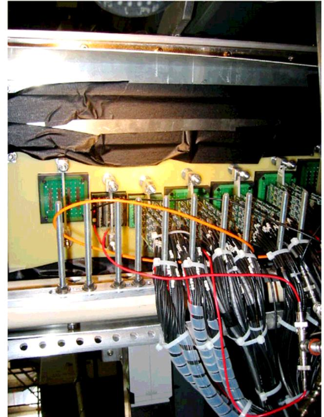
Photon detectors: flat pannel PMTs and Burle MCP PMTs,
