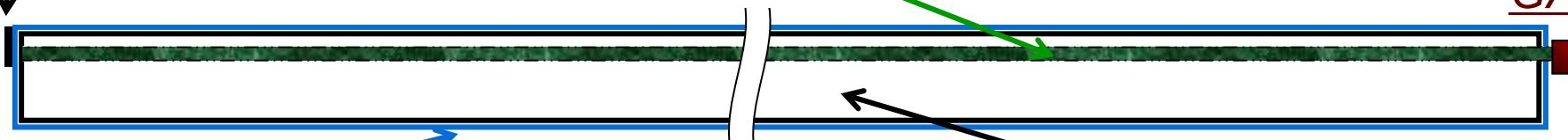
Diffusion reflector ( $\text{TiO}_2$ )    Strips: polystyrene with 1.5% PTP & 0.01% POPOP
