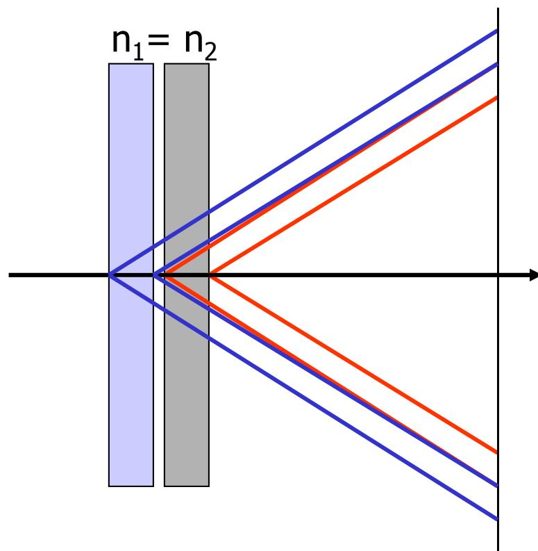
Samo Korpar: → stack two tiles with different refractive indices: “focusing” configuration
