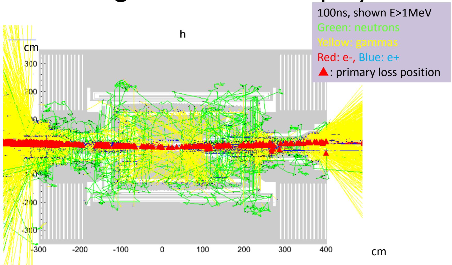
Neutrons: background hits in the muon and KL detection system (KLM) → reduce the efficiency of muon and KL detection → replace RPCs in the endcaps and 2 barrel layers.
