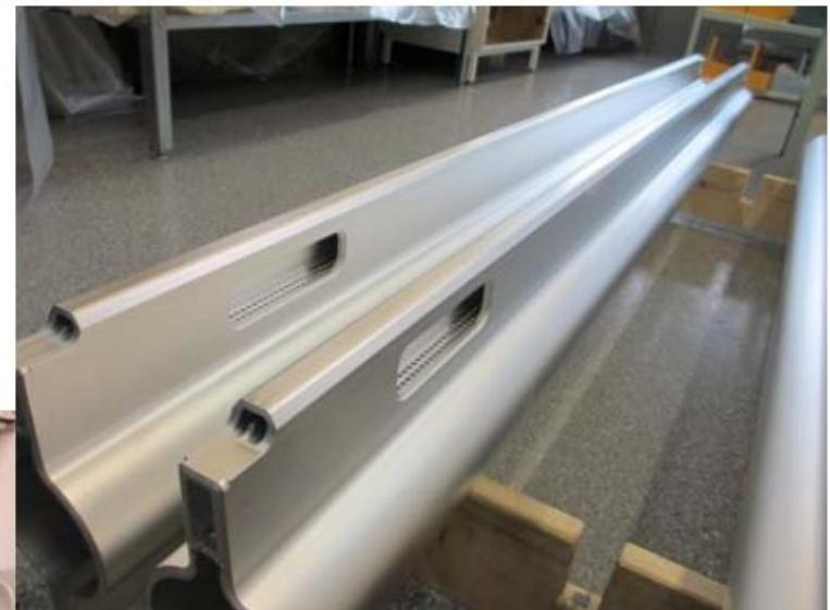
Beam pipe is made of aluminum.
