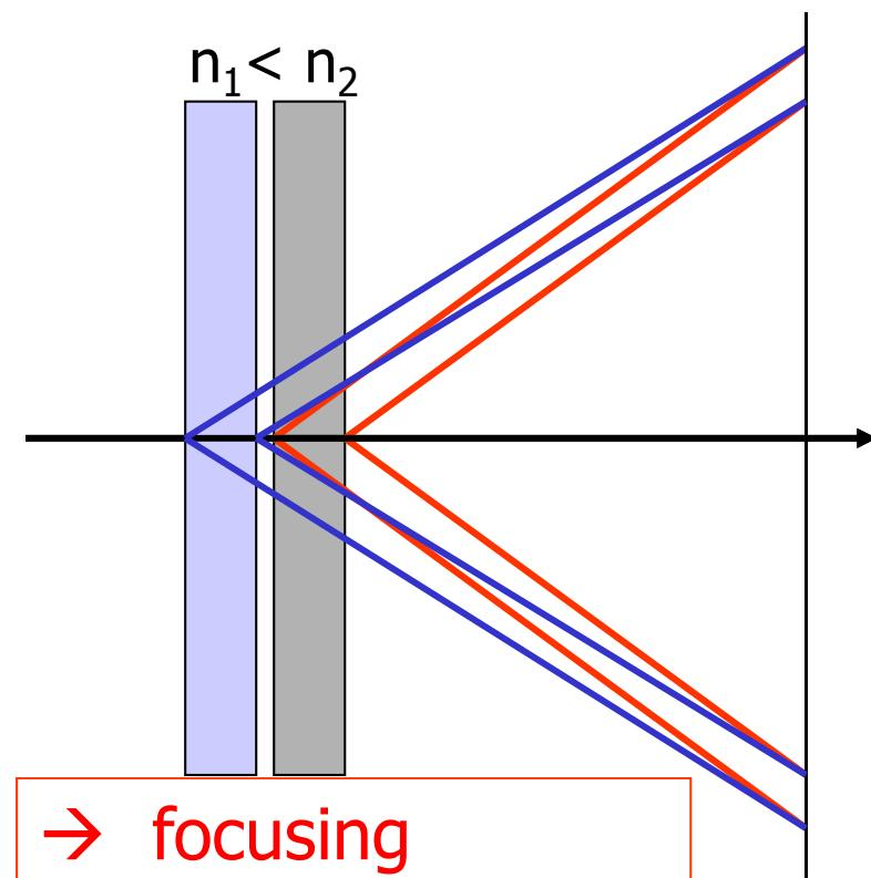
Such a configuration is only possible with aerogel (a form of  $\text{Si}_x\text{O}_y$ )
