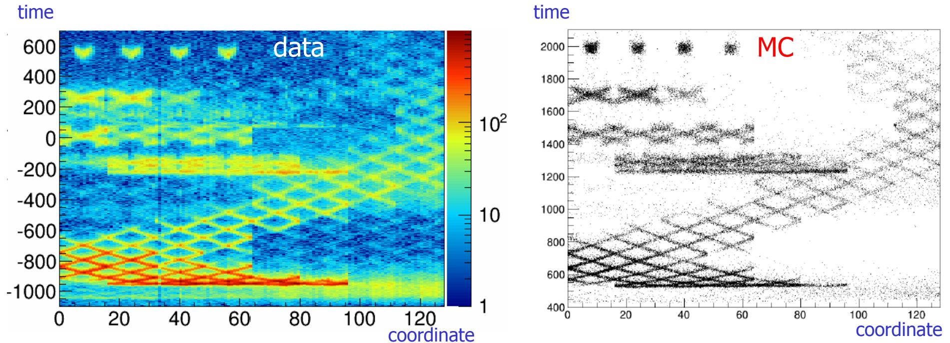
Excellent agreement between beam test data and MC simulated patterns.
