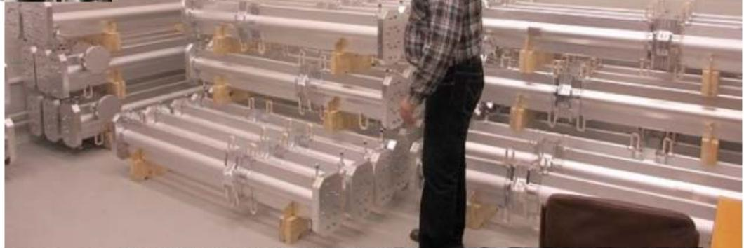
Fabrication of the LER arc beam pipe section is completed
