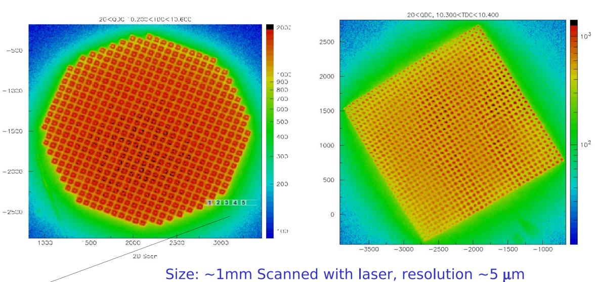
Close-up of the two sensors,  $150\mu m \times 150$  resolution  $\sim 5\mu m$
