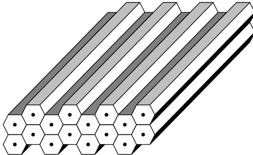
**Figure 2.9:** Schematic view of a honeycomb drift chamber
