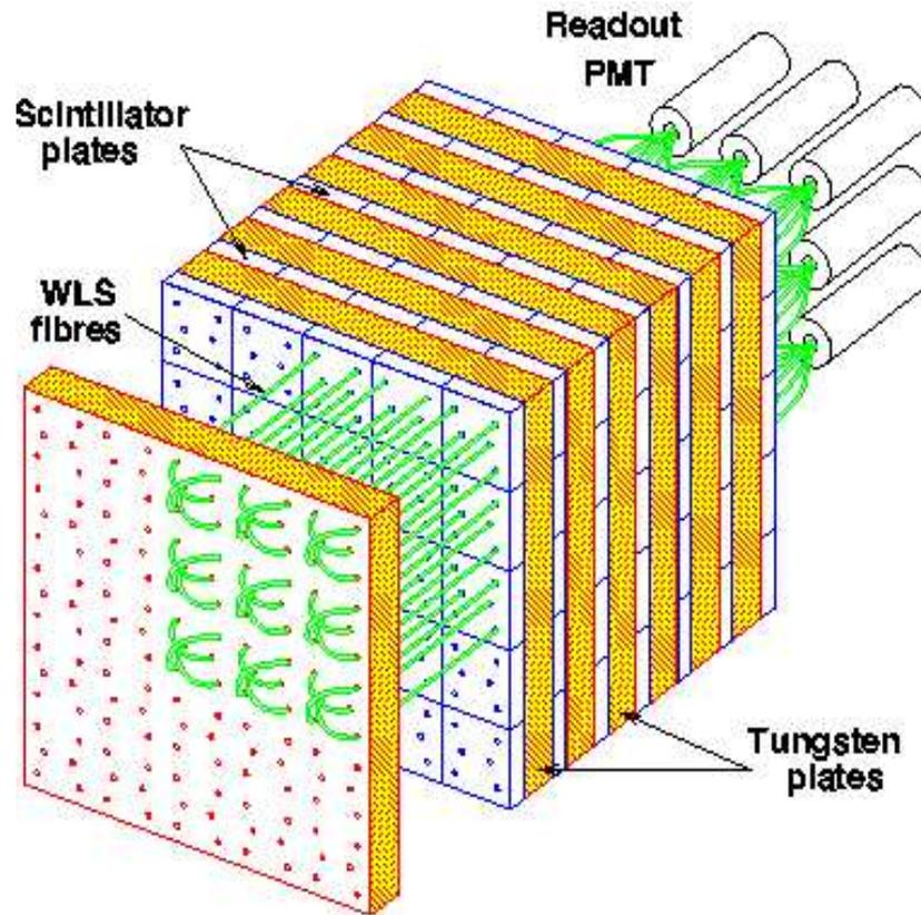
Figure 2.12: Schematic view of one ECAL inner module
