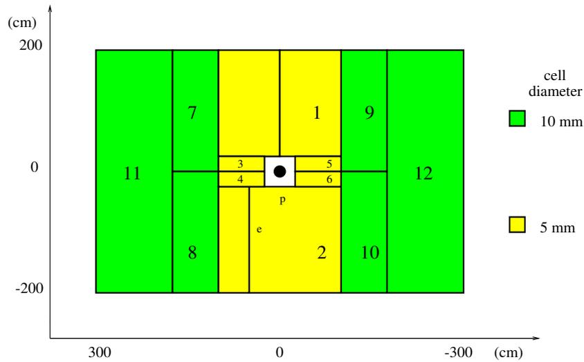
**Figure 2.8:** An OTR superlayer with its twelve subsections.
