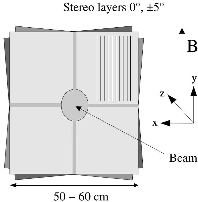
**Figure 2.6:** Geometry of the inner tracker stereo layers
