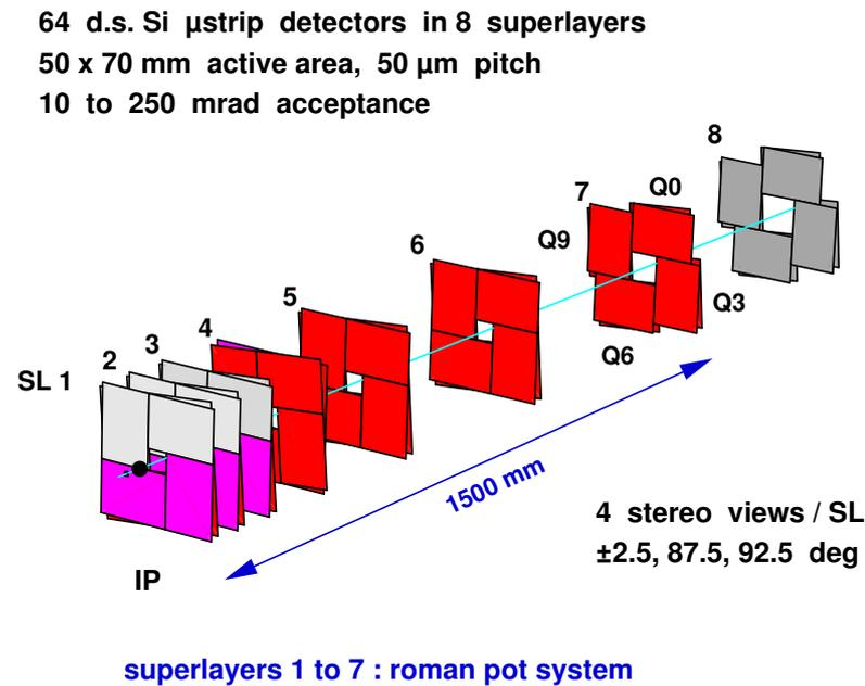
Figure 2.5: Scheme of the detector wafers in the VDS
