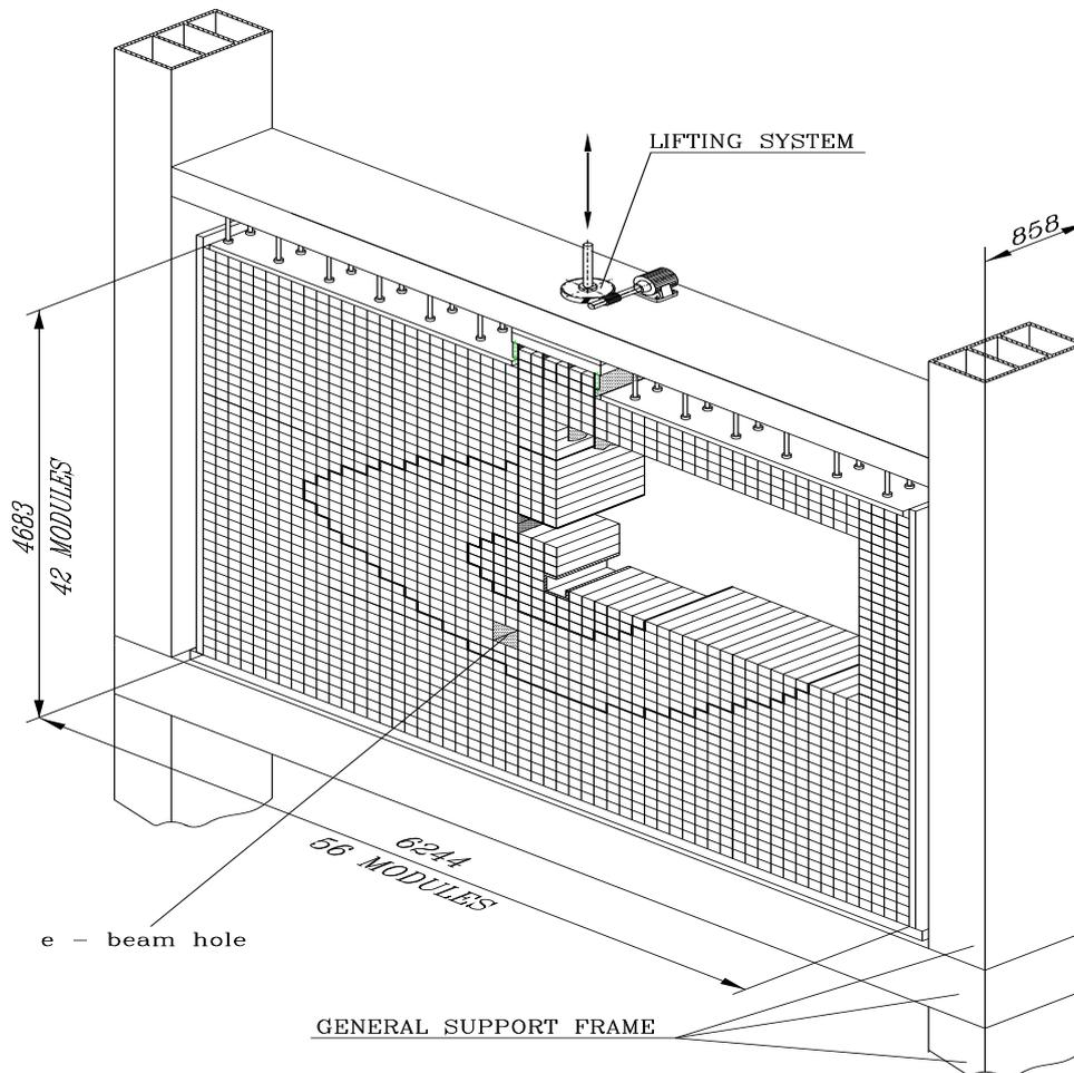
**Figure 2.11:** Schematic view of the ECAL
