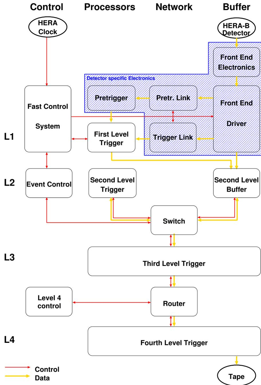
Figure 2.14: Data acquisition scheme and triggering system architecture
