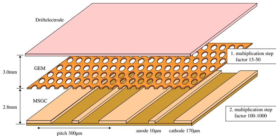
**Figure 2.7:** Schematic view of a microstrip gas chamber
