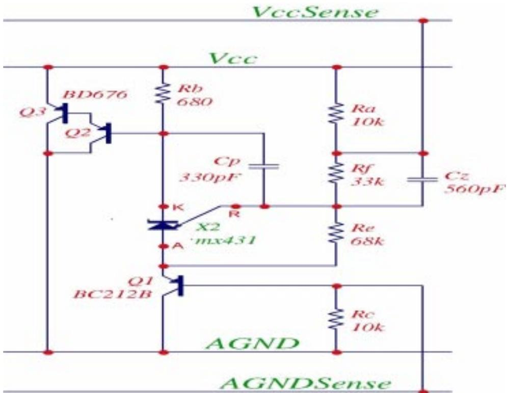
**Fig 1. Schematics of the limiter for Vcc. The circuit for the Vdd is the same but with different values of resistors Rf and Re.**
