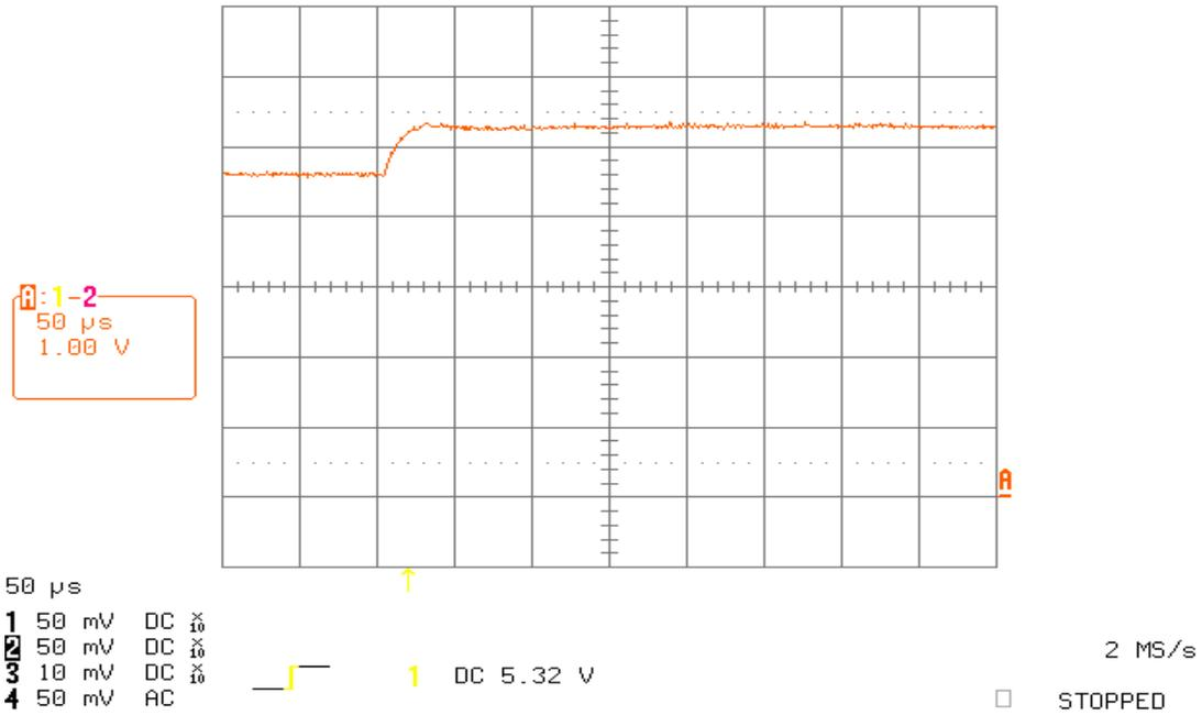
**Fig 7. Vdd vs time after clock off, operating point Vdd = 4.5V**
