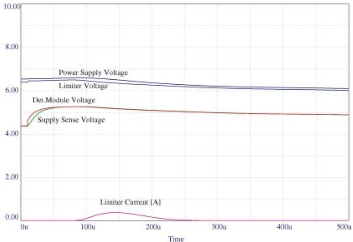
**Fig 9. Simulation of switching the current from 750mA to 375mA with limiter set to  $V_{lim} = 5.1V$ . Det. Module Voltage (red line) is the Vdd on the hybrid (compare with Fig 7)**
