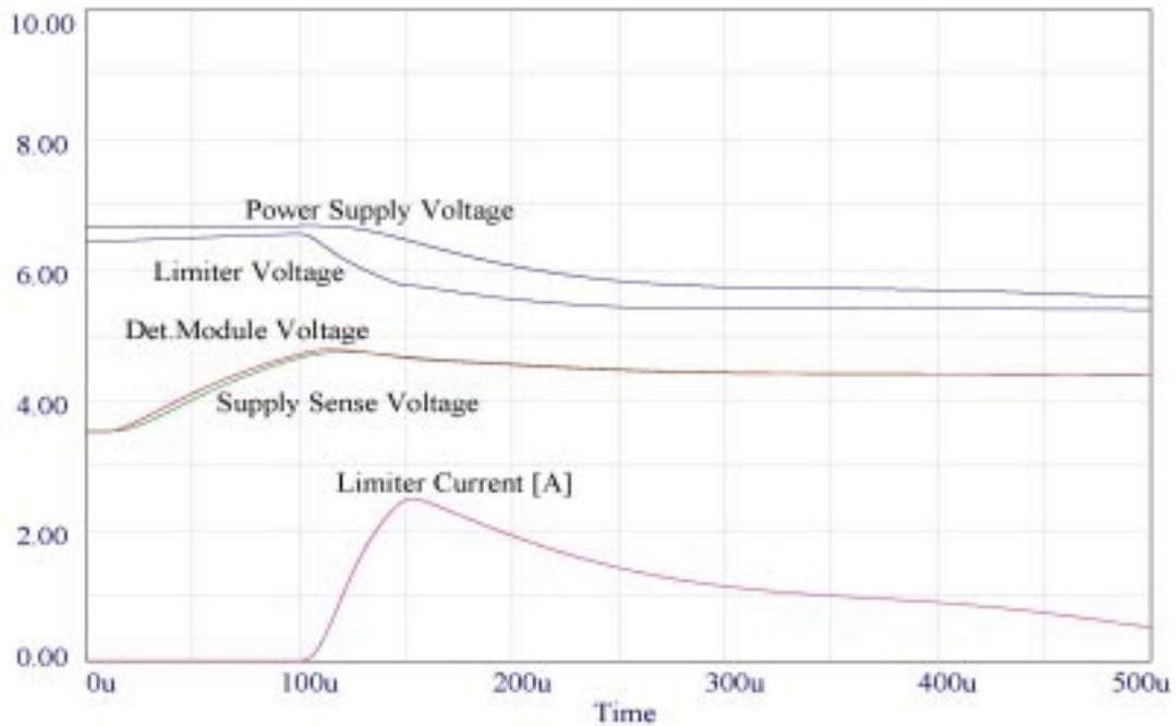
**Fig 4. Simulation of voltages and currents when  $I_{cc}$  is switched from 820mA to 230mA with time constant as measured. Det. Module Voltage (red line) is  $V_{cc}$  on the hybrid and should be compared with measurement.**
