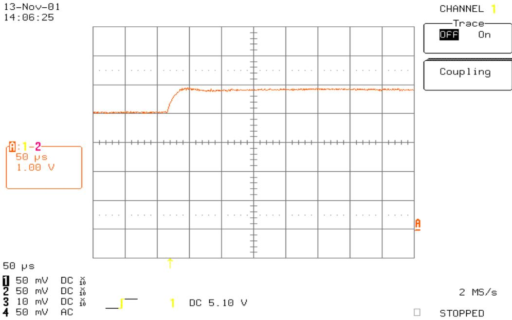
**Fig 5. Vdd vs time after clock off, operating point Vdd = 4V**
