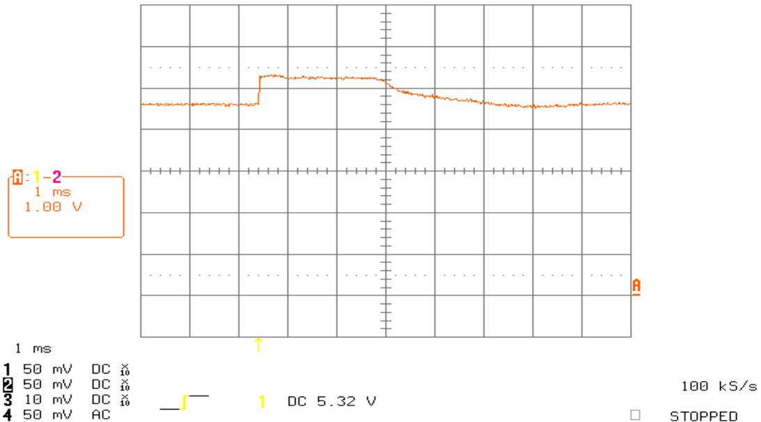
**Fig 8. Vdd vs time after clock off, operating point Vdd = 4.5V, longer time scale**
