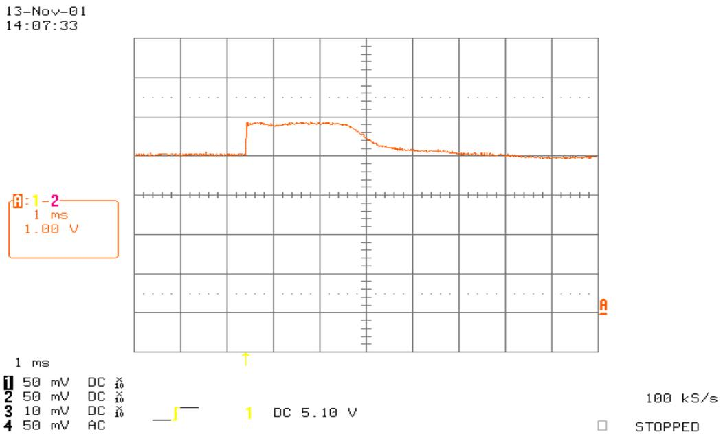
**Fig 6. Vdd vs time after clock off, operating point Vdd = 4V, longer time scale.**
