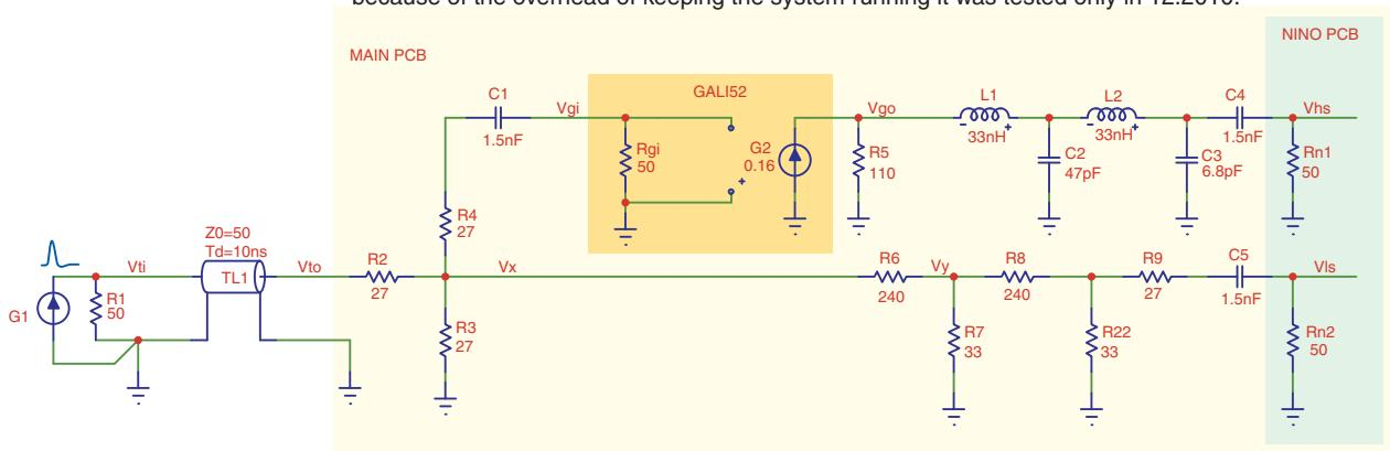
Difference: The attenuation from the GALI output has been moved to the input, and another resistive divider has been added to the low-sensitivity attenuation.
