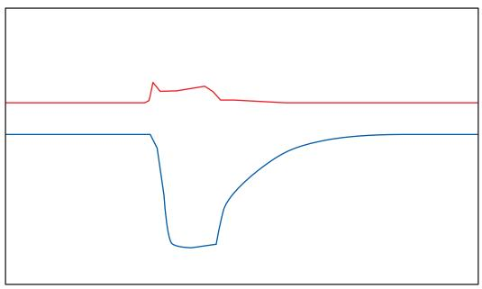
When the input polarity is reversed, the output lines exchange shape, the red becomes the blue and vice versa, but always the line going up is much lower than the line going down, and the line going down has always are latively long tail.
