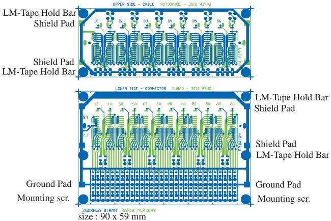
Note: Due to filtering capacitors \* jumpers requirement, the board size was increased (PP1N from 25 to 36 mm and PP1W from 54 to 59 mm). Free Hold Bar screw holes can be used for additional Mounting screws.
