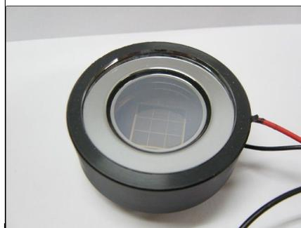
Fig. \* Multi-photon spectrum obtained by the 3x3 multi-channel HAPD and a photo of the HAPD.
